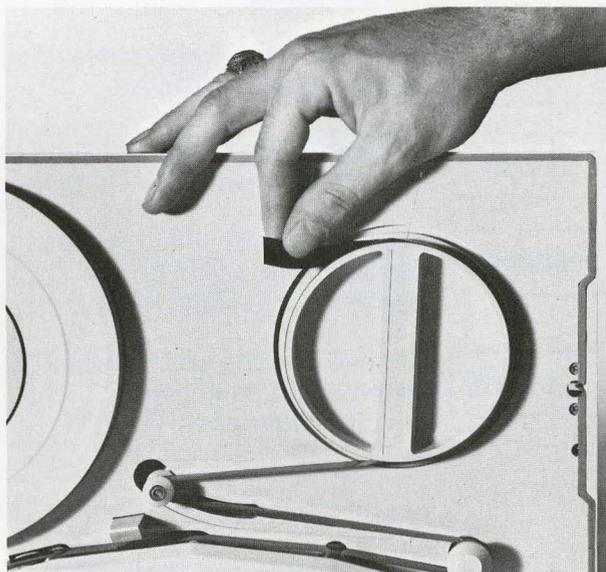
All Pertec 7000-Series transports have a unique tape loading feature. Since these models will often be used by unskilled operators, Pertec has devised a unique design which eliminates the take-up reel, making tape loading and tape handling extremely fast and simple.
