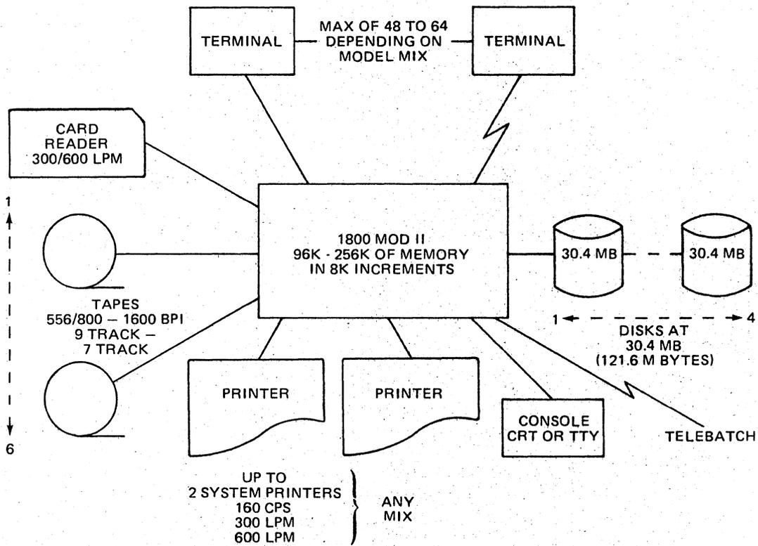
Figure 1. PCC 1800 MOD II System Block Diagram
