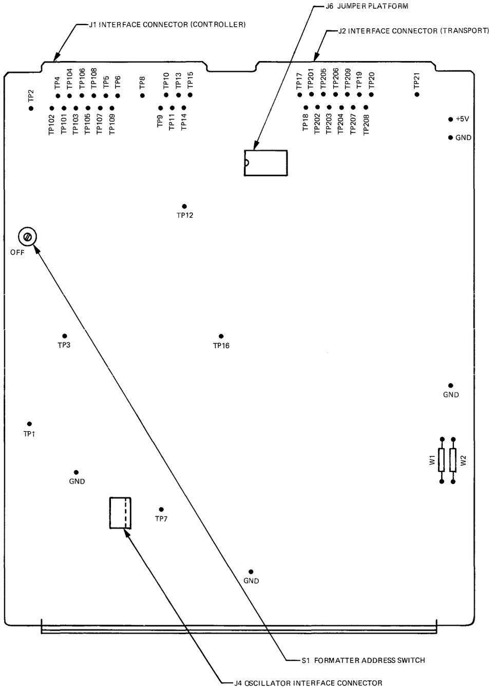
Figure 5-8. PE Write/Control PCBA, Test Point and Connector Placement
