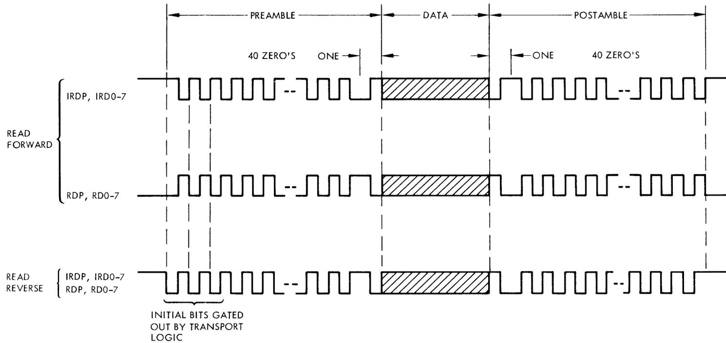
Figure 5-17. Read Input Signals
