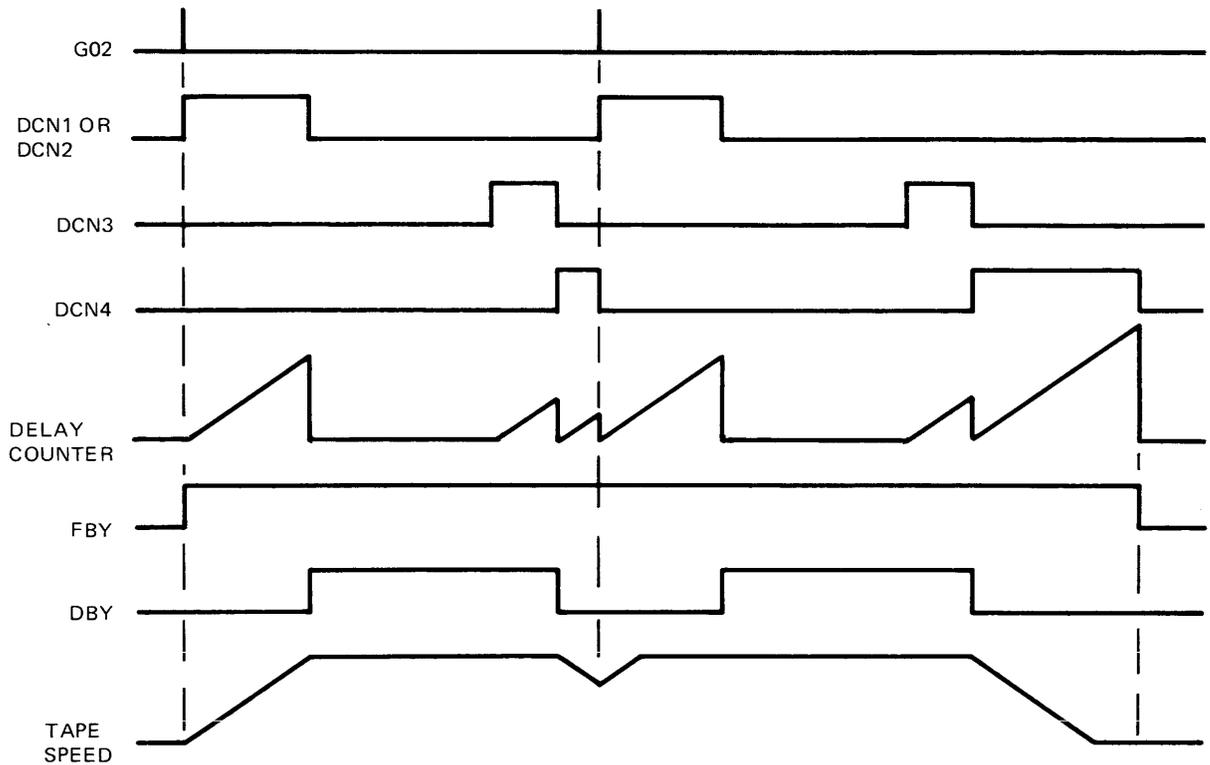
Figure 5-12. On-the-Fly Operation
