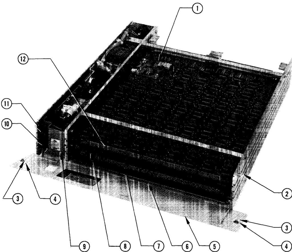
Figure 7-1. Phase Encoded Formatter Photo Parts Index
