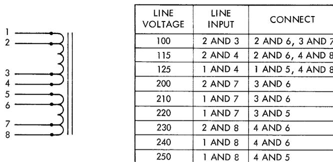
Figure 2-1. Transformer Primary Connections
