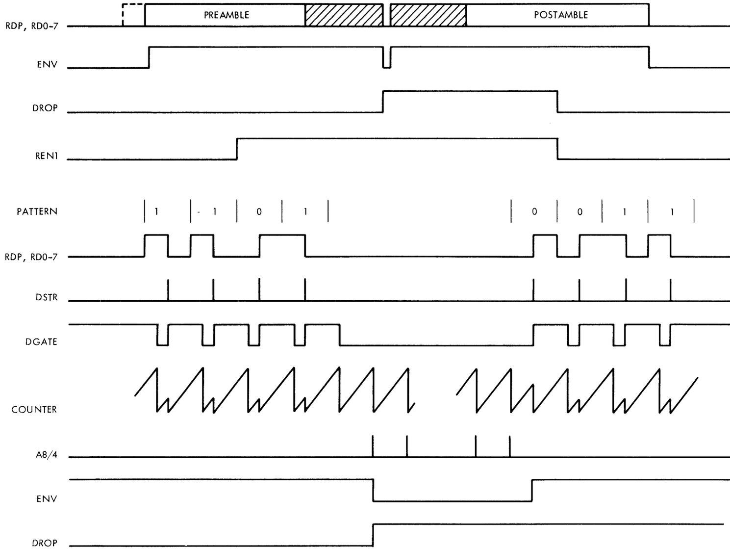
Figure 5-19. Envelope and Drop Waveforms
