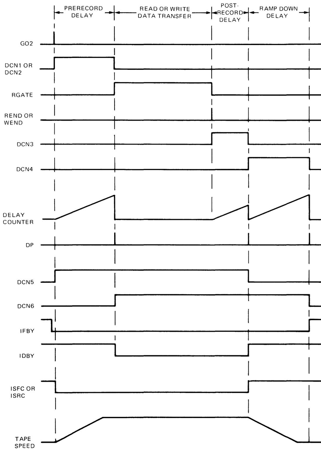
Figure 5-11. Command Timing
