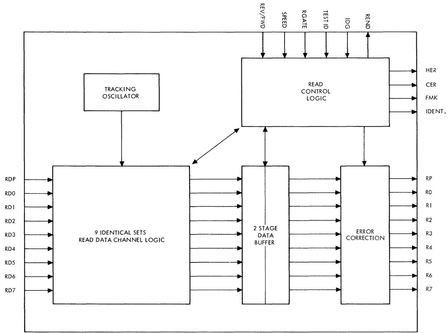
Figure 4-6. Read Recovery PCBA, Simplified Block Diagram
