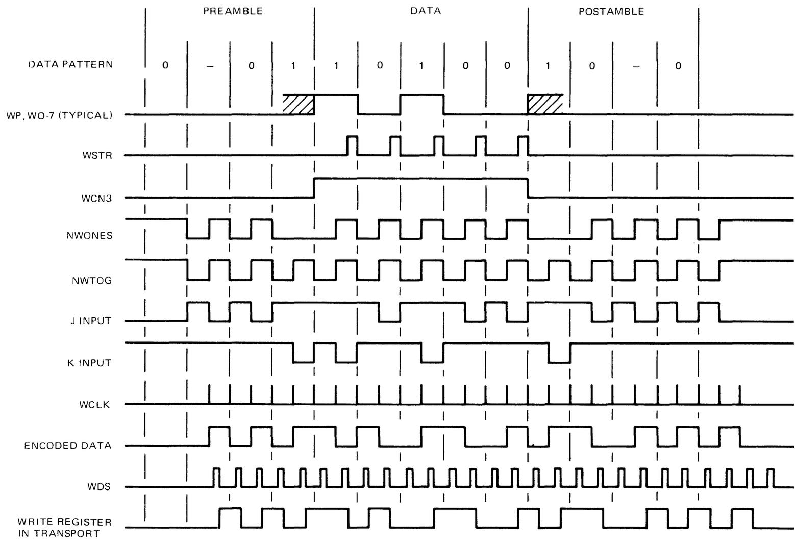
Figure 5-15. Write Data Encoding
