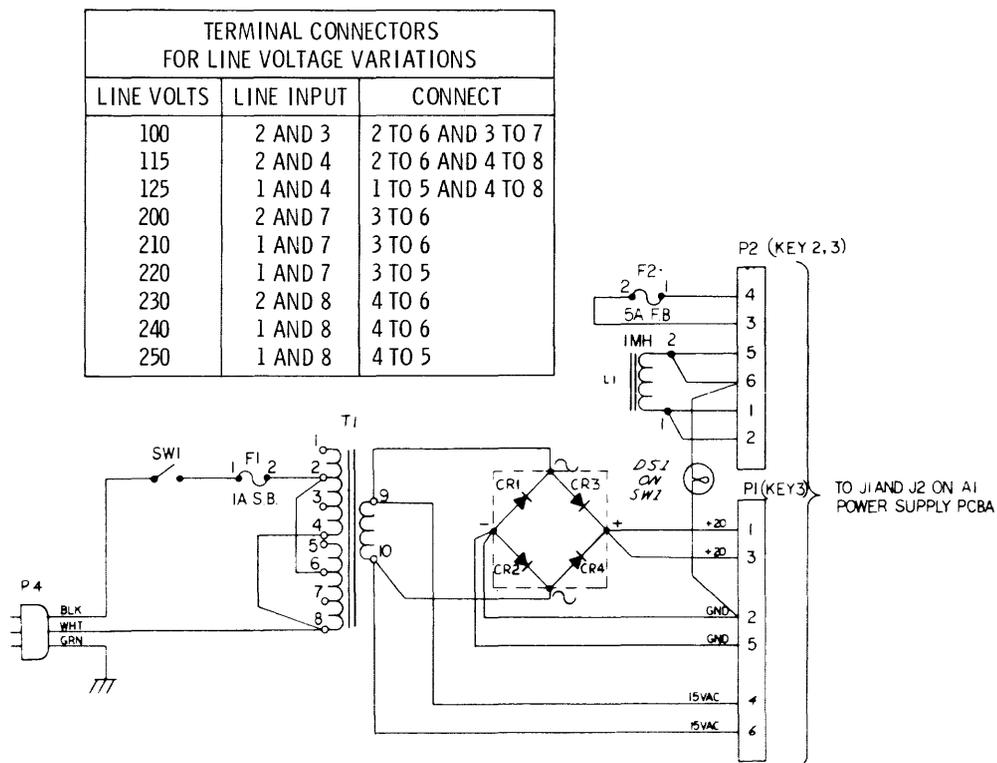
Figure 5-3. Chassis Mounted Power Supply Components
