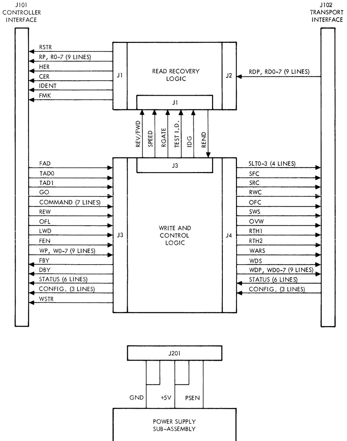
Figure 4-3. Phase Encoded Formatter Organization
