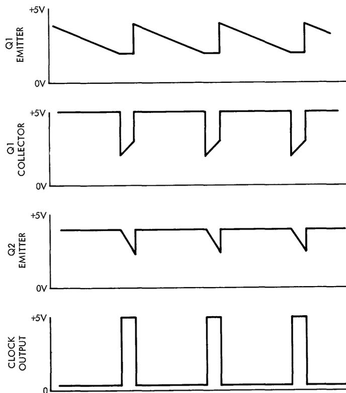
Figure 5-5. Fixed Oscillator Waveforms
