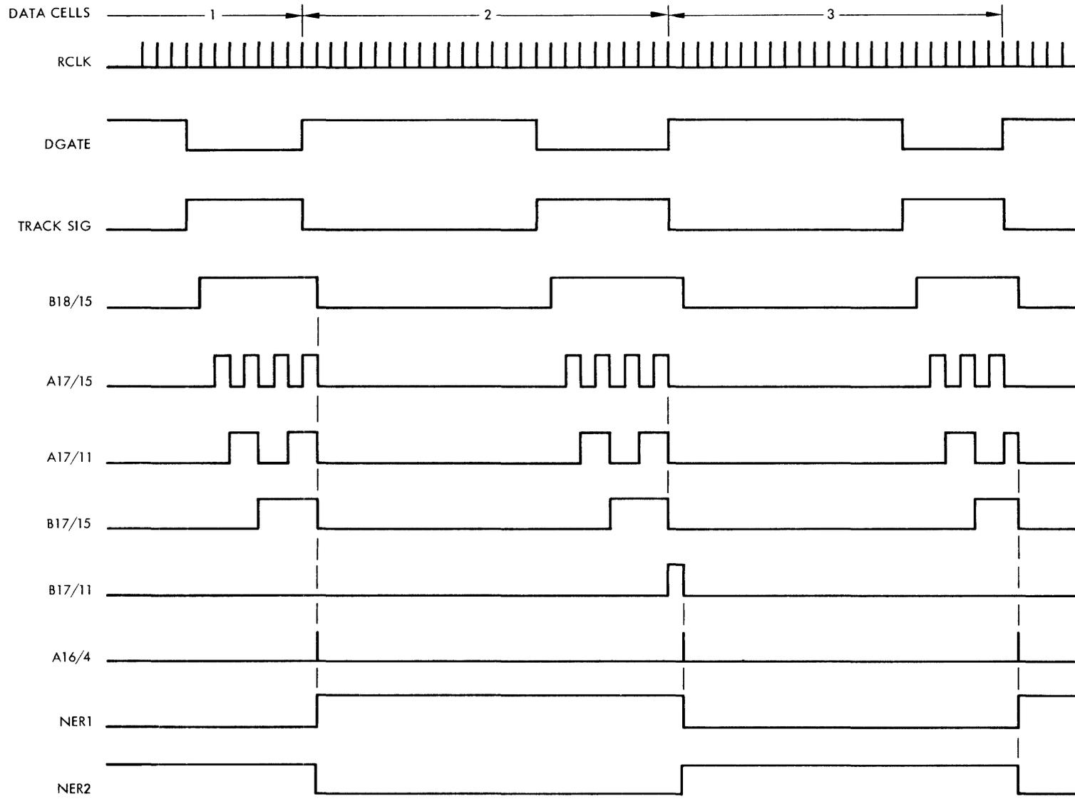
Figure 5-21. Tracking Control Waveforms
