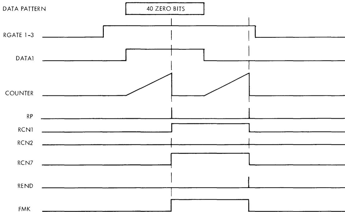
Figure 5-25. File Mark Waveforms
