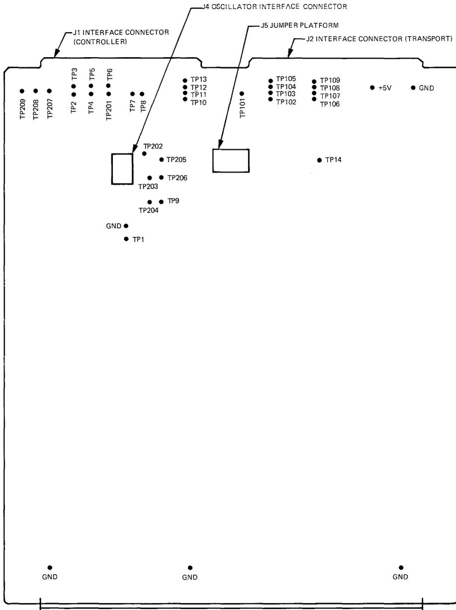
Figure 5-16. PE Read Recovery PCBA, Test Point and Connector Placement
