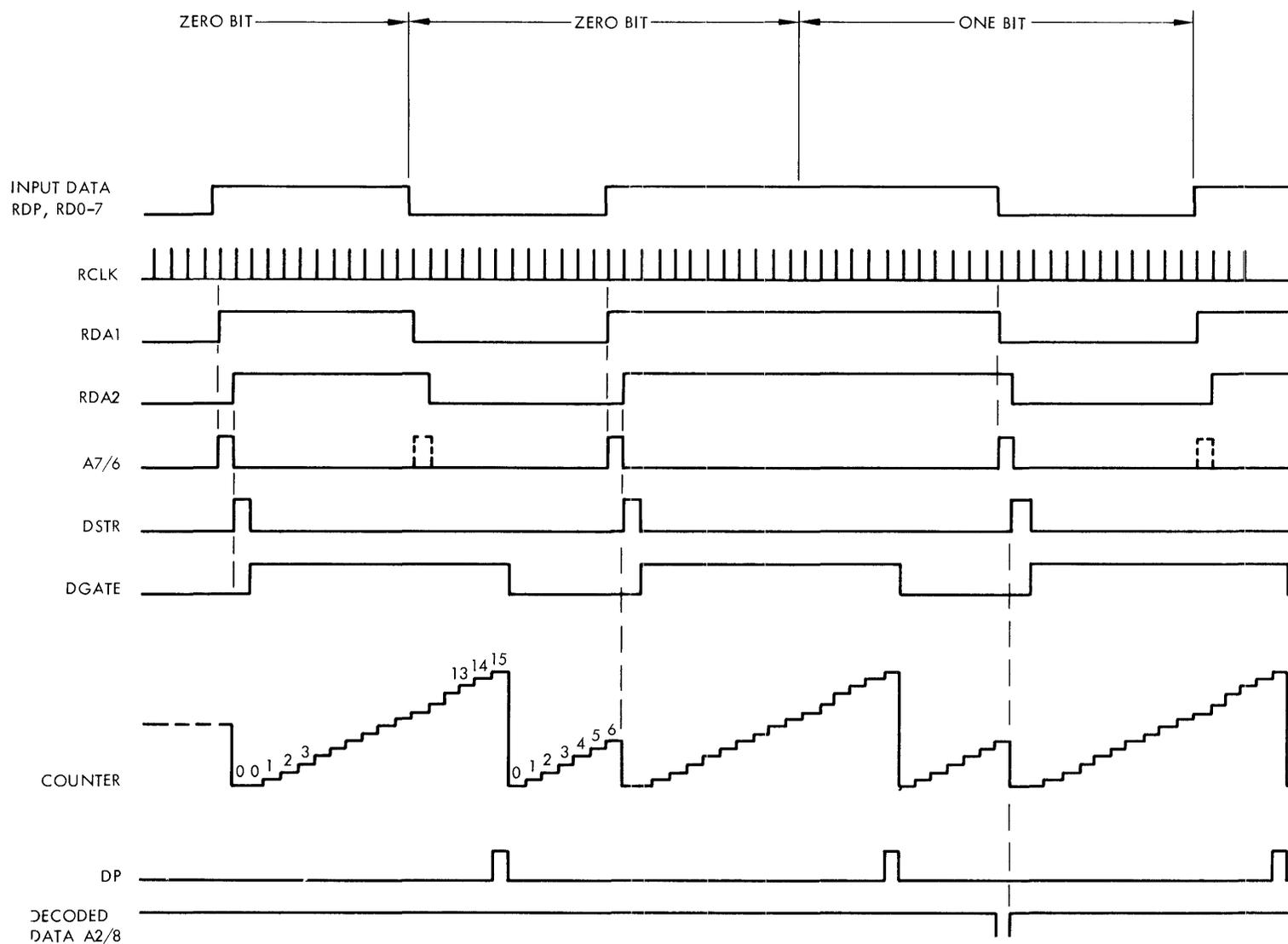
Figure 5-18. Data Decoding Waveforms
