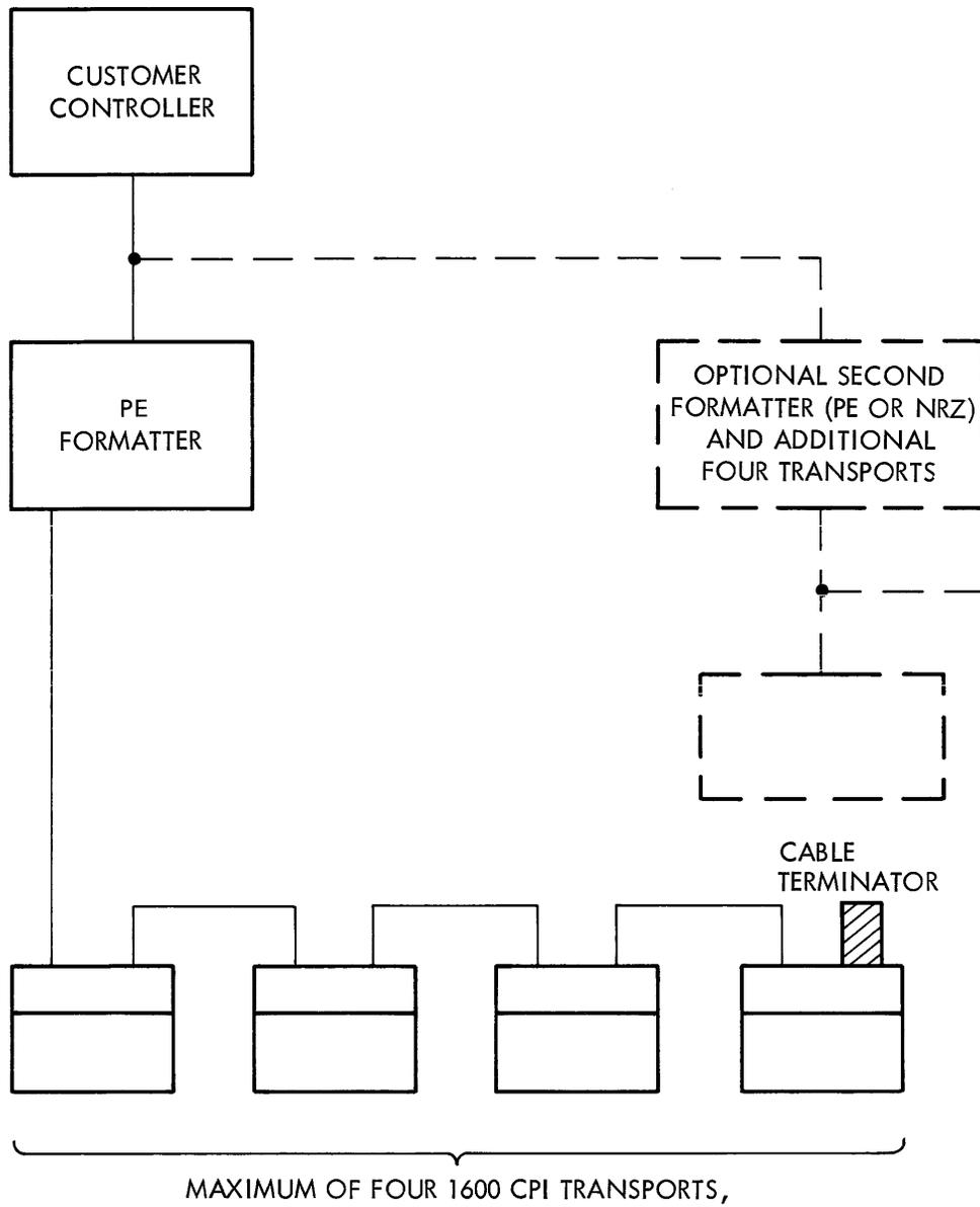
Figure 1-2. PE Formatter System Configuration
