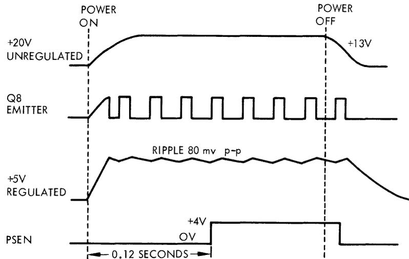
Figure 5-4. Switching Regulator Waveforms
