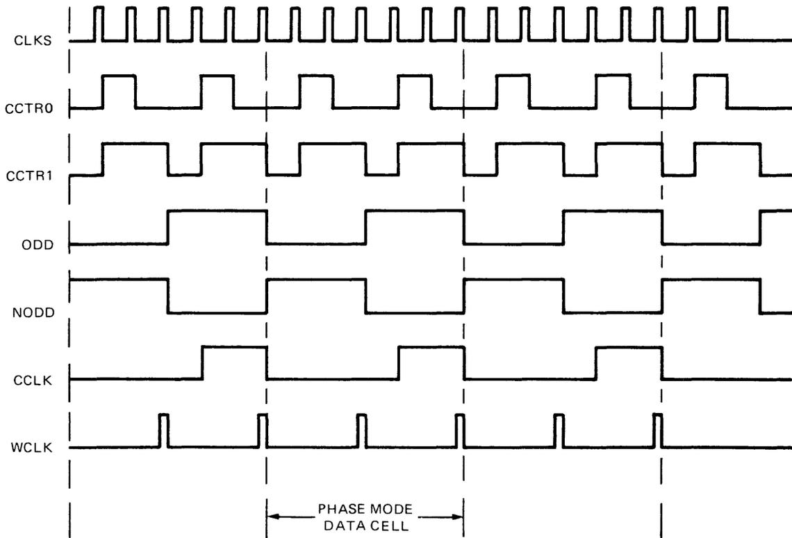
Figure 5-9. Clock Waveforms
