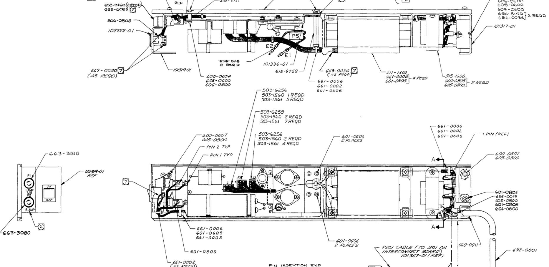
9. SECURE WIRES WITH CABLE CLAMPS PRIOR TO SOLDERING TO TERMINALS.
