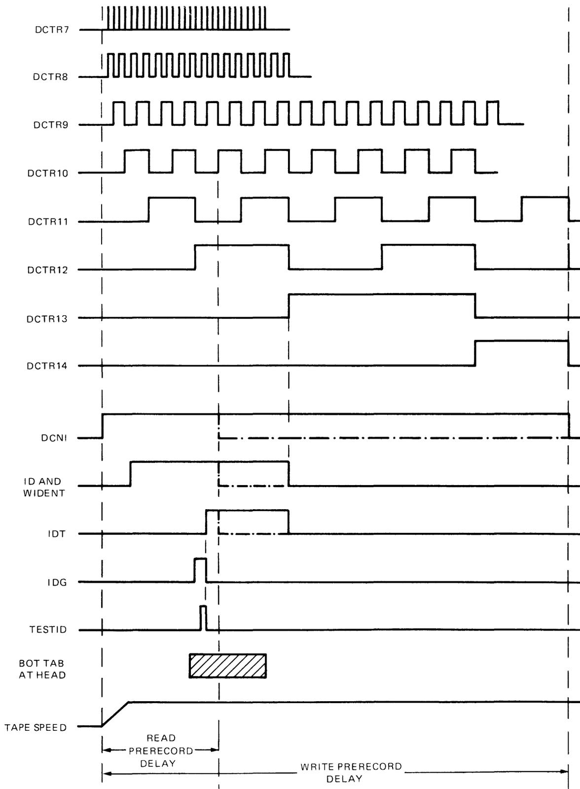
Figure 5-13. Identification Timing, Read and Write
