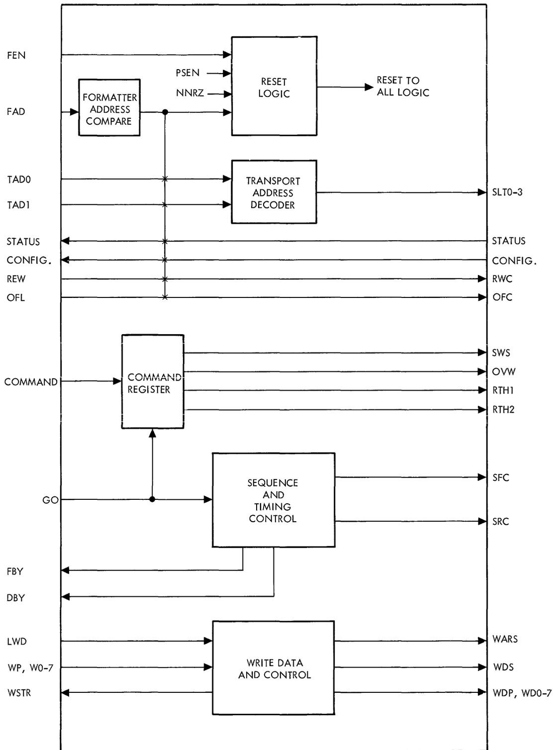
Figure 4-4. Write/Control Logic, Simplified Block Diagram
