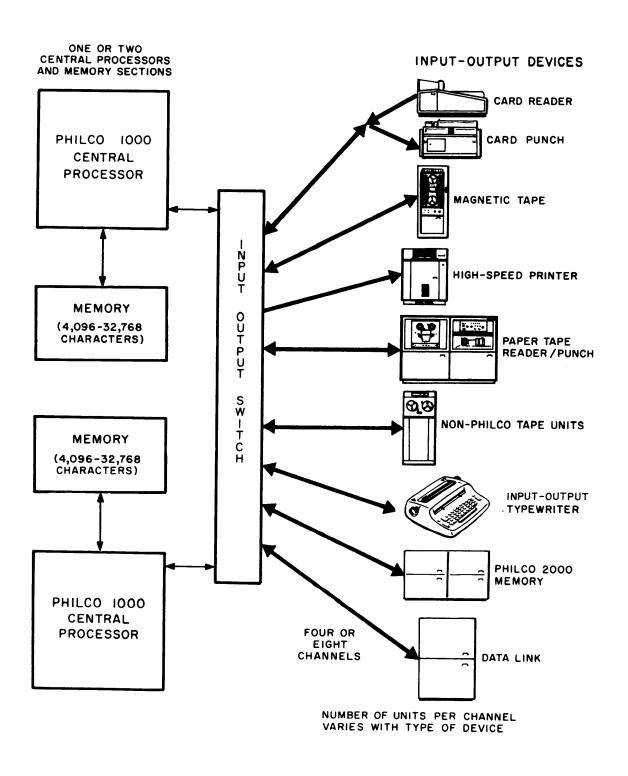
Figure 1. Philco 1000 System Configuration
