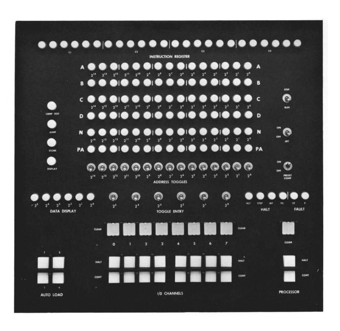
Figure 4. Philco 1000 Operator's Console
