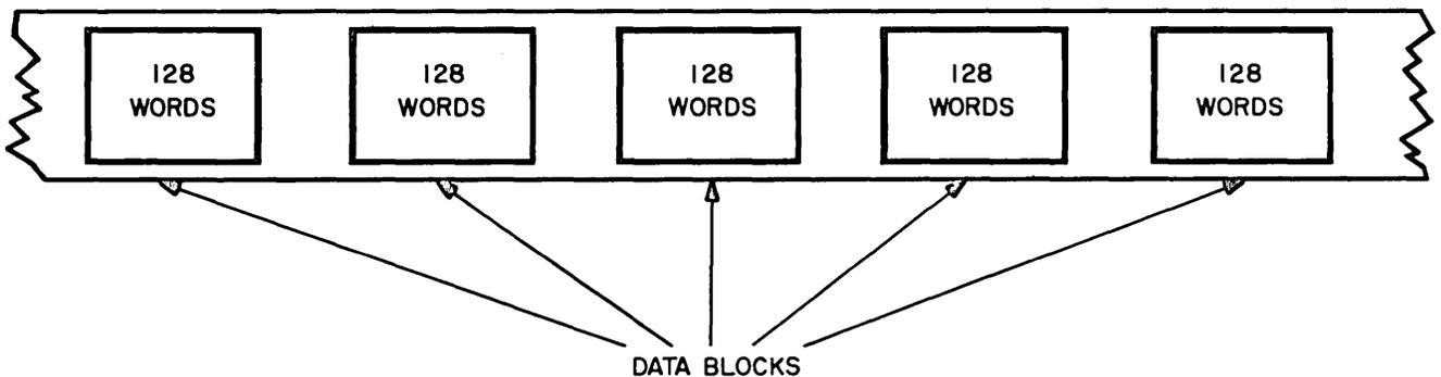
Figure MT-1. Arrangement of Data on Magnetic Tape
