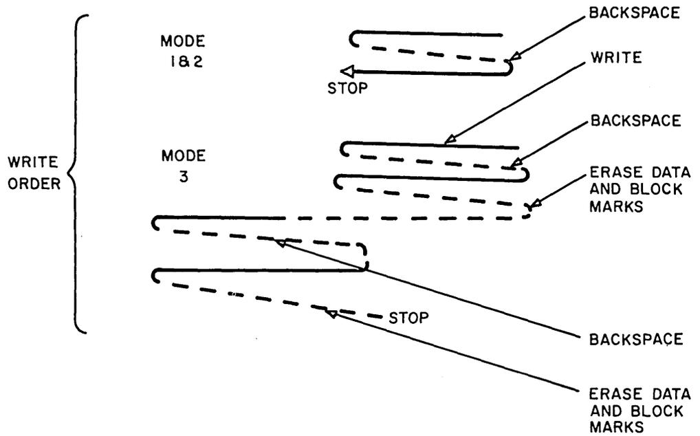
Figure IOP-10. Action of IOP Following Magnetic Tape Parity or Sprocket Errors
