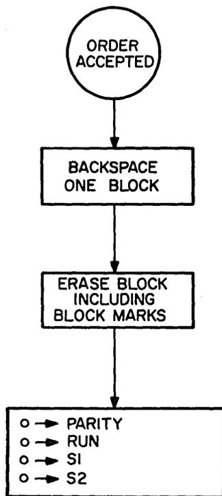
Figure TAC-8. Flowchart of Magnetic Tape Erase Order
