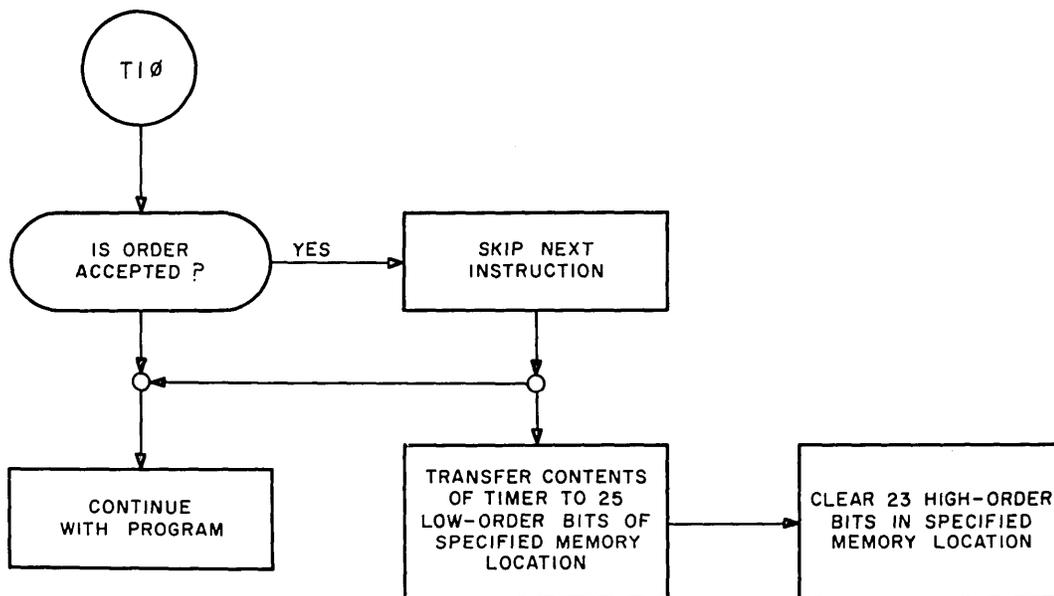
Figure RT-6. Flowchart of Input Order for Interval Timer Unit
