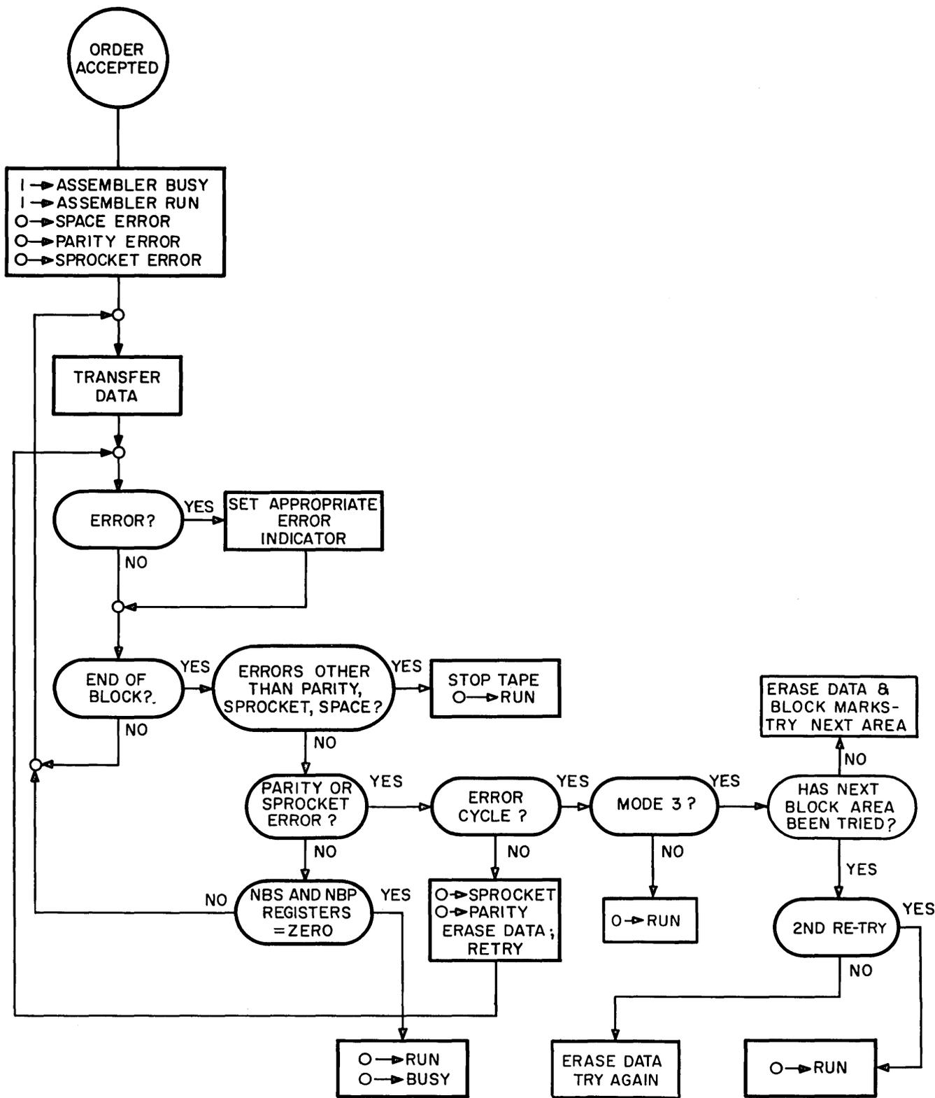
Figure TAC-4. Flowchart of Magnetic Tape Write Order
