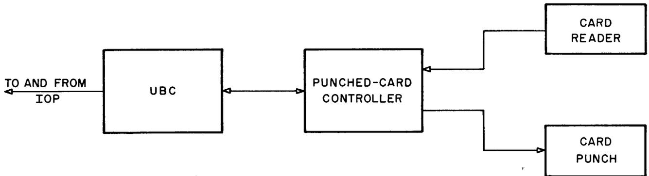
Figure PC-1. Tie-In of Punched-Card System with 2000 System
