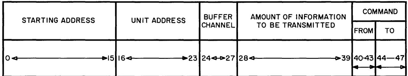
Figure INT-2. Breakdown of D Register Showing Parameters of I-O Order
