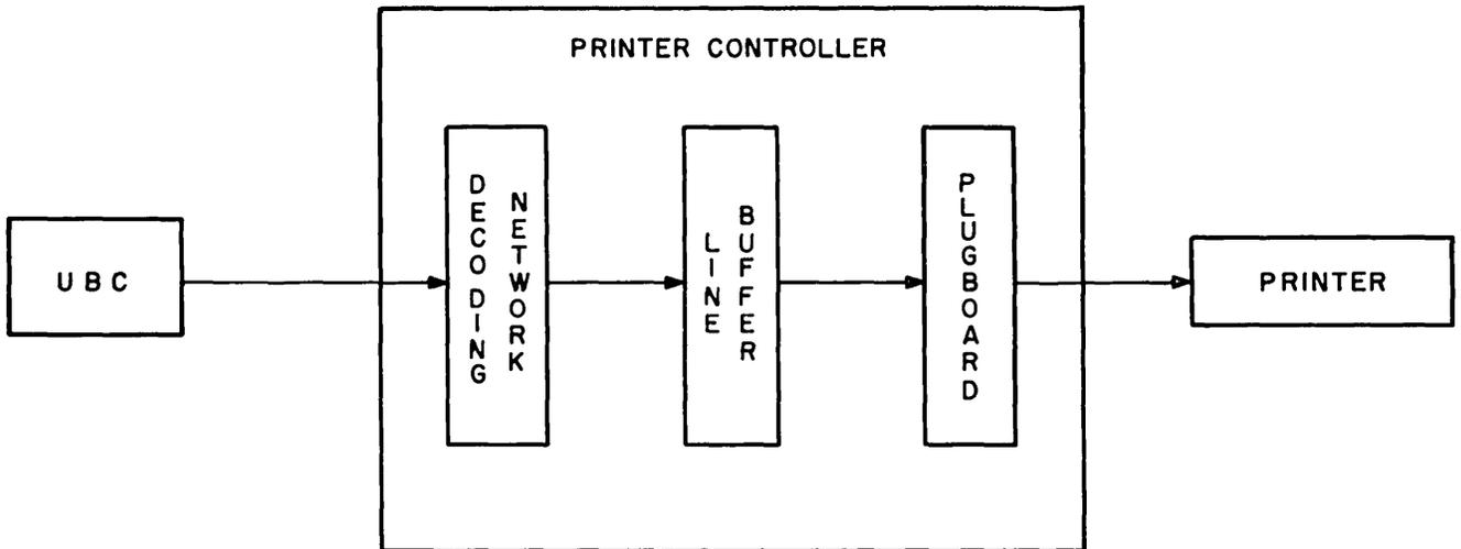
Figure PR-4. Data Flow during a Printing Operation
