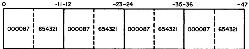
Figure PT-11. Format of One Word in Memory Following a Reading Operation of Eight-Level Tape
