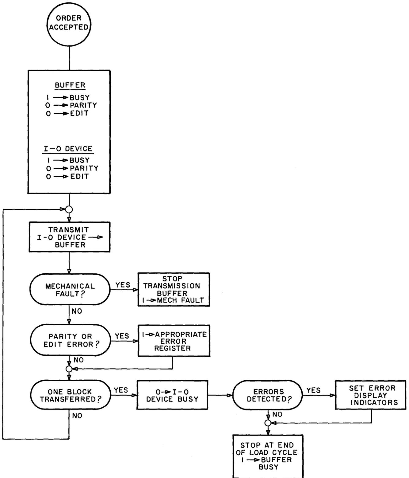
Figure TAC-11. Flowchart of I-O Order, I-O Device to Buffer
