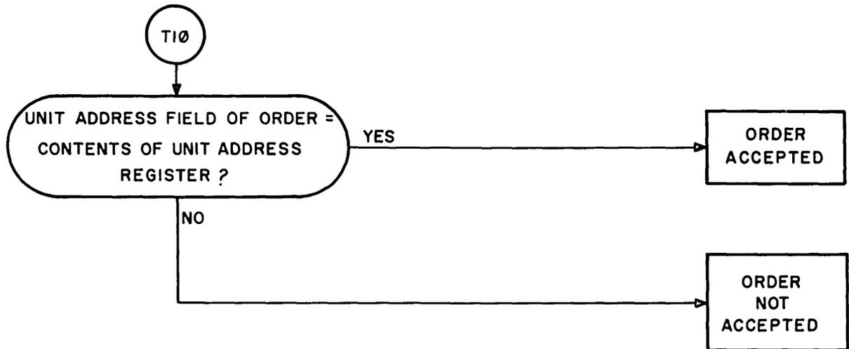
Figure IOP-7. Flowchart of Class B Magnetic Tape Order Acceptance
