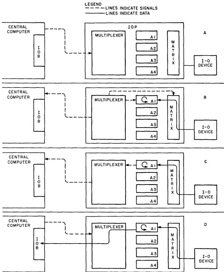
Figure IOP-2. Operation of the IOP During Input Order
