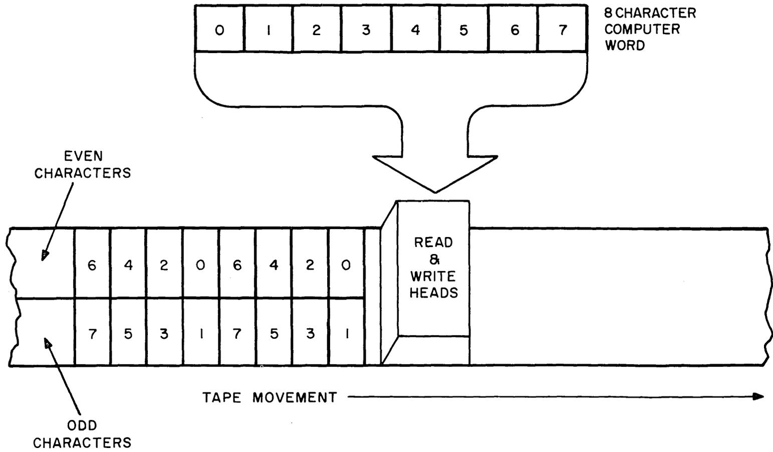
Figure MT-3. Arrangement of Characters on Tape
