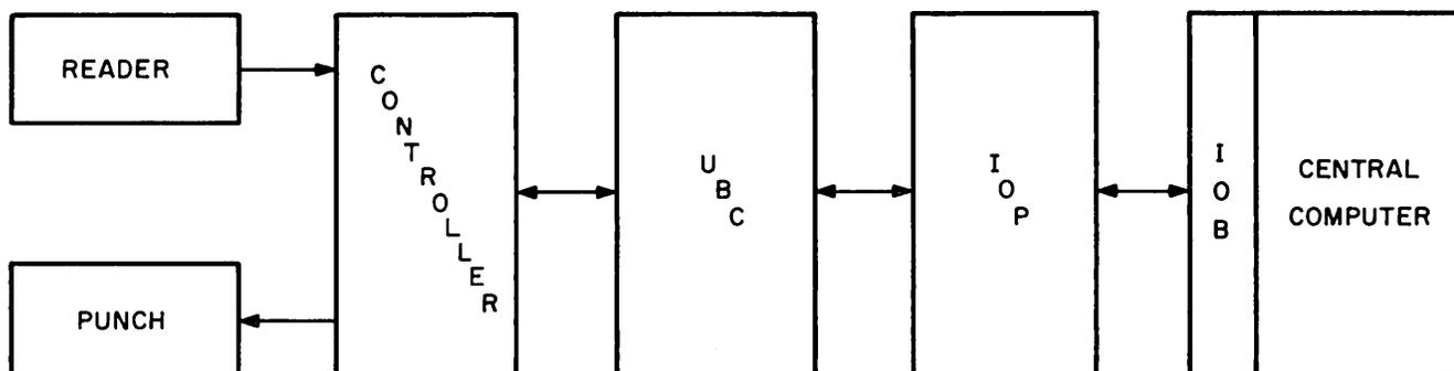
Figure PT-9. Paper Tape System, Model 241,
