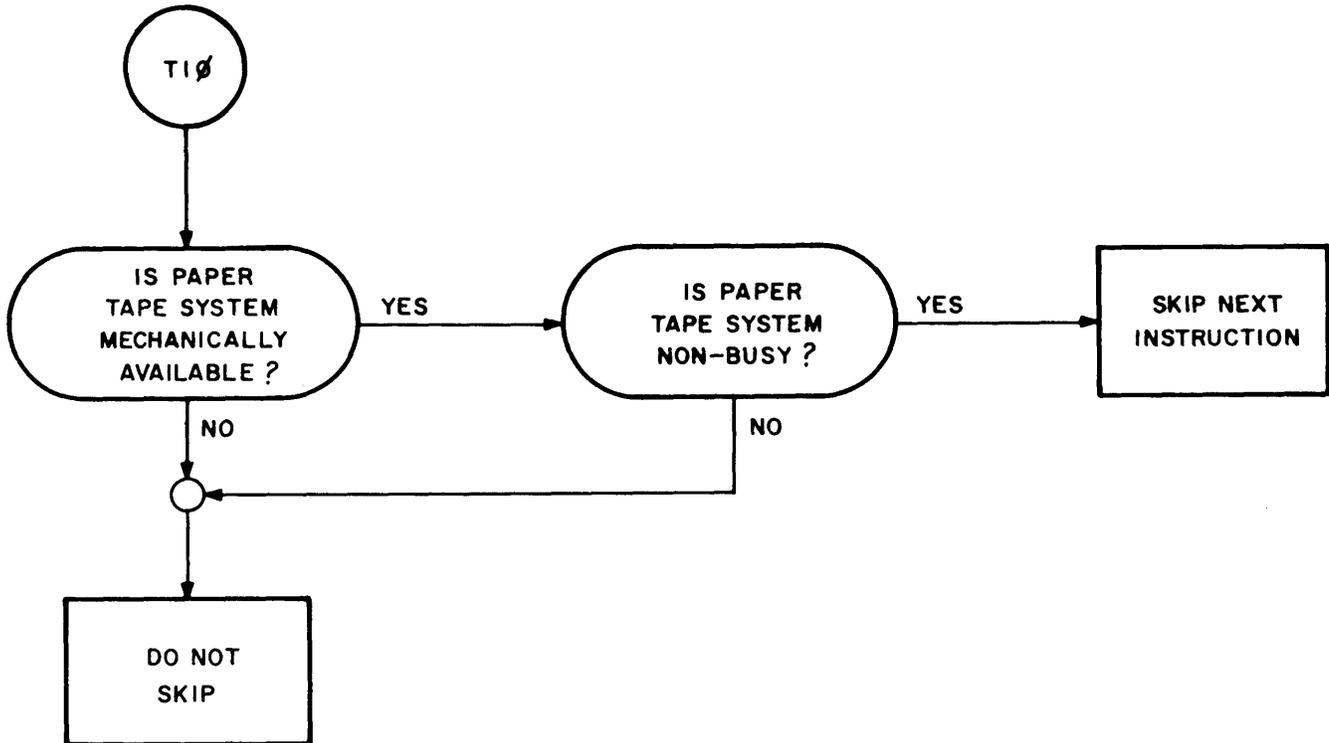
Figure PT-3. Flowchart of Paper Tape System, Model 240, Order Acceptance Procedure
