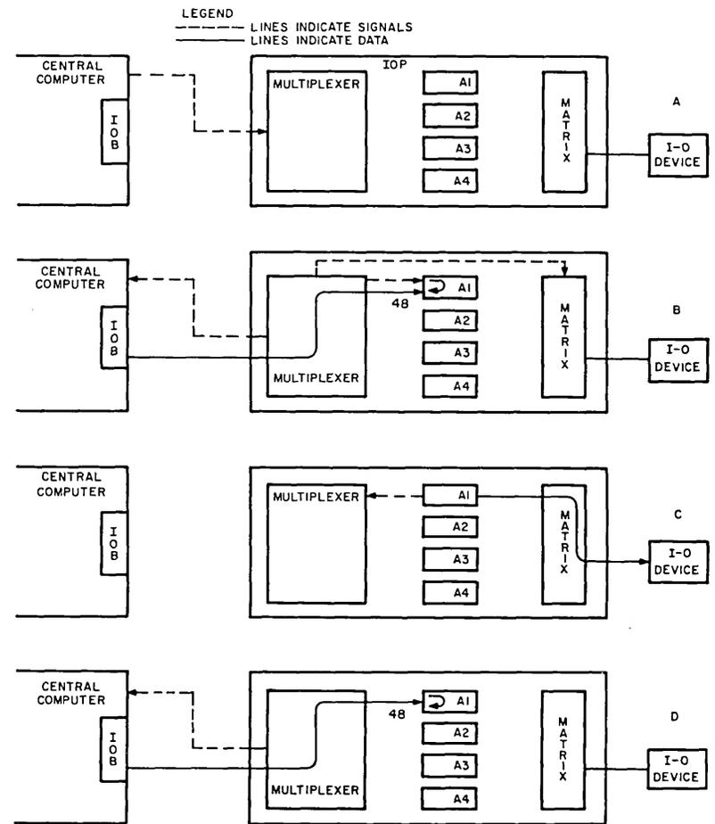
Figure IOP-3. Operation of the IOP During Output Order
