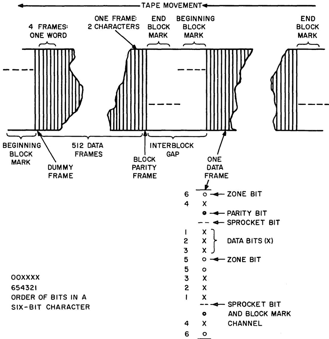
Figure MT-2. Magnetic Tape Format
