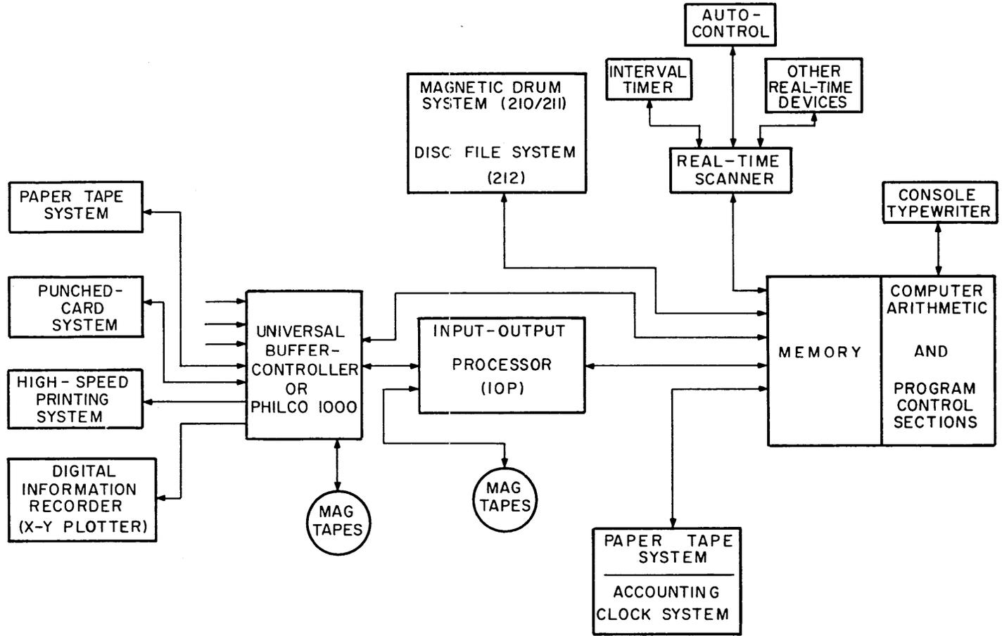
Figure INT-1. Simplified Block Diagram of the Philco 2000 Input-Output Section
