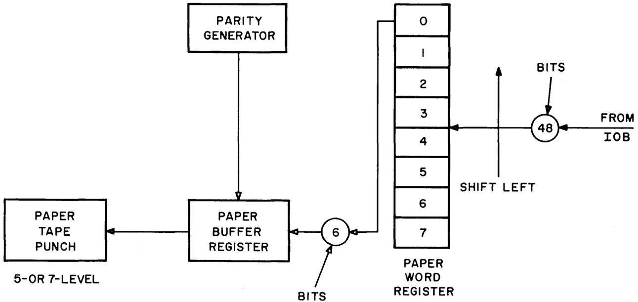
Figure PT-5. Data Flow During Paper Tape System, Model 240, Punching Operation
