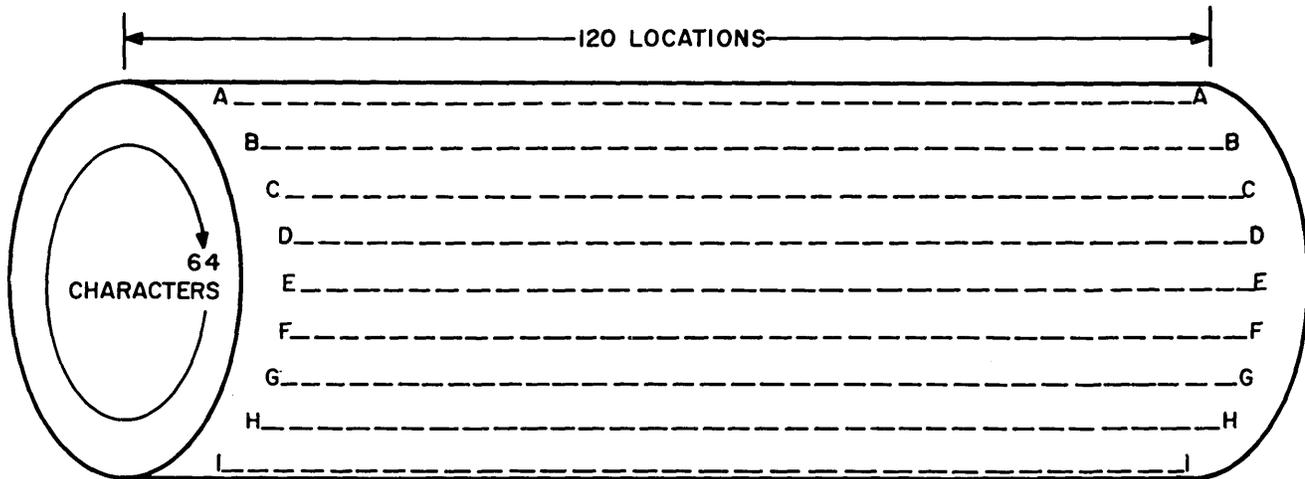
Figure PR-5. Print Roll of High-Speed Printer
