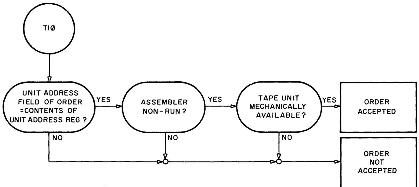
Figure IOP-8. Flowchart of Class C Magnetic Tape Order Acceptance
