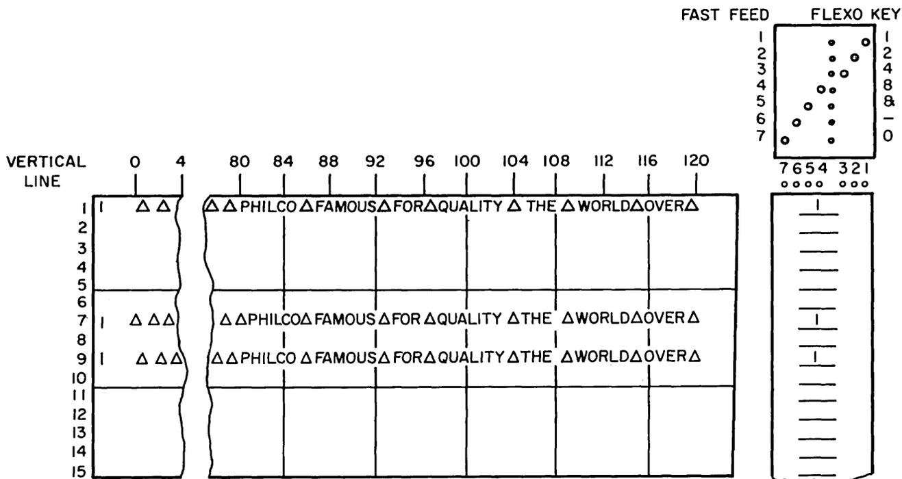
Figure PR-3. Use of Printer Layout Sheet
