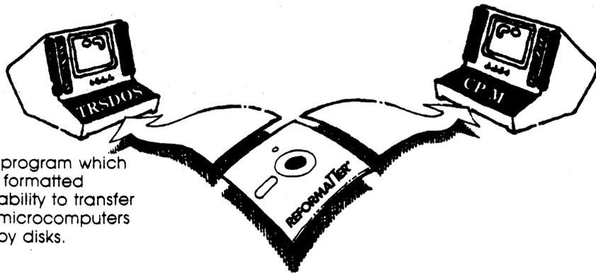
**REFORMATTER**<sup>®</sup> is a diskette utility program which gives the TRSDOS user complete access to CP/M formatted diskettes. With REFORMATTER, you now have the ability to transfer files back and forth between TRS-80 Model II/16 microcomputers and CP/M based computers which have 8" floppy disks.
