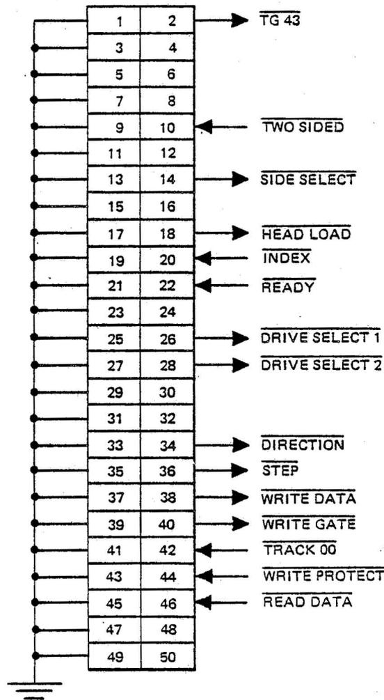
Figure 2-3. Connector Pin Definitions
