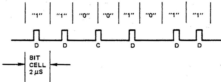
Figure 1-3. MFM Recording Characteristics
