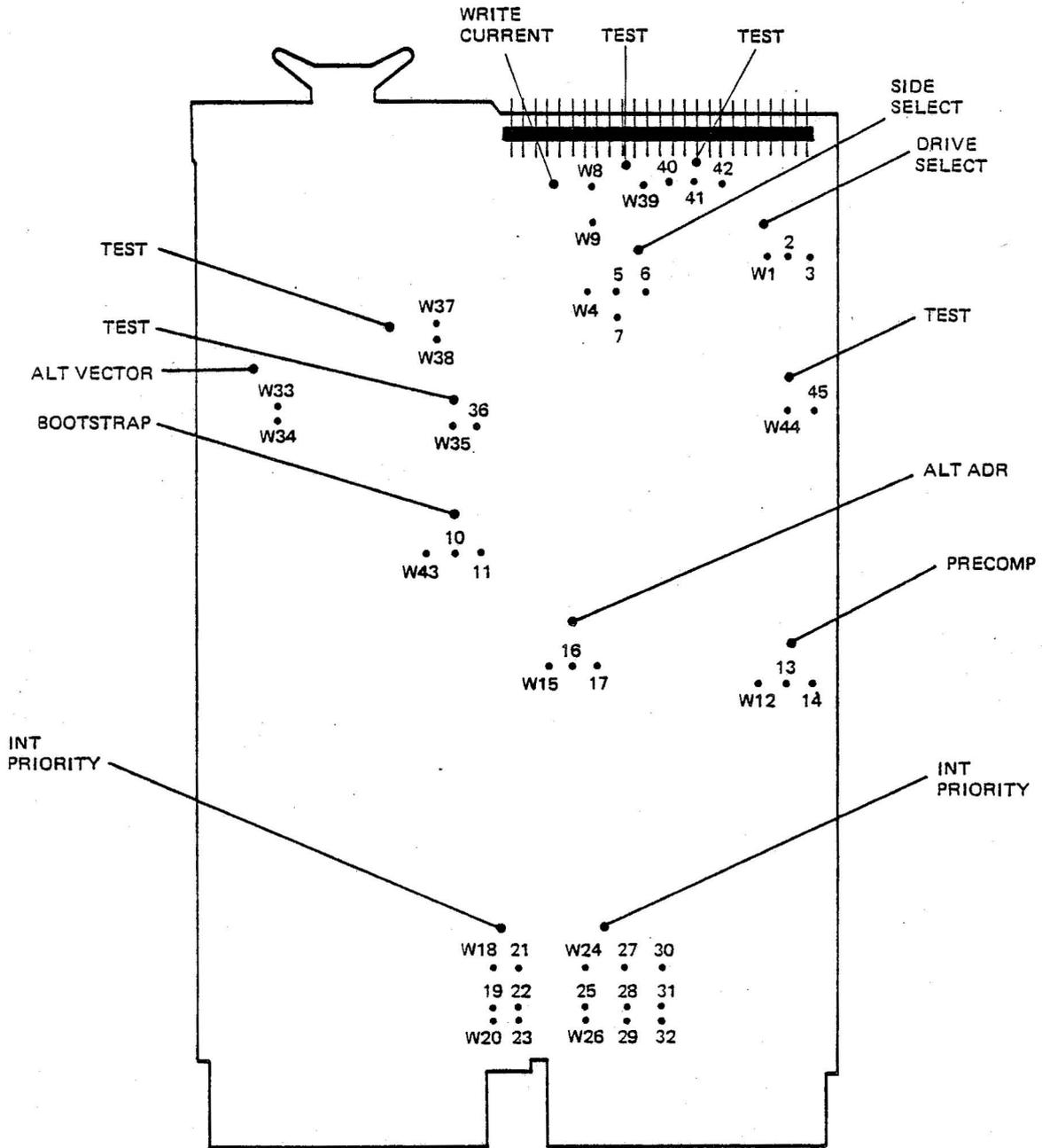
Figure 2-1. PM-XCV21/XCV31 Configuration Jumper Locations
