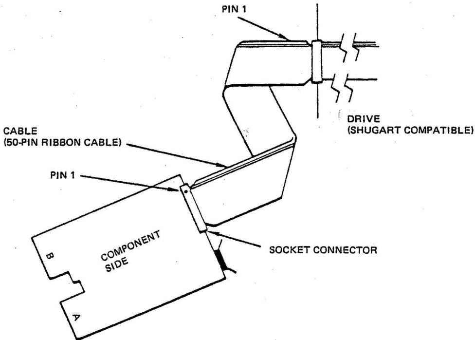
Figure 2-2. Drive/Controller Cabling
