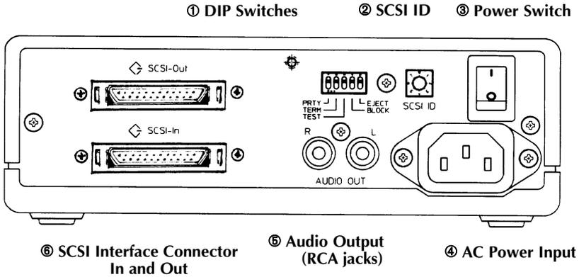
① **DIP Switches:** Use to select parity, term, test, block size, and eject lock options. Leave these switches at their factory settings unless one or more of the following pertain to you:
