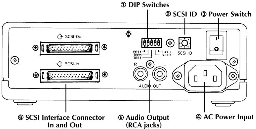
① **DIP Switches:** Use to select parity, term, test, block size, and eject lock options. Leave these switches at their factory settings unless one or more of the following pertain to you:
