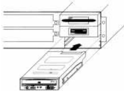
You now need to make the power connection. In most computers, you will find additional power connectors that are ready for your use. Check the cable running from your power supply to your hard disk and see if it has extra connectors on it. If so, you can plug one of these into the power connector found on the rear panel of the CD-RW drive.
