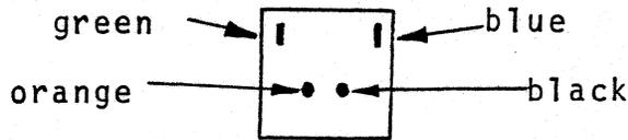
(✓) 25. Insert molex pins into the small female molex connector as shown:
