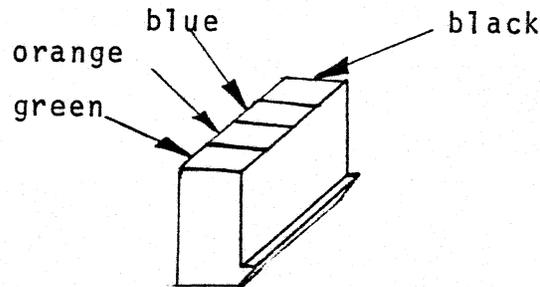
(✓) 26. Insert connector through square hole on front panel and draw the wires through. With the green and blue wires at the top, snap the switch firmly in place.
