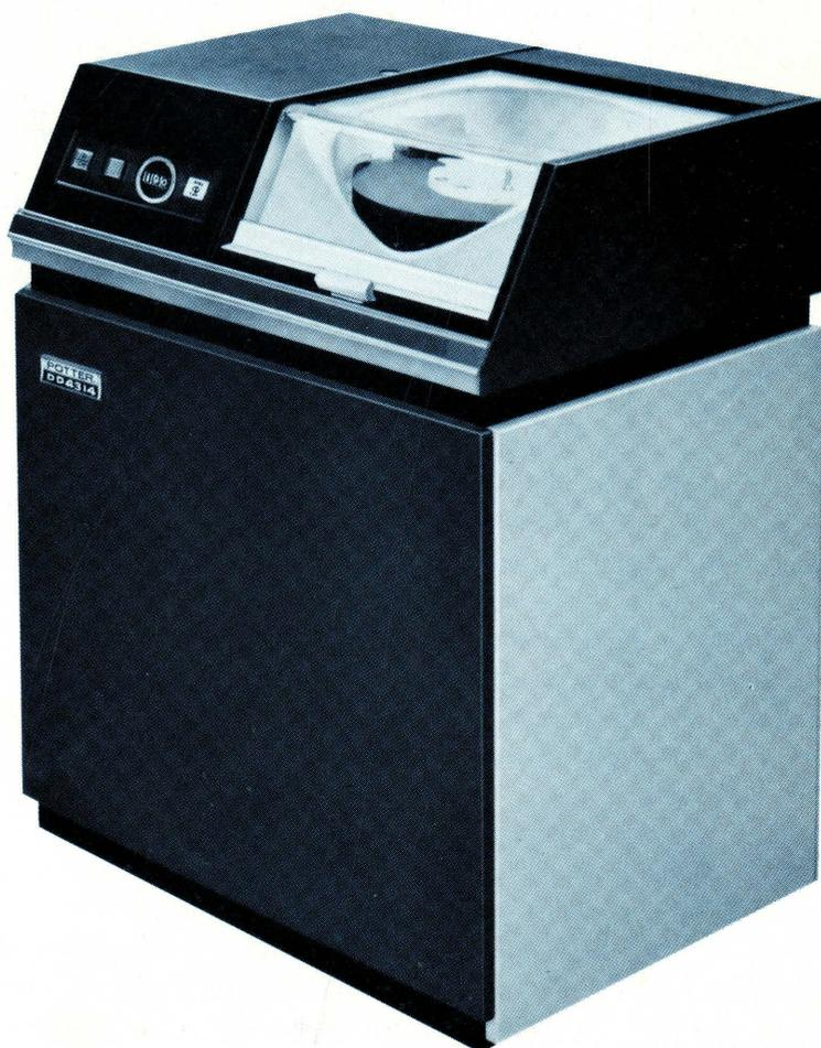
The Potter DD4314-1 Disk Storage Drive is a random access device which provides an "on-line" capacity of 233 million bits. The unit is capable of reading and writing on disk surfaces and utilizes the IBM 2316 Disk Pack or equivalent. Each disk pack can be removed and interchanged between disk drives in a simple and rapid operation.
