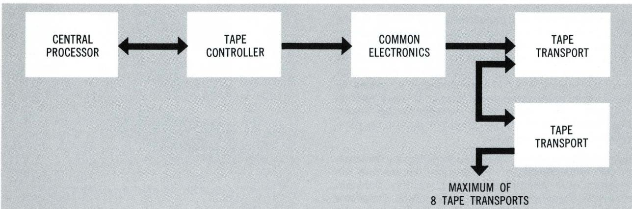
Figure 2. Magnetic Tape System
