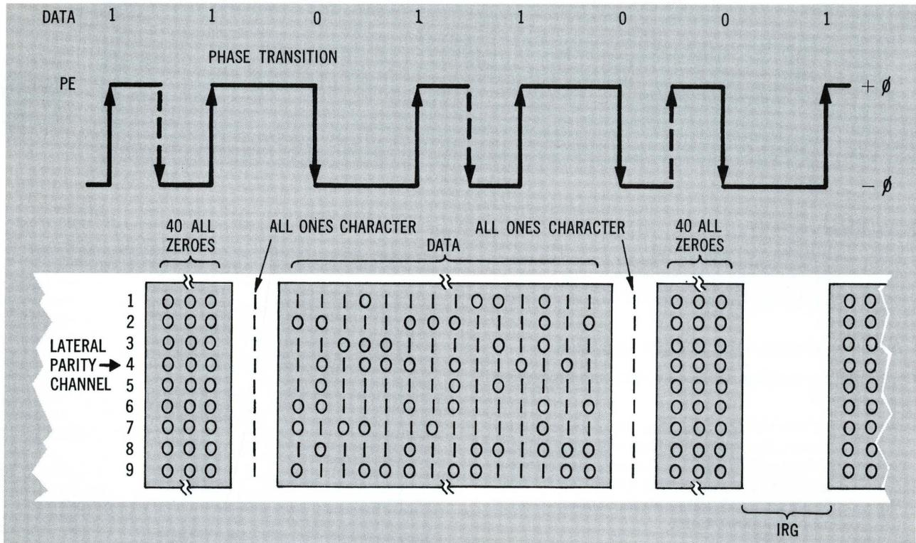
Figure 1. PE Recording Format
