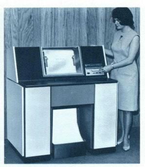
CHARACTER COMPLEMENT Up to 192 different characters may be placed on the horizontally rotating type chain. This unique feature allows a change in code format by simply addressing the required font. For example, 4 sets of 48 characters can be utilized. In addition, any type slug may be changed by an unskilled operator in a matter of minutes. The absence of waving printlines due to misregistration is an outstanding by-product of this system.
