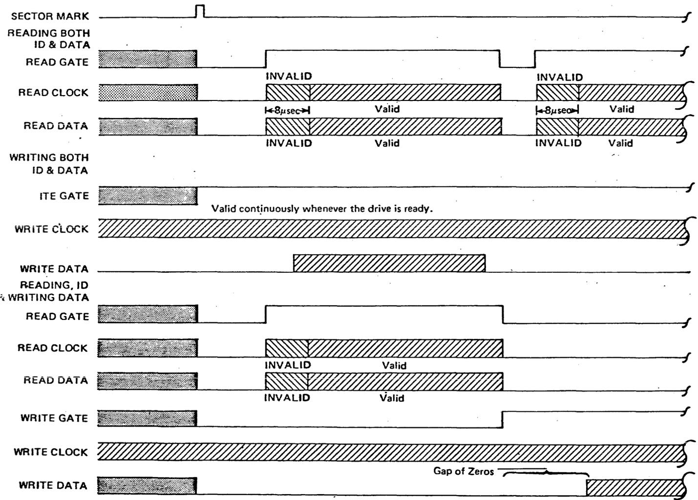
Figure 15. READ & WRITE Transitions During Gaps
