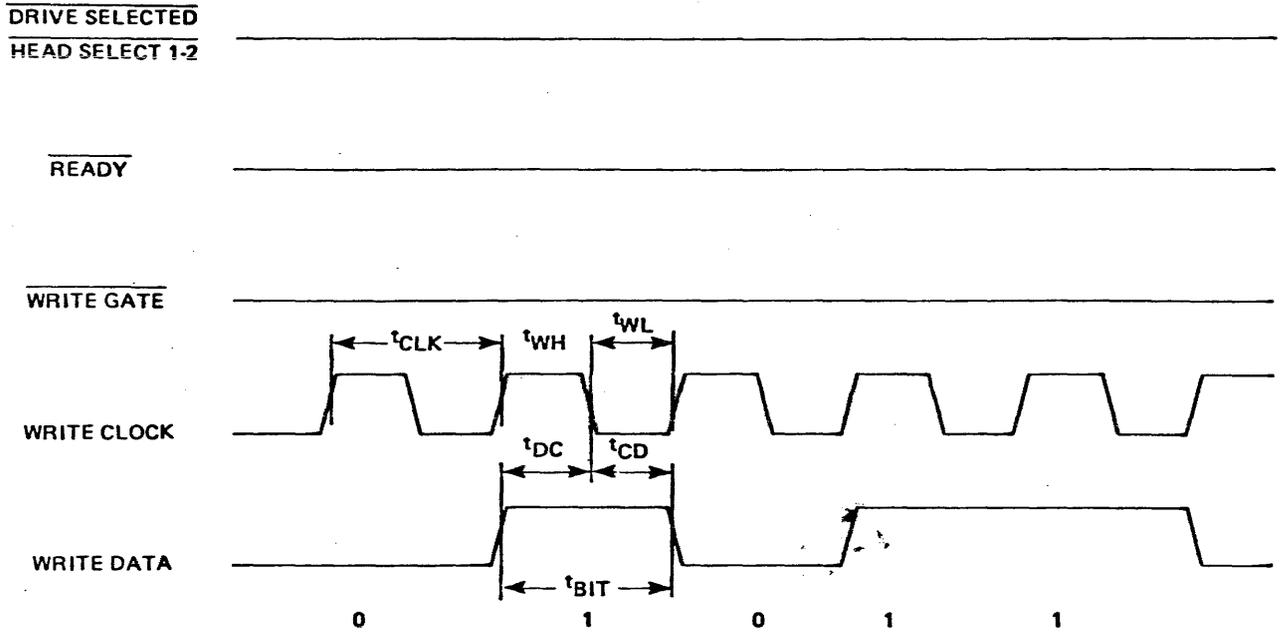
Figure 11. WRITE DATA and WRITE CLOCK Timing
