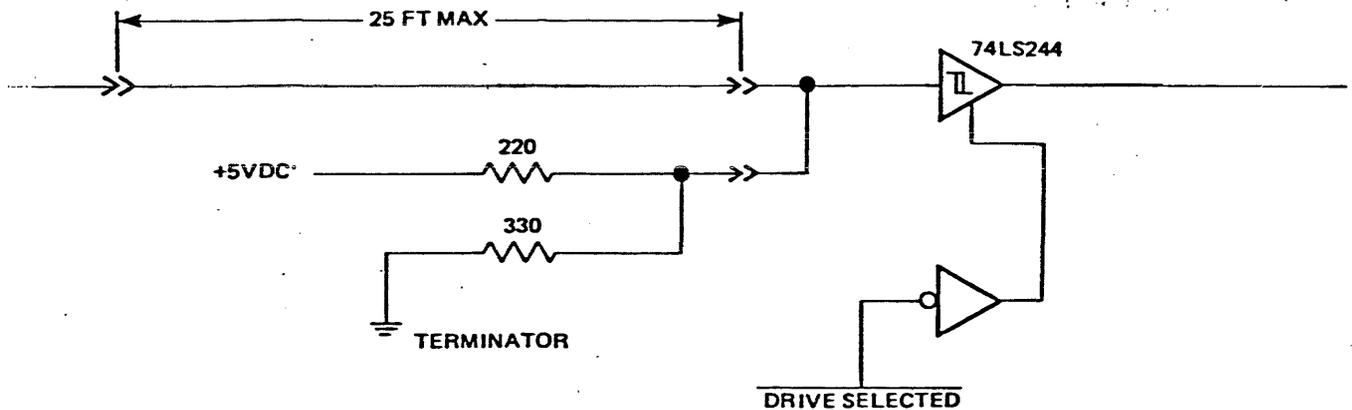
Figure 3. Single Line Receiver Gated By Drive Select
