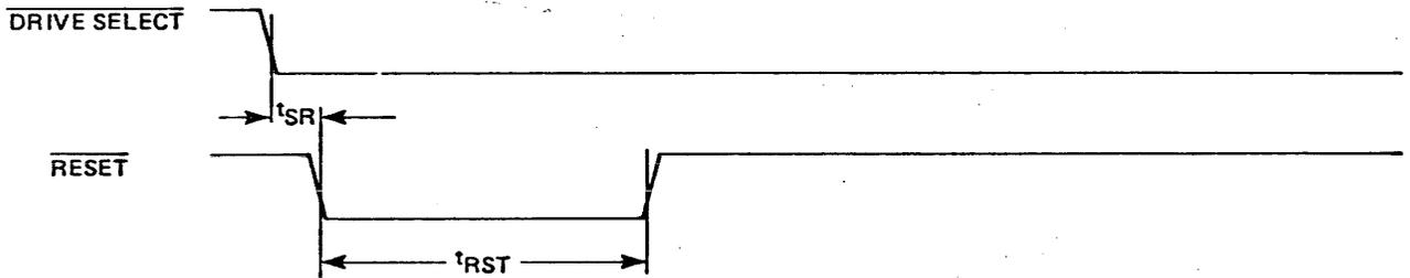
Figure 9. Reset Pulse Width Timing
