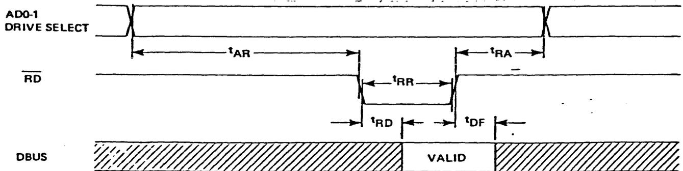
Figure 8. Register Read Timing
