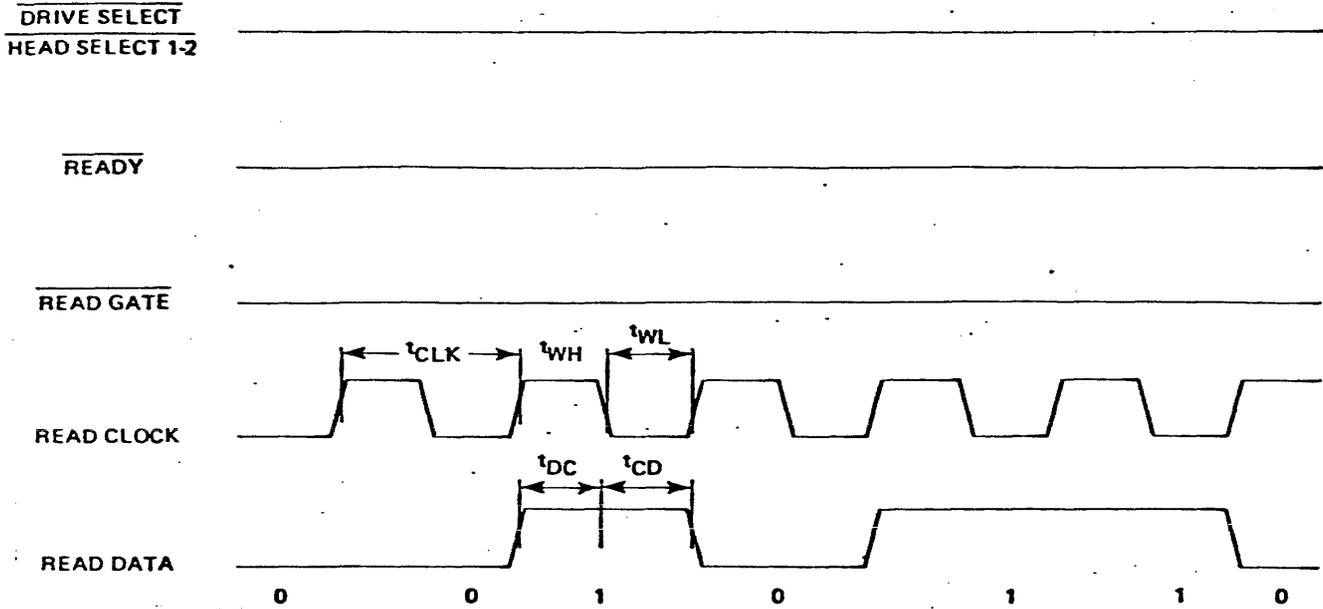
Figure 12. READ DATA and READ CLOCK Timing
