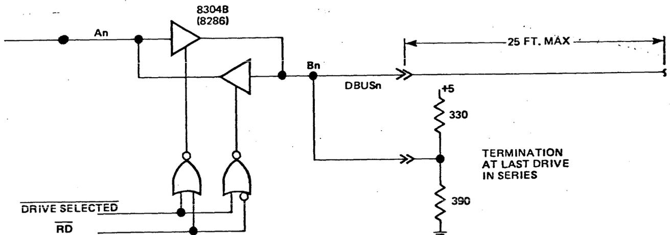
Figure 2. DBUS Transceiver
