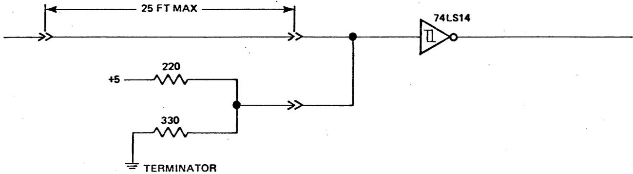
Figure 4. Single End Line Receiver
