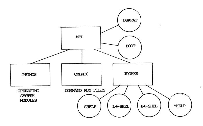
Figure 2-2. Typical portion of PRIMOS File System, Showing: MFD, Command UFD, and User UFD.
