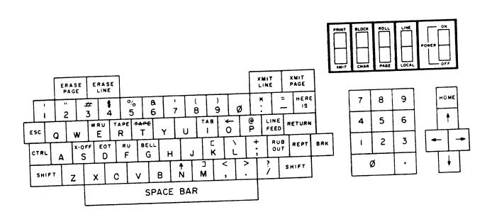
Figure 2-1. Typical Terminal Keyboard
