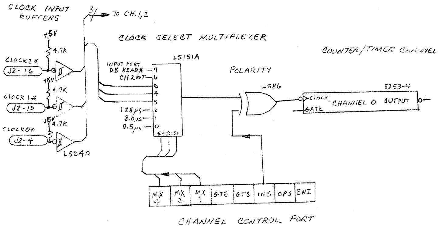
Figure 3-2-A Clock Control Circuit for Channel 0
