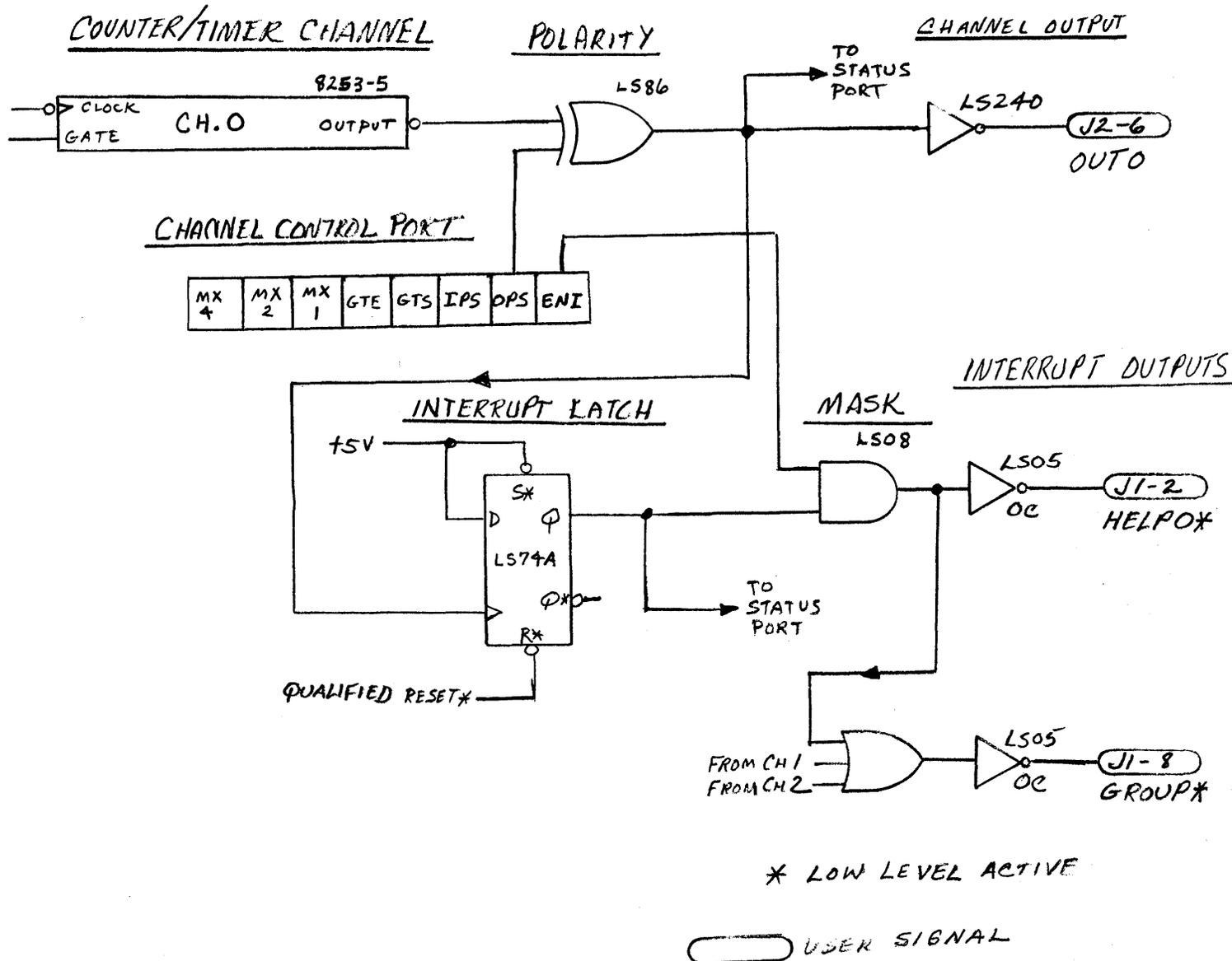
Figure 3-2:C Channel 0 Interrupt Circuit for the 7308 (typical of all channels)
