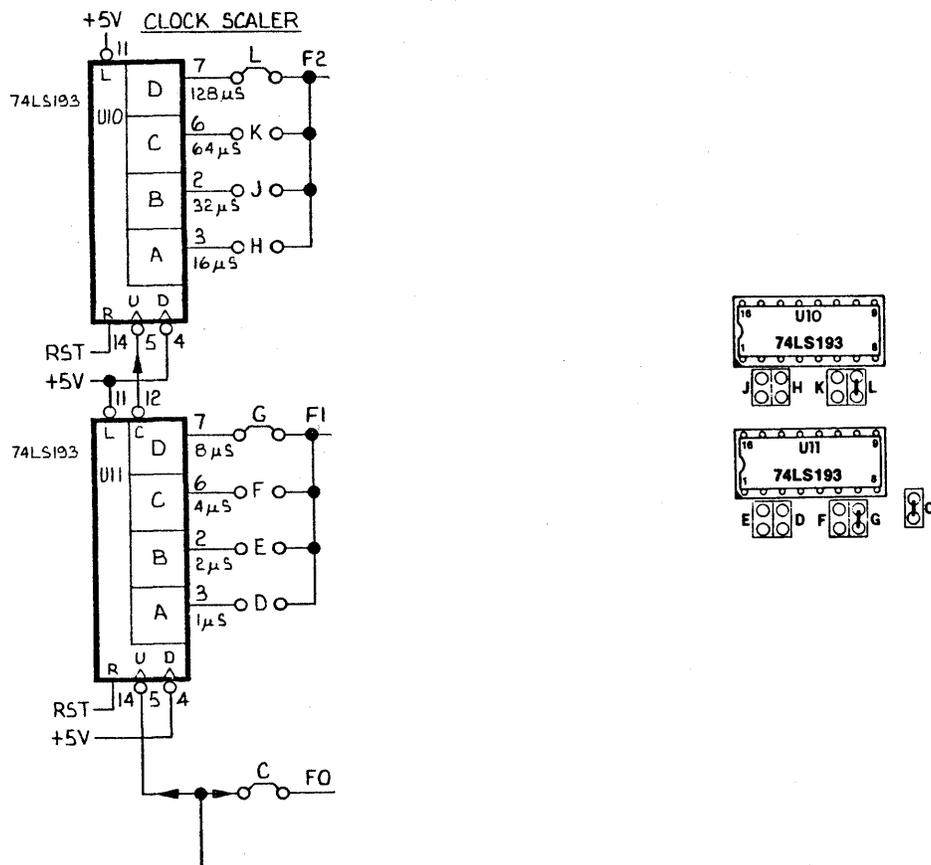
Figure A-2. Clock Scaler Output Jumpers
