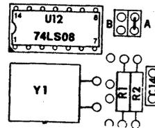
Figure A-1. External Clock Input Option
