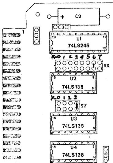
FIGURE 2-3: DECODER JUMPER PAD NUMBERING (TYPICAL)
