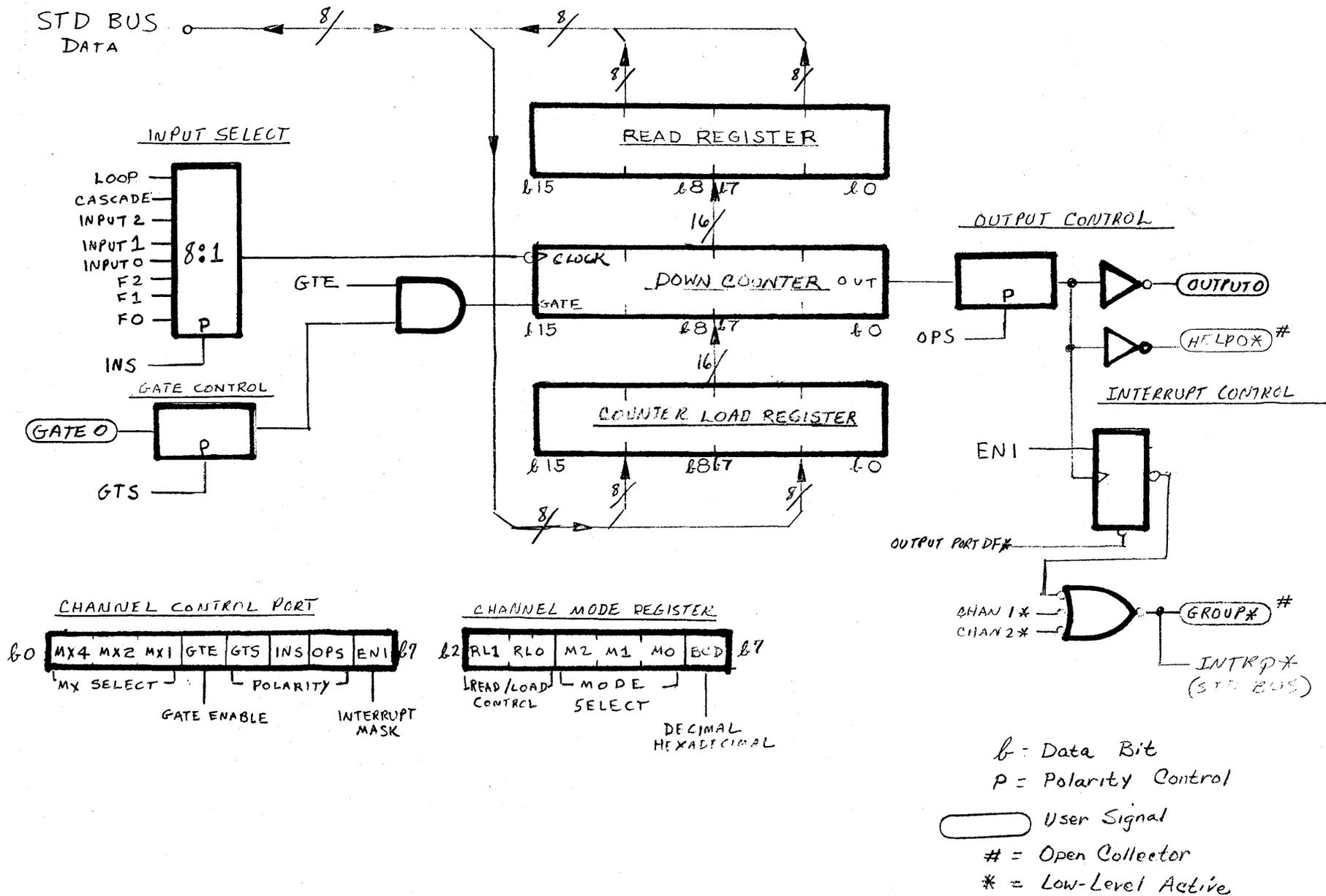
Figure 3-1. Logical Organization of 7308's Counter/Timer Channel 0 (Typical of all channels)
