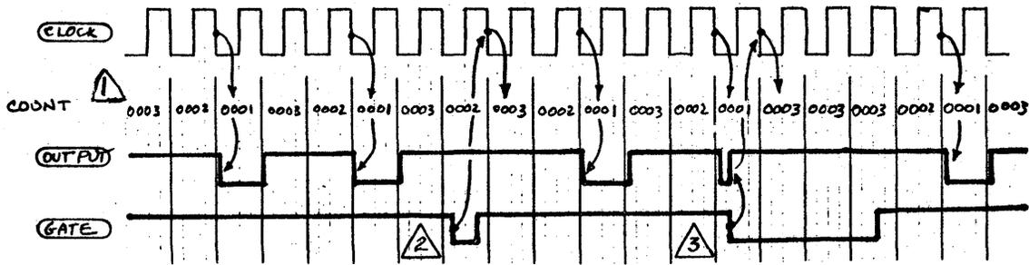
Mode 2: Rate Generator or Divide-by-N Counter with AutoReload
