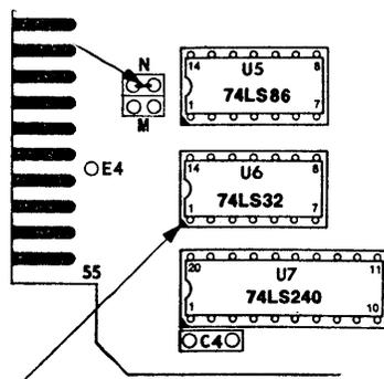
Figure A-3. Interrupt Output Jumpers
