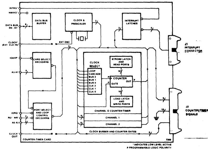
Figure 1-2. Block Diagram of 7308 Multichannel Counter/Timer Card.
