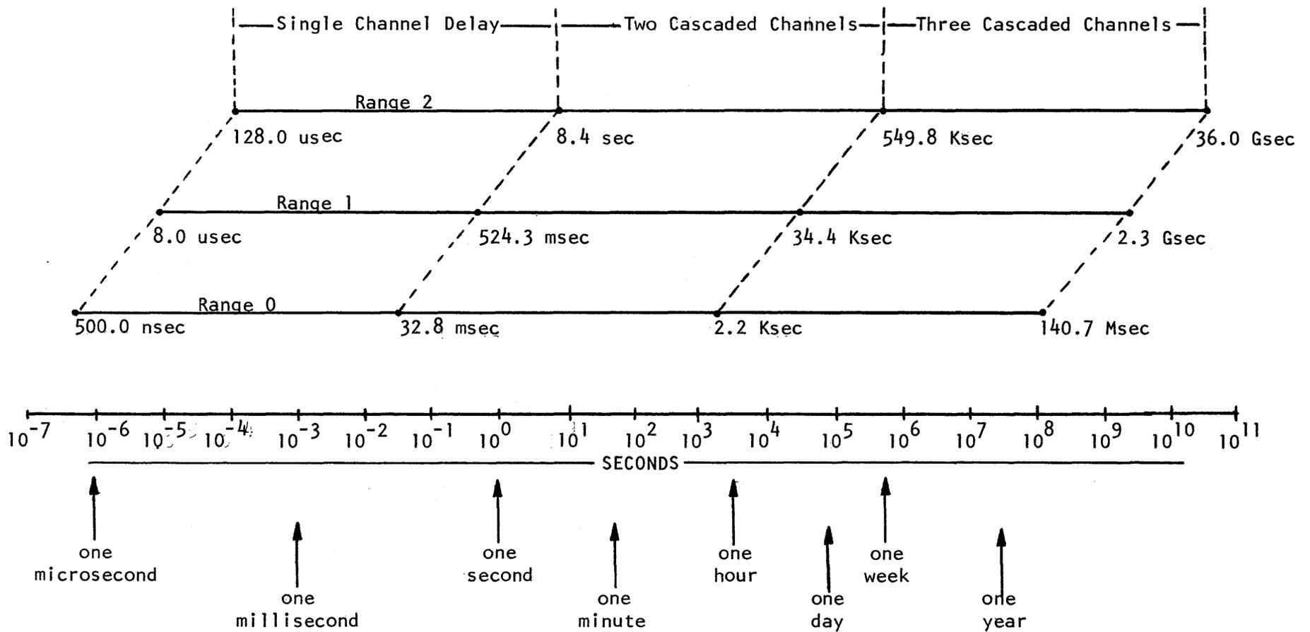
FIGURE 3-9: SINGLE CHANNEL AND CASCADED CHANNEL DELAY RANGES
