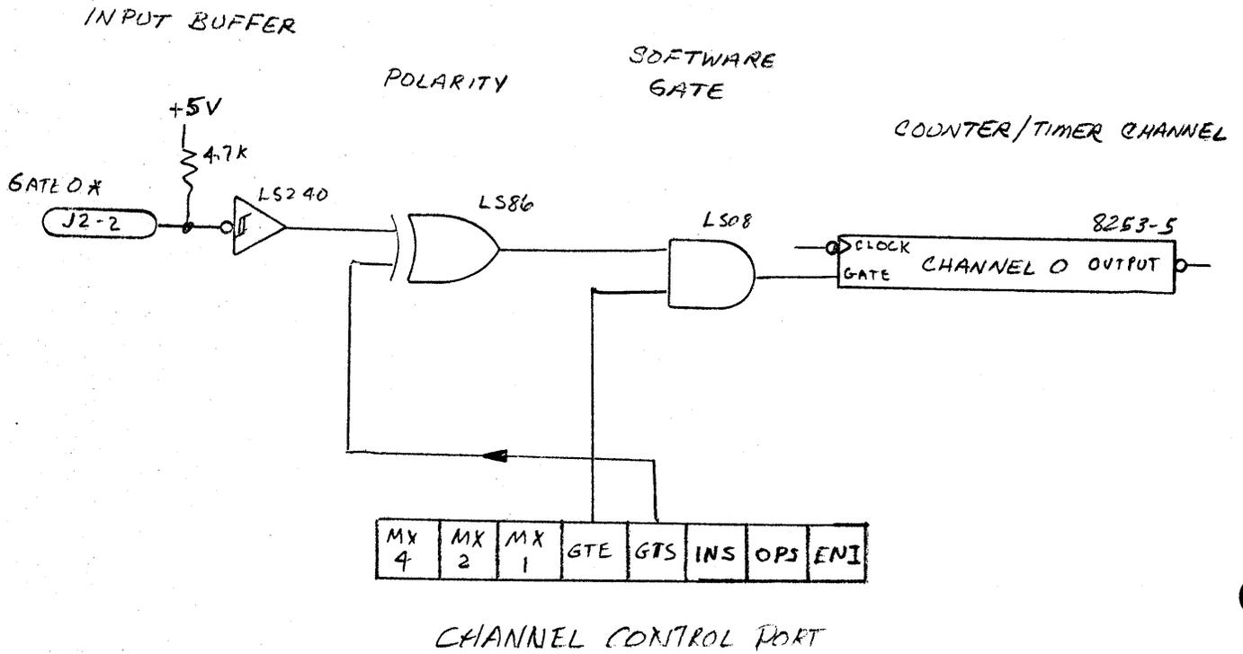
Figure 3-2-B. Gate Control Circuit for Channel 0
