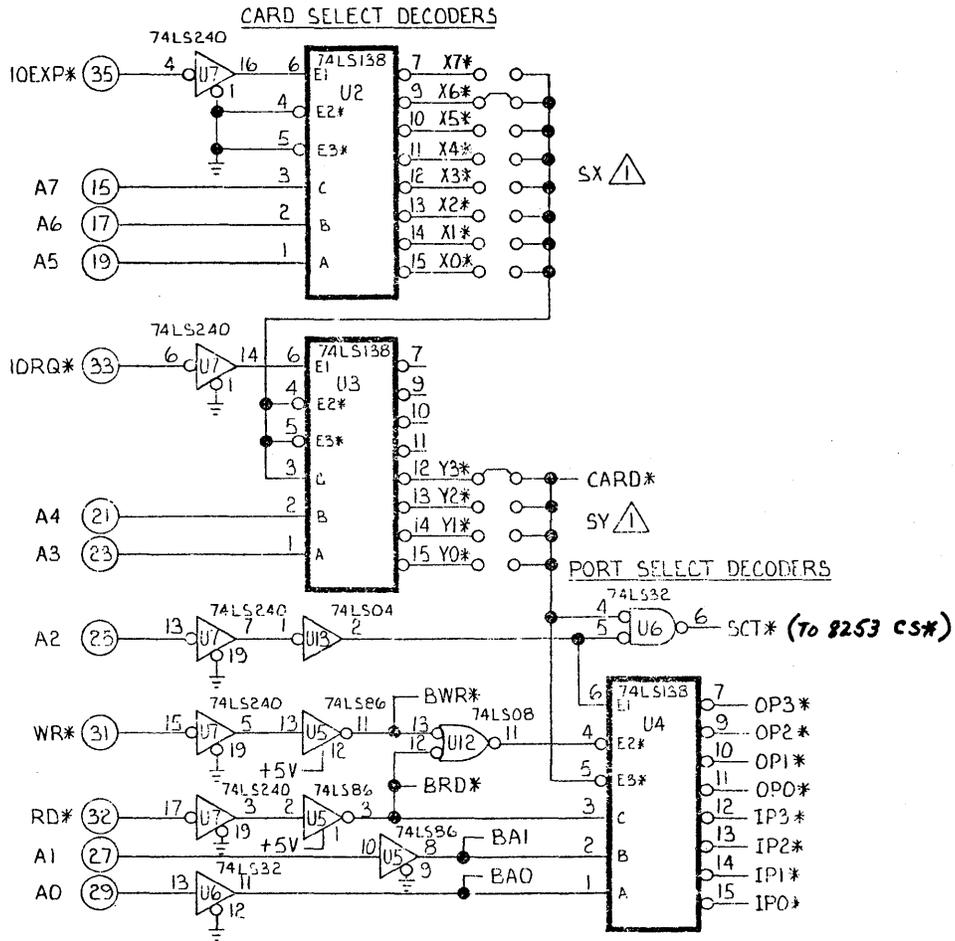
FIGURE 2-2: 1/0 PORT SELECT CIRCUIT (TYPICAL)
