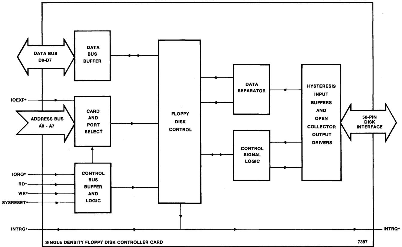
Figure 1-2. 7387 Block Diagram.
