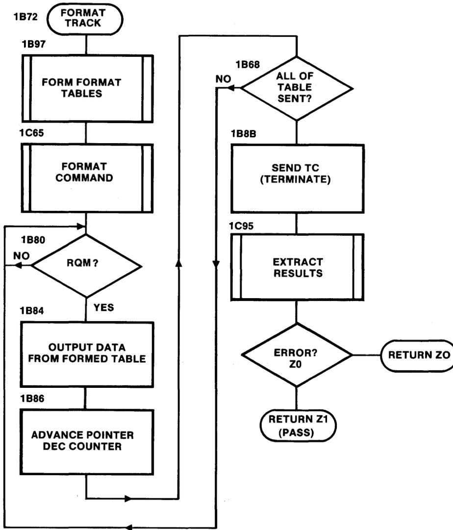
Figure 4-9 . 7387 "Format Track" Flowchart
