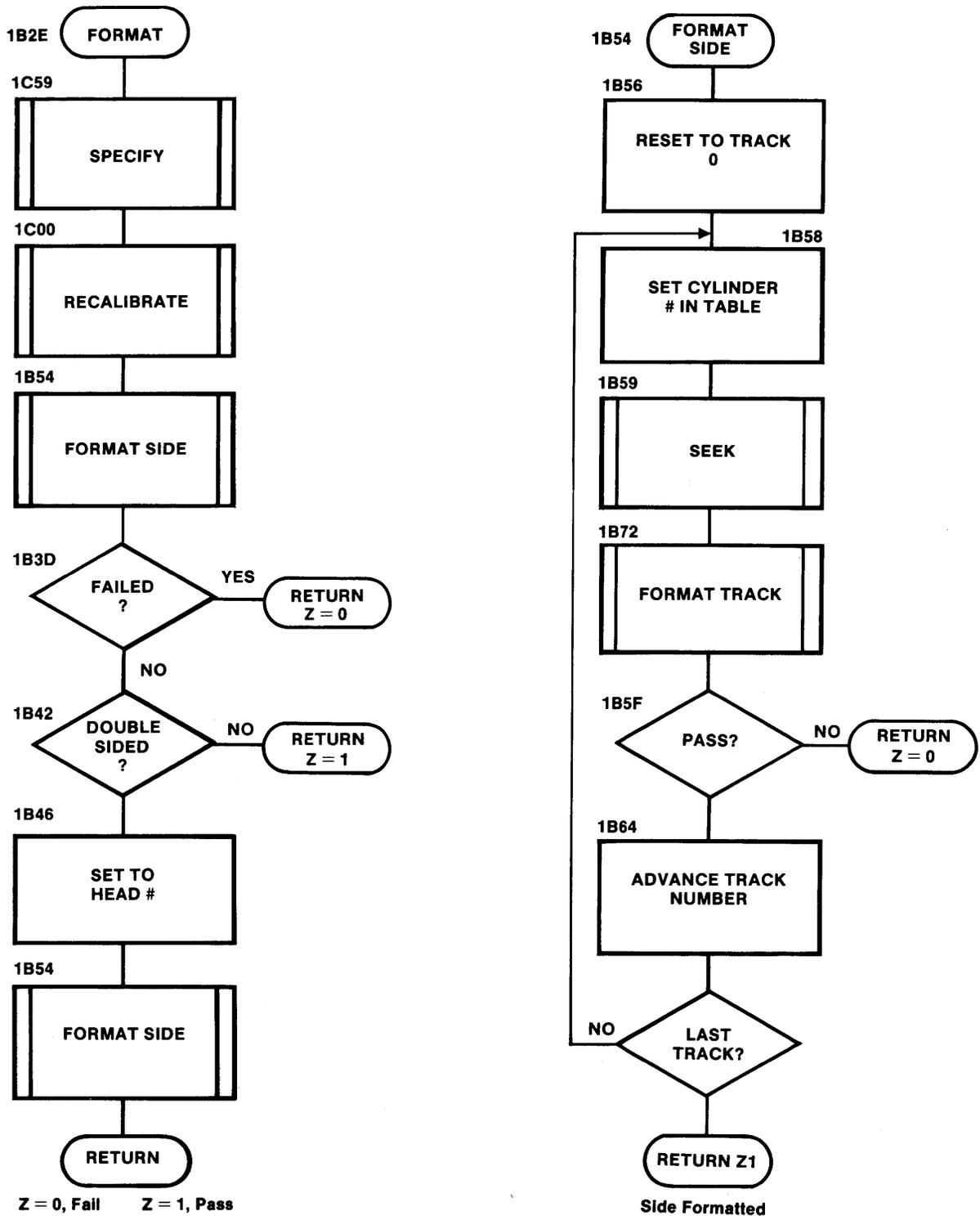
Figure 4-8. 7387 "Format" and "Format Side" Flowchart
