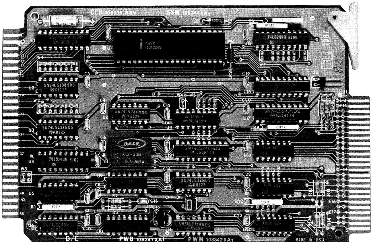
Figure 1-1. 7387 Floppy Disk Controller Card.
