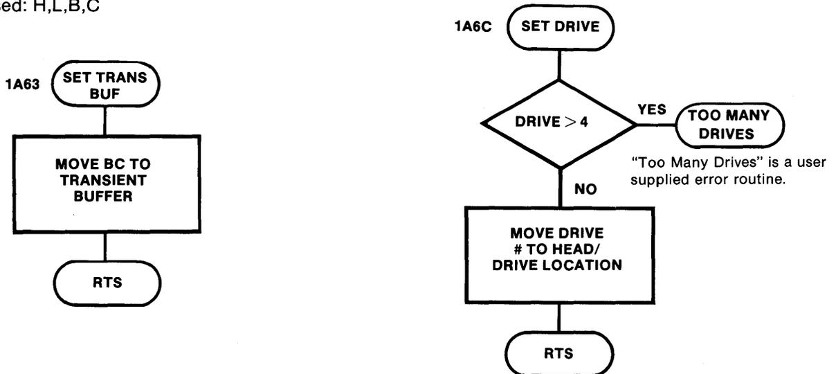
Figure 4-14. 7387 "Set Trans Buf" and "Set Drive" Flowchart
