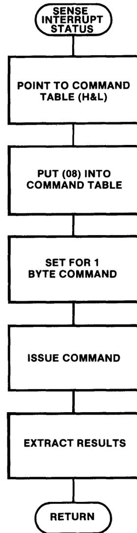
Figure 4-12. 7387 "Sense Drive Status" and "Sense Interrupt Status" Flowchart
