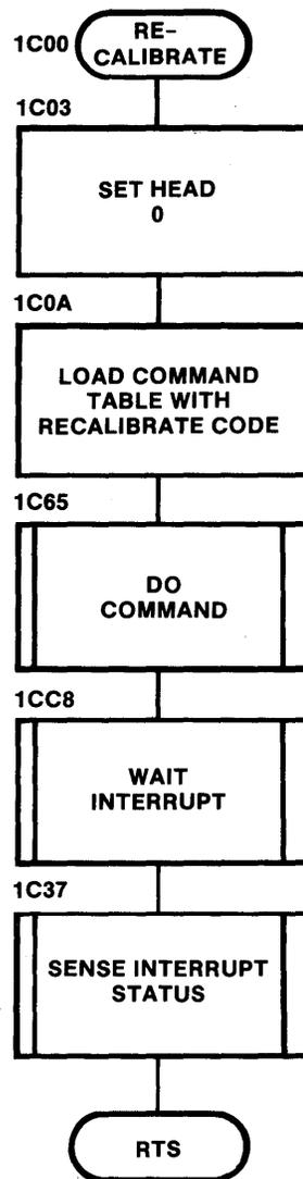
Figure 4-11. 7387 "Seek" and "Recalibrate" Flowchart
