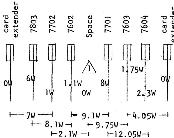
As above except 1" spacing on component side of 7701 RAM card.
