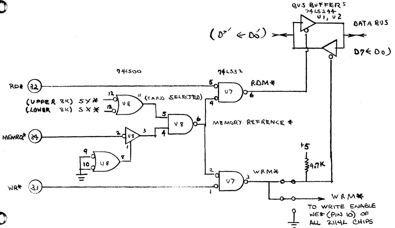
The write strobe to the 2114L chips and the read/write control signals for BUS BUFFER directional control is the implementation of the following Boolean Logic:
