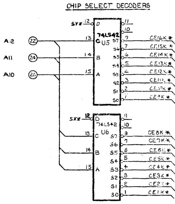
Each chip enable line goes to pin 8 (CE\*) of a pair of 2114L chips, (1K block) The lower ten address lines are used for direct addressing of the 1K chip pairs, and are buffered by U3 and U7.
