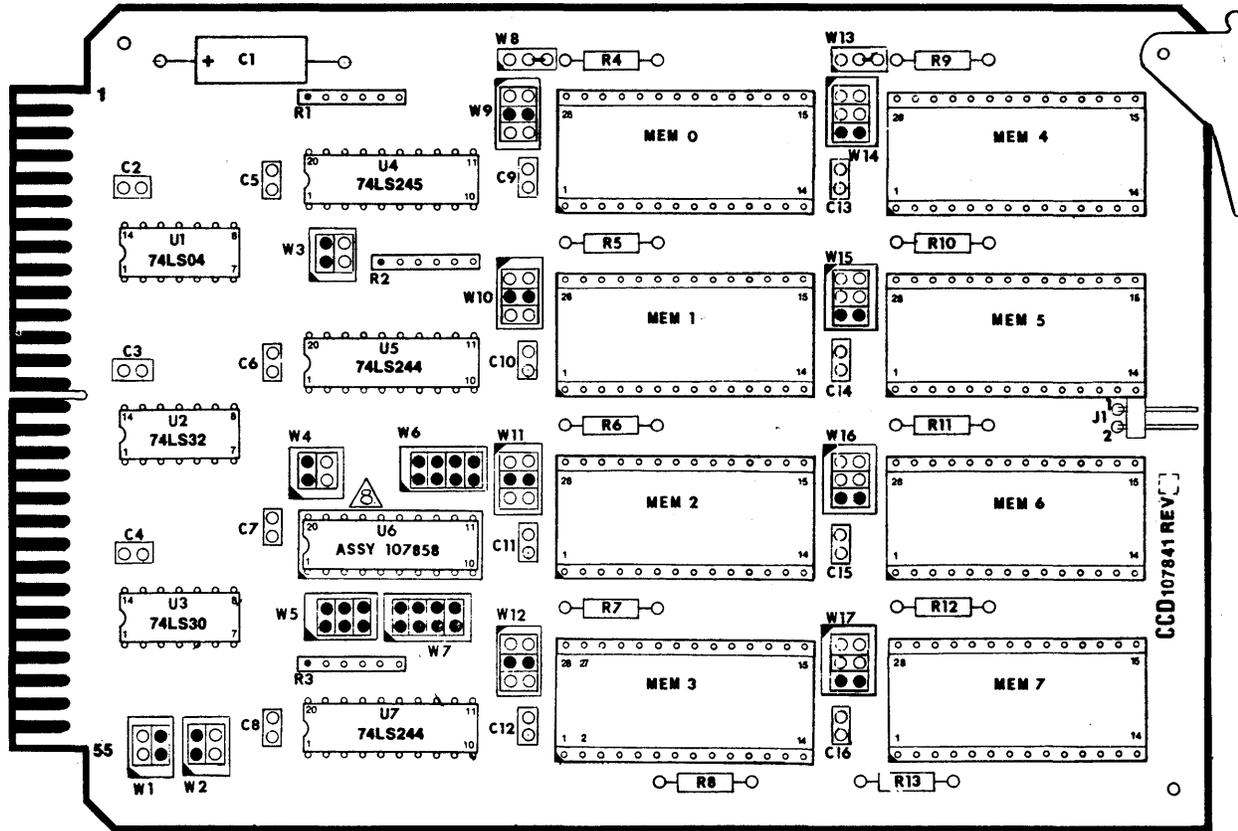
Figure 2-4. Physical Locations of Features on the 7704 Card
