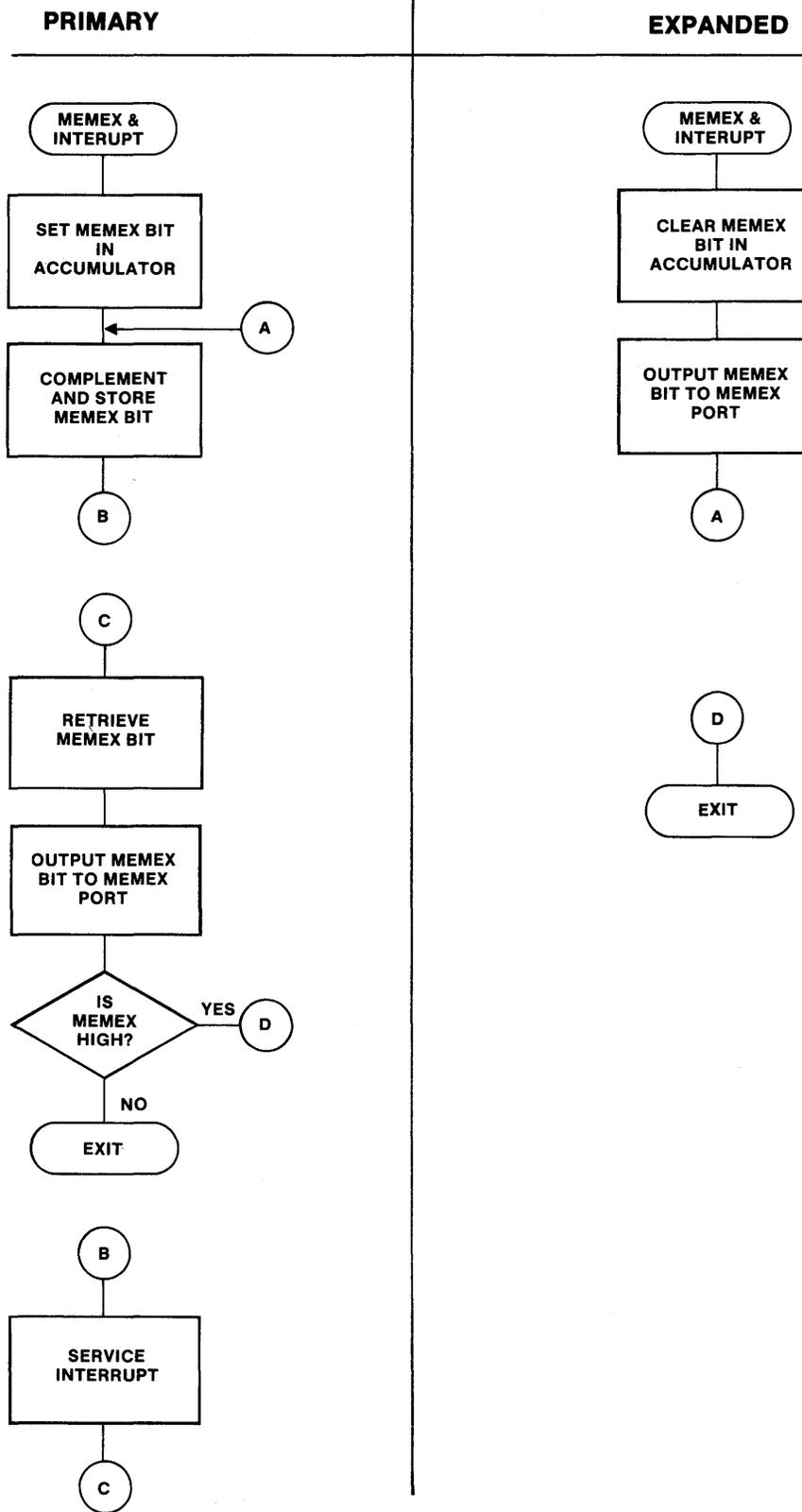
Figure 3-11.7704, MEMEX, Interrupt Software Flowchart
