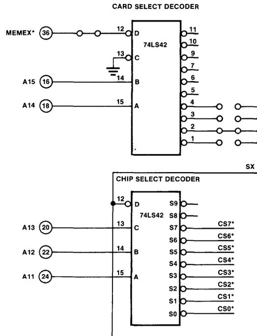
Figure 2-12A Address Decoder Schematic For 2K Memory Blocks (16K Memory Card)
