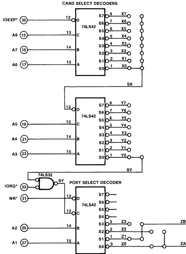
Figure 2-16A I/O Address Decoder And Schematic For 2 Addresses Per Card
