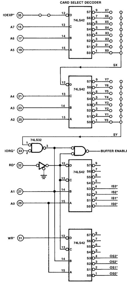
Figure 2-17A I/O Address Decoder And Schematic For 4 Addresses Per Card
