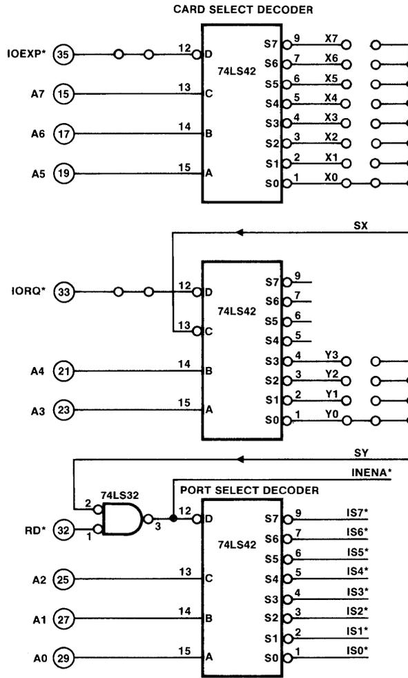
Figure 2-18A I/O Address Decoder And Schematic For 8 Addresses Per Card
