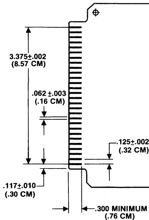
Figure 1-7B Recommended Edge Card Finger Design
