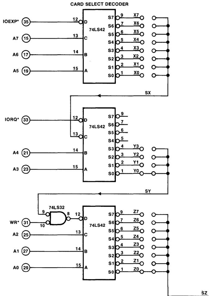
Figure 2-15A I/O Address Decoder And Schematic For 1 Address Per Card
