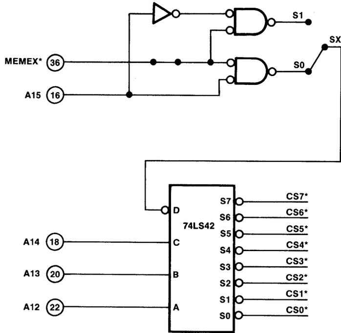
Figure 2-13A Address Decoder Schematic For 4K Memory Blocks (32K Memory Card)
