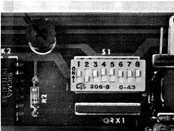
Figure 8. CUTS Switches
