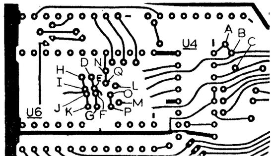
Step 2 Install a 74LS00 IC in the SPARE IC pattern on the board. Be sure to connect +5V and GND to the chip using the conveniently located traces on the bottom side of the board.
