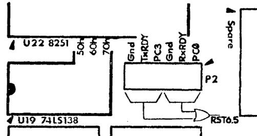
Of course it is also possible to use interrupt signals other than the four mentioned above. Just cut trace 5-6 or 11-12 and connect the desired interrupt signal to pads 2-4-6 or 8-10-12 as above.
