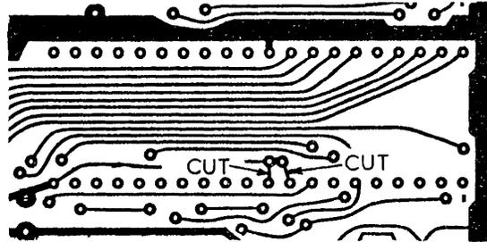
NOTE: If the DMA option is later removed (chips U15 and U16 removed) these traces MUST be re-installed or the SCCS-85 will not operate.
