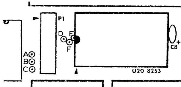
At this point possible reconfigurations should be apparent. If it is desired to supply any of the timers with clocks other than the CPU clock, one need only cut the appropriate trace under P1 (or trace D-E in the case of timer 1) and connect the desired clock. Note that if the clock is originating off the board, pin 1 of J3 has been conveniently routed to pin 9 of P1 for the user to connect to whatever he pleases.
