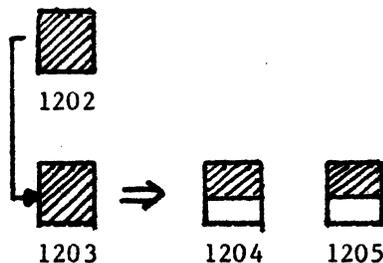
Adding new entry to 1202 for split above causes 1202, level 1, to split. 1202 is divided in half and two new sectors, 1206 and 1207 are written to disc. Sector 1202 is added to system stack for Delete.
