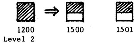
A new level 3 sector, containing pointers to the two, new level 2 sectors, is built in memory.
