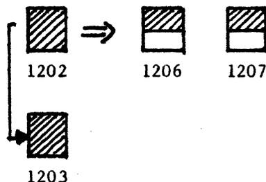
Sector 1200 is read in, the pointer pointing to 1202 is changed to point to one of the new level 1's, and an entry is made for the additional level 1. Sector 1200, which reflects all of the splits made, is rewritten to disc and the sectors in the system stack are Deleted. (See "Splitting Top Key Sector" if addition to the level 2 causes it to split).
