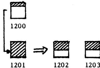
Sector 1200 is read in and adjusted to point to 1202 and 1203. If no new splits are required, sector 1200 is written to disc.
