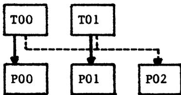
T00 and T01 are Controlling Terminals to Partitions P00 and P01. Partition P02 is a Background Partition and can be ACTIVATED by any program in partitions P00 or P01.
