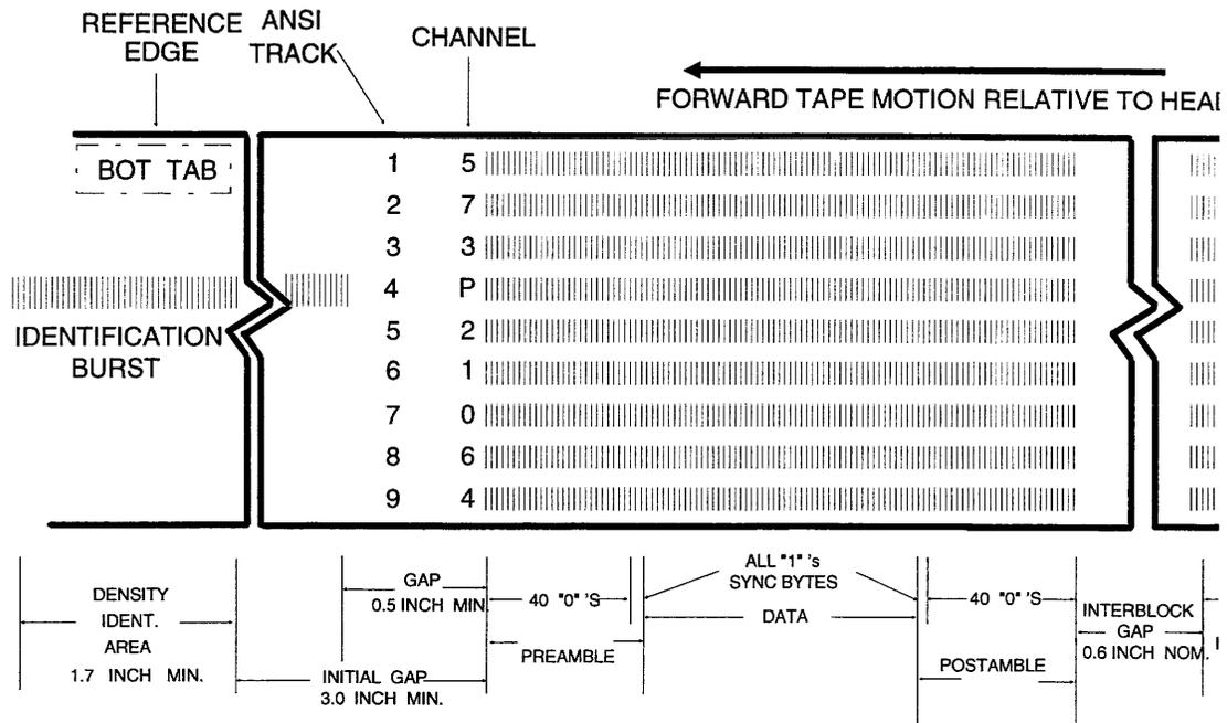
Figure 2-1 PE Data Tape Format
