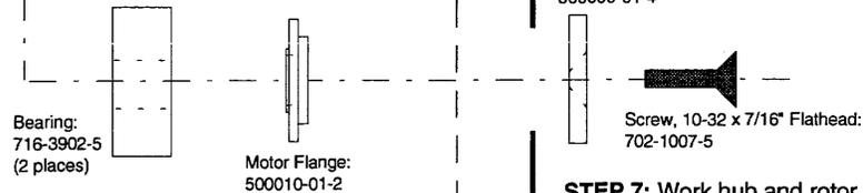
**DO NOT FORCE BEARINGS INTO POSITION WITH THE USE OF TOOLS.**
