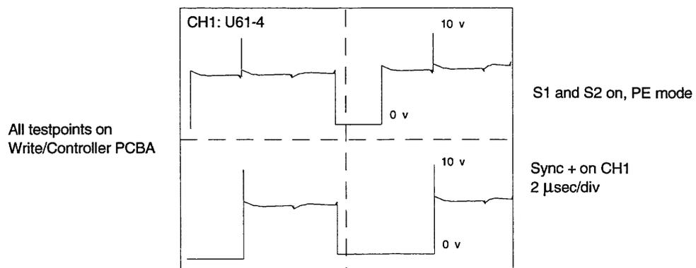
Figure 3-6 Write Head Driver Waveforms
