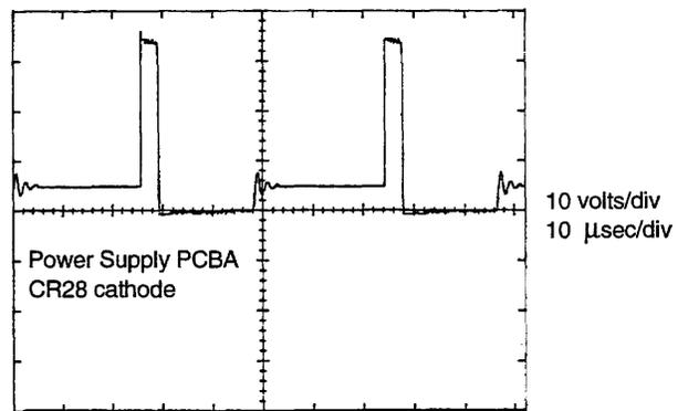
Figure 3-12 +5 Volt Regulator without Load
