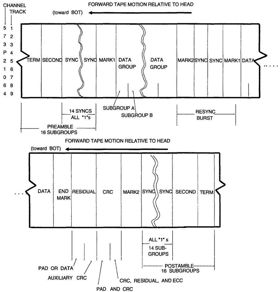
Figure 2-3 GCR Data Tape Format
