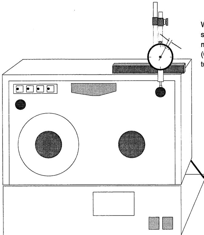
When the runout is within spec, the pointer will not move more than one division (0.0005 inch) during one full turn of the tape guide.
