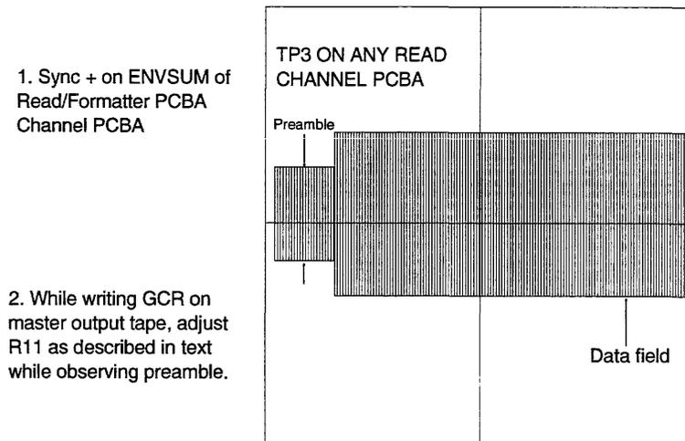
Figure 7-4 GCR Write Current Adjustment Waveform
