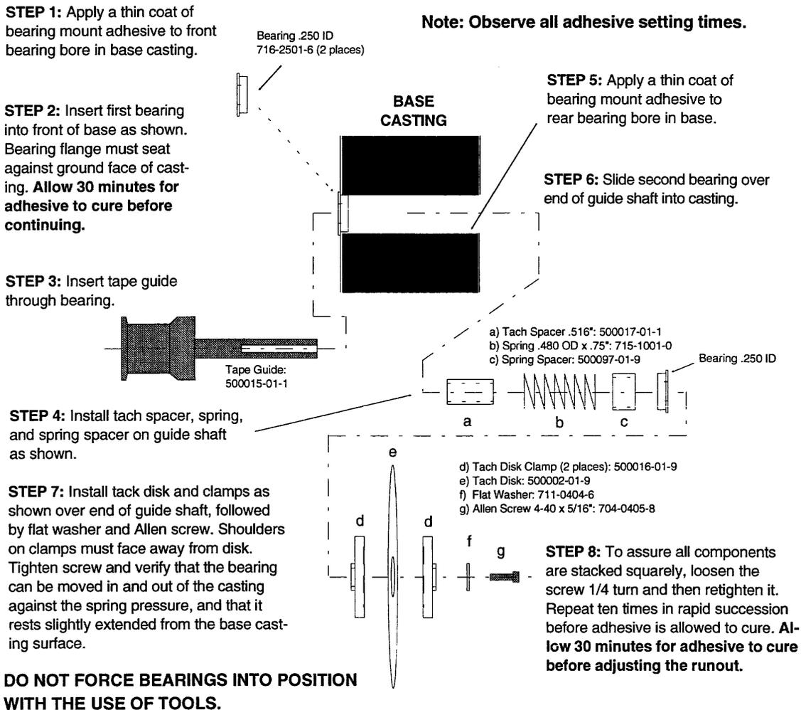
Figure 8-2 Tachometer Tape Guide Assembly
