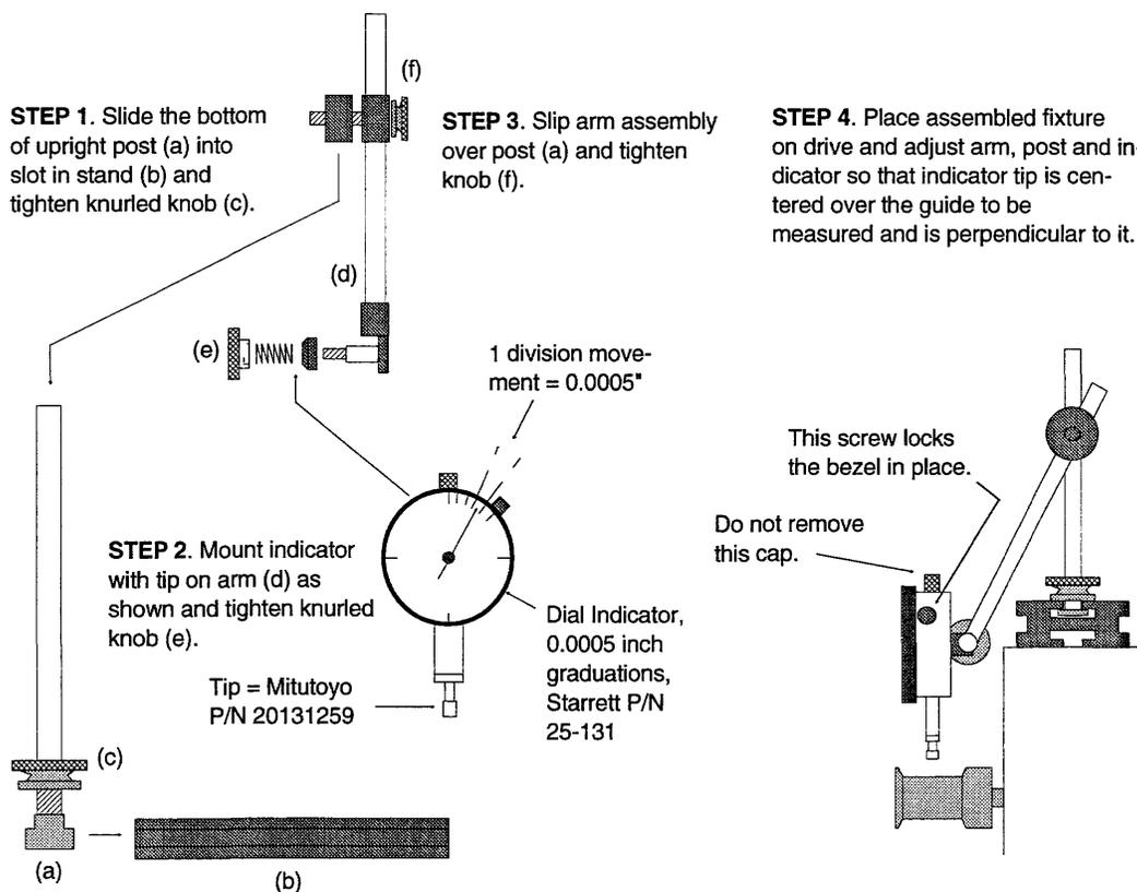
**Note:** *The tip of the indicator should be flat to provide a line of contact with the tape guide. A round tip will provide a point of contact which may scratch the finish on the tape guide and cause future tape damage. Always use a flat tip, such as Mitutoyo P/N 20131259 or equivalent.*
