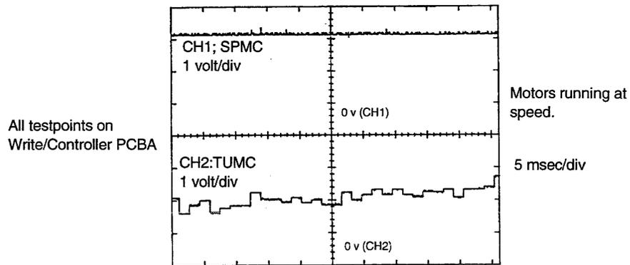
Figure 3-5 Supply and Take Up Motor Waveforms
