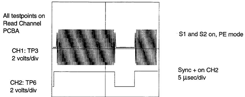
Figure 3-4 Read Analog and Envelope Waveforms
