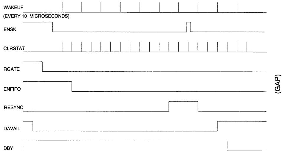
**Figure 3-3** Relative Read Timing Diagram
