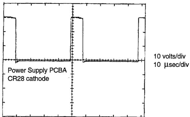
Figure 3-11 +5 Volt Regulator with Load
