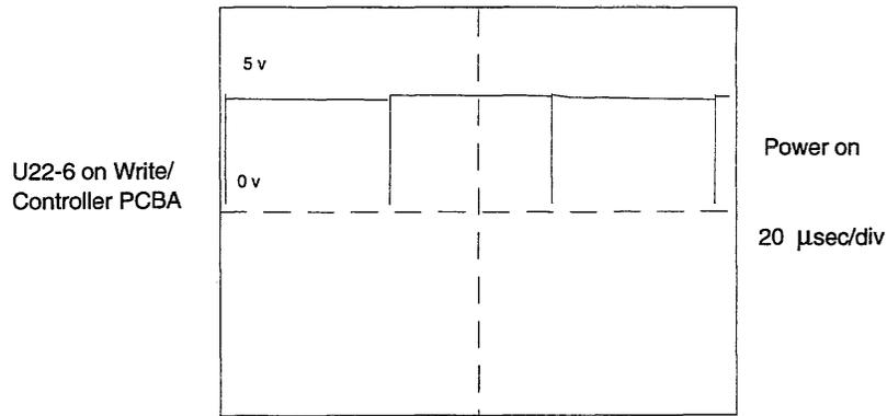
Figure 3-7 Ramp Reset Pulse
