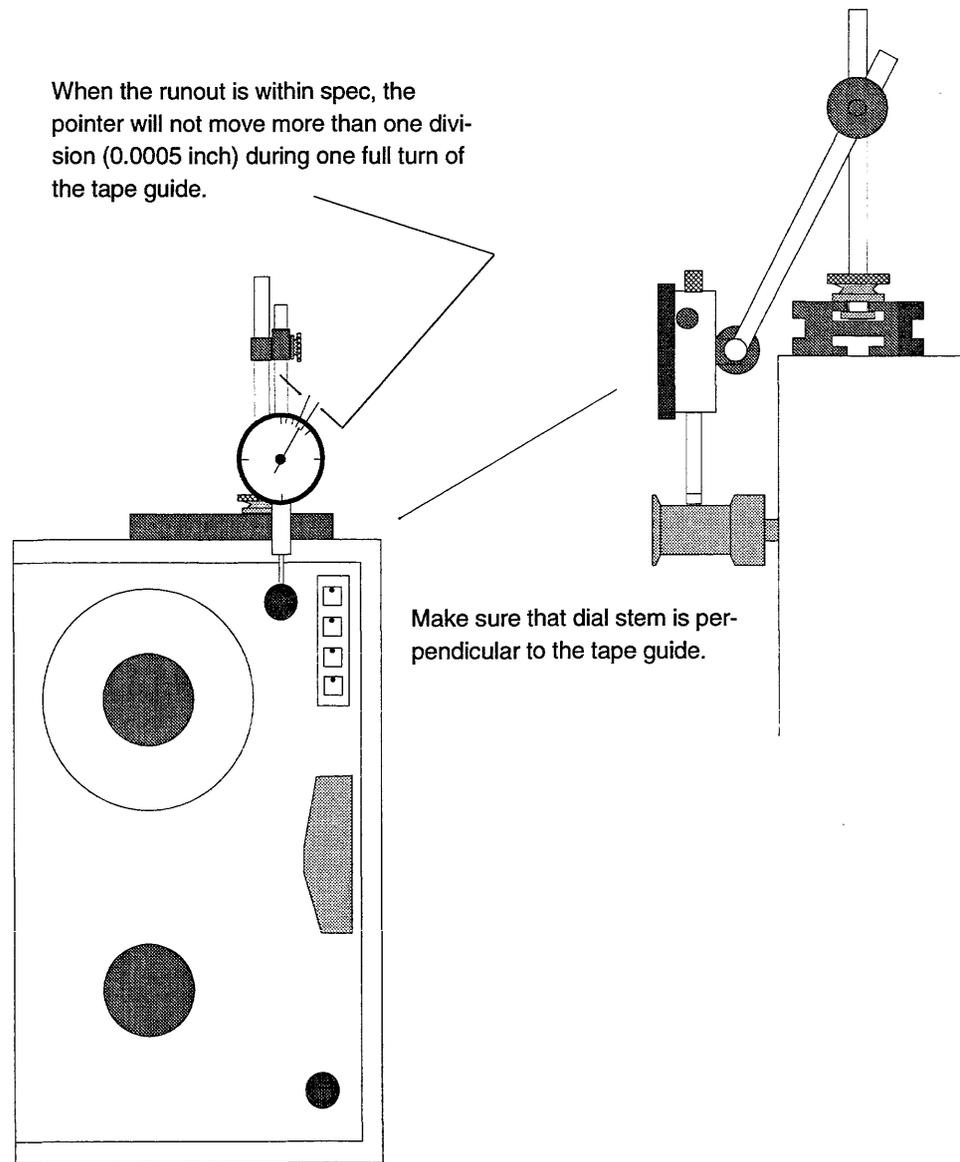
**Figure 8-5** Measuring Tachometer Tape Guide Runout
