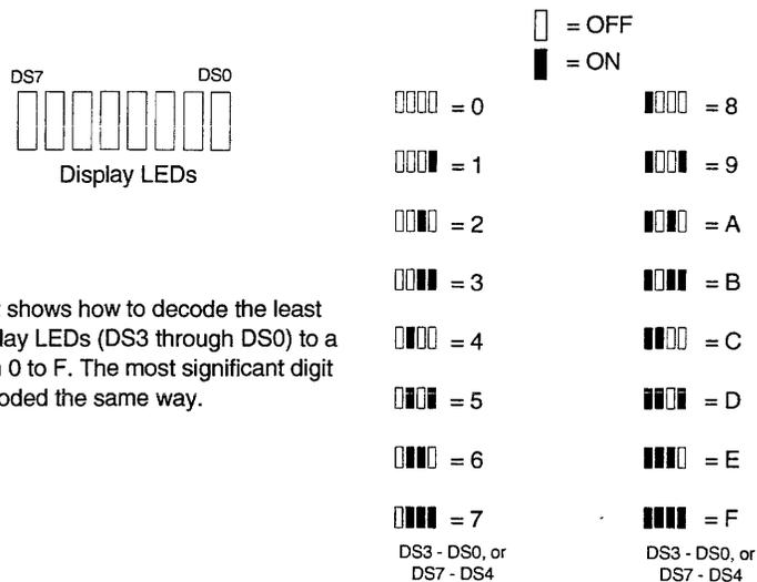
The illustration to the right shows how to decode the least significant digit of the display LEDs (DS3 through DS0) to a hexadecimal number from 0 to F. The most significant digit (DS7 through DS4) is decoded the same way.
