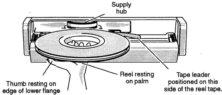
**Figure 3-5 Correct Way to Insert Reel**
