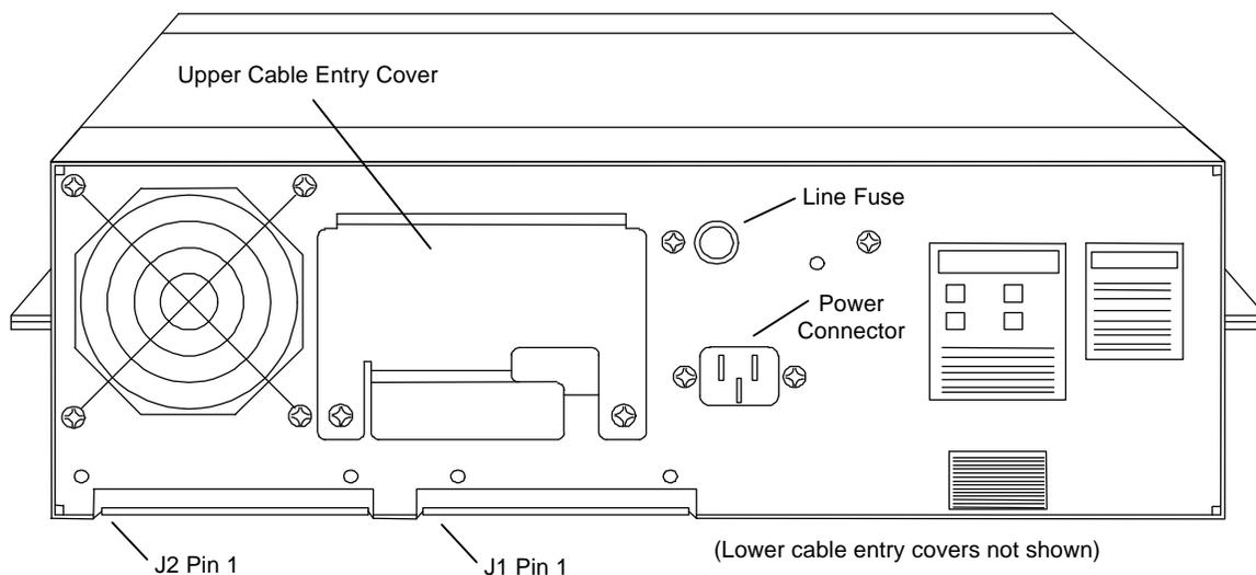
**Figure 1-10 Industry Standard Interface Connector Placement**
