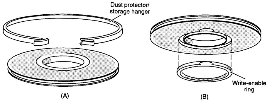
**Figure 3-3 Dust Protector and Write-enable Ring**
