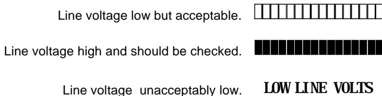
Figure 4-4 AC Line Voltage Display
