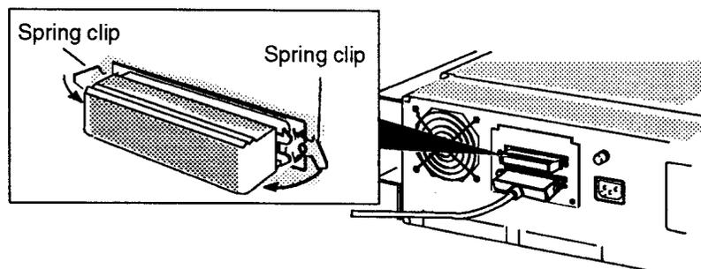
Figure 1-8 Connecting the SCSI Cable to the Tape Drive (SCSI Alternative 2 shown)
