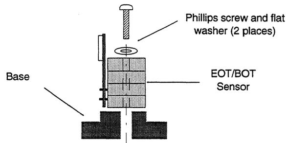
**Figure 9-8** EOT/BOT Sensor Assembly Mounting
