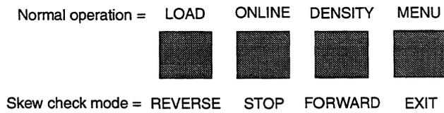
Figure 10-5 Front Panel Switches in the Skew Check Function
