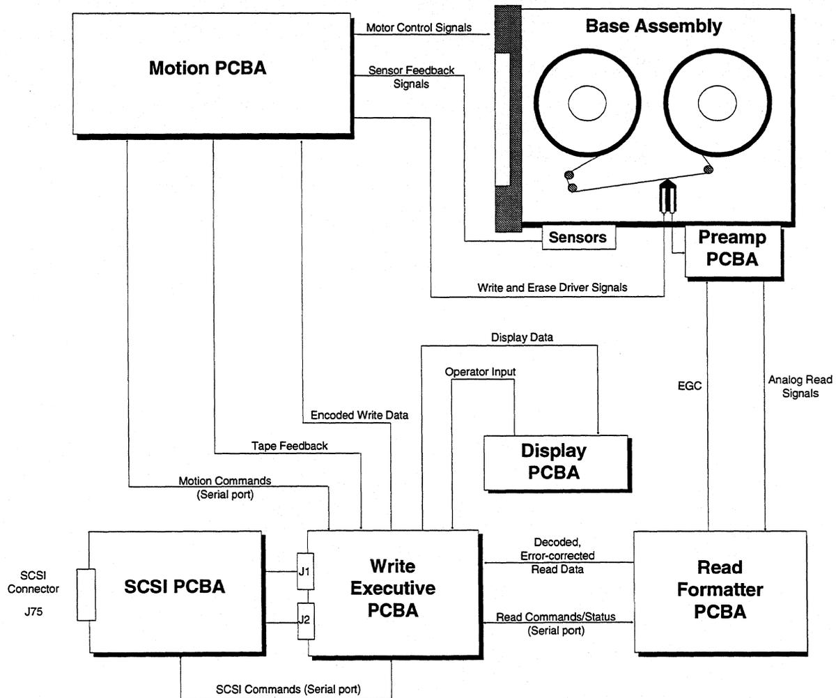
Figure 2-1 34XX Series General Block Diagram
