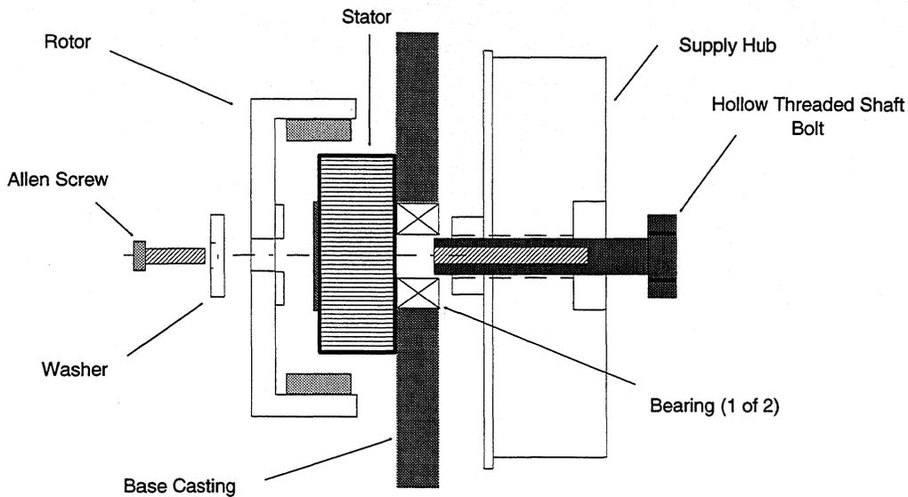
**Figure 9-9** Typical Motor Assembly
