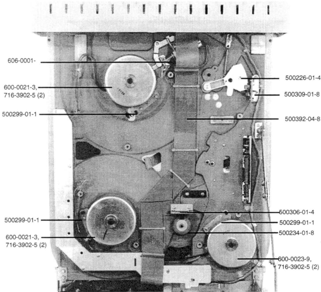
Figure 13-4 Underside of Base with Motion PCBA removed
