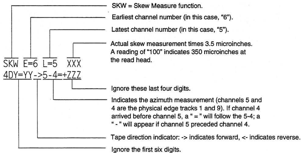
Figure 10-1 Skew Measure Front Panel Display
