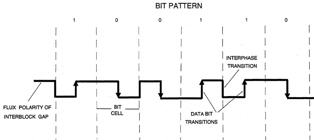
A "1" bit transition is in the direction of the erased tape polarity.
