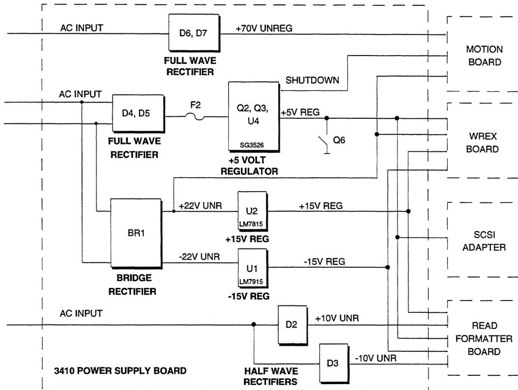
Figure 4-3 Power Supply Block Diagram
