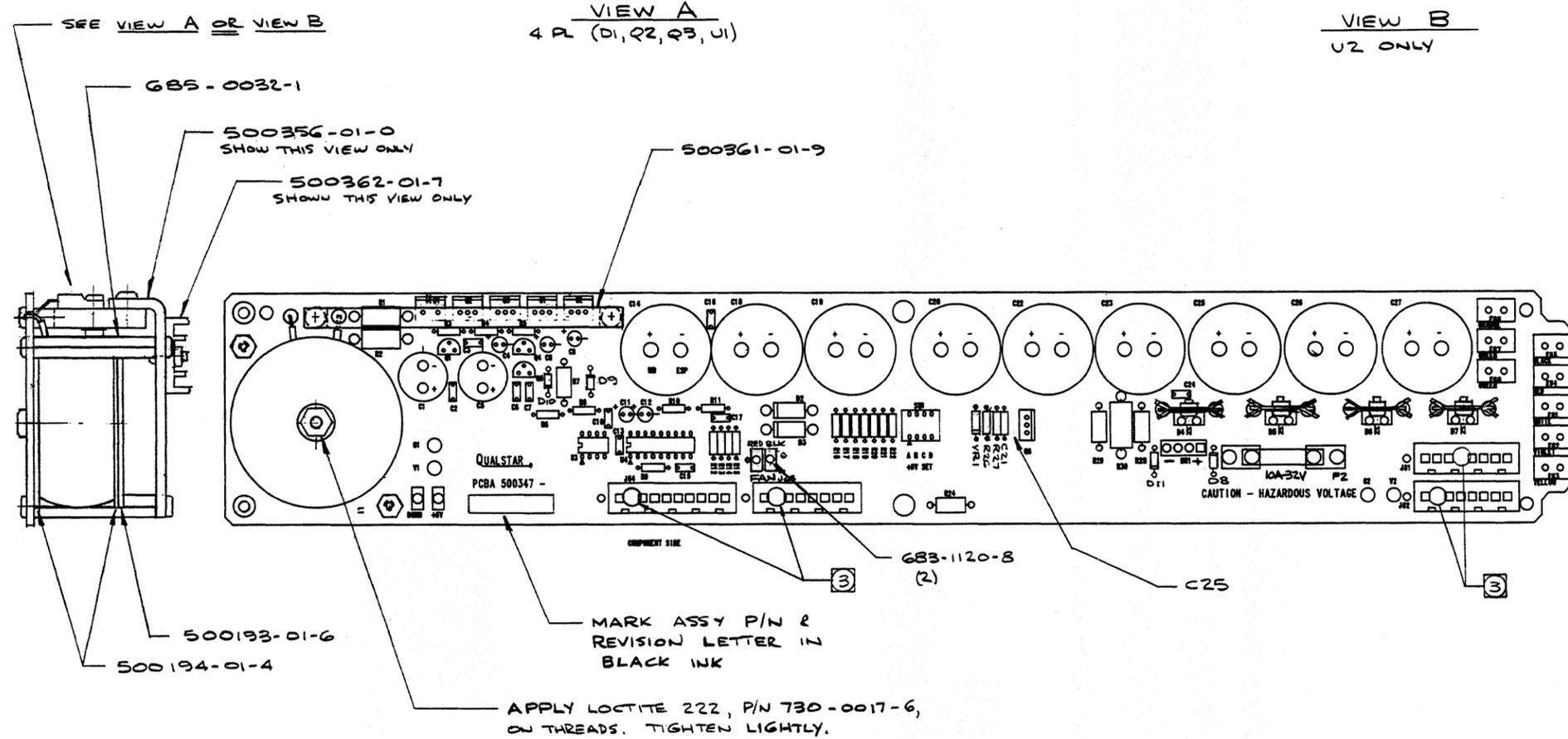
③ REMOVE INDICATED PINS BEFORE INSTALLING HEADERS.
