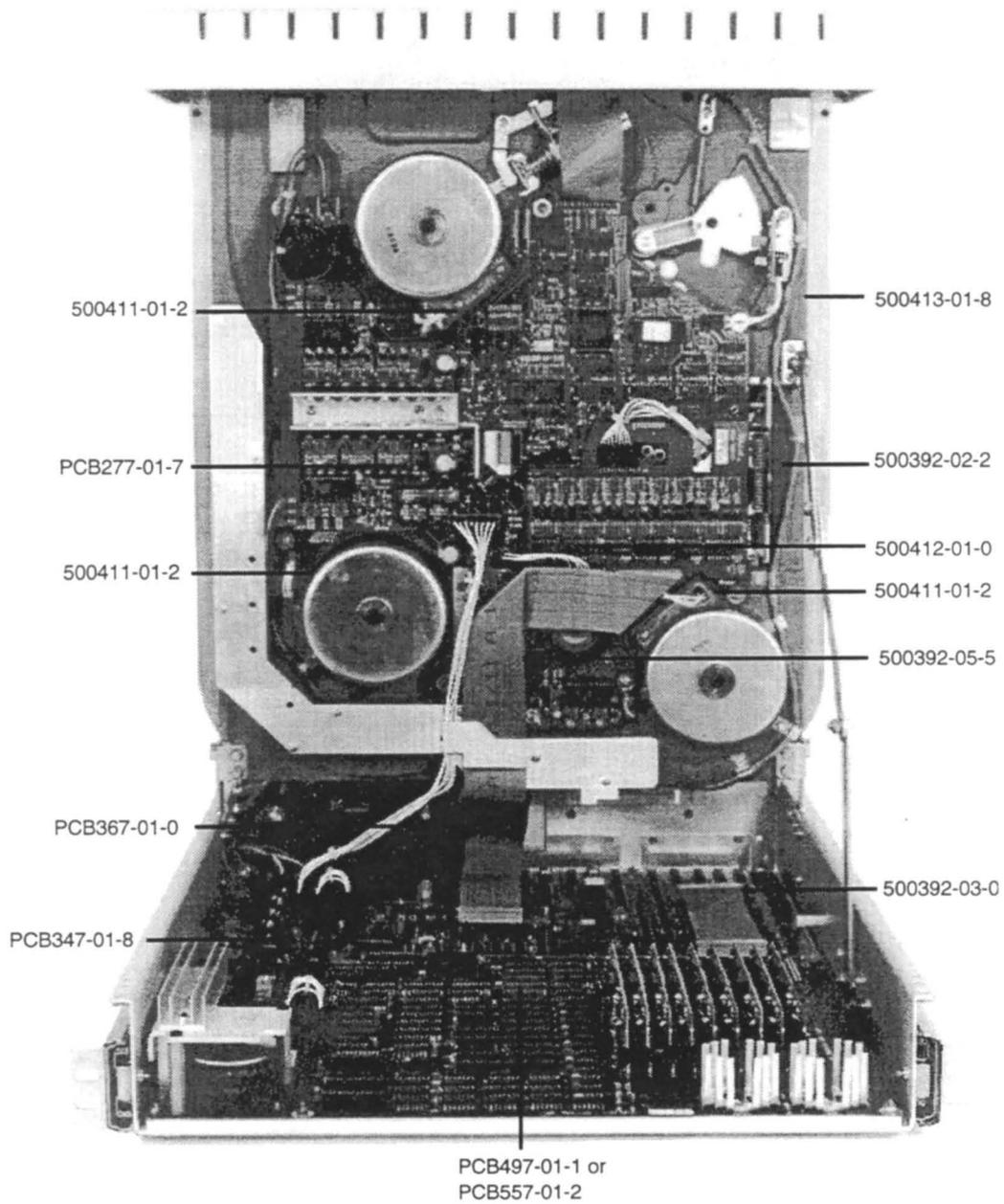
**Figure 13-3** 3410/3412 Internal Component Locations
