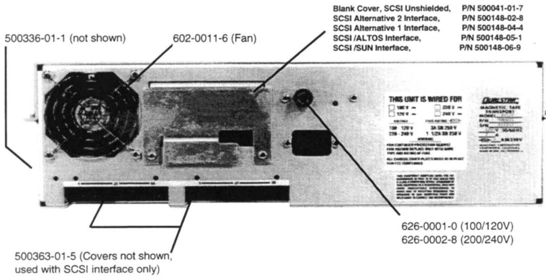
Figure 13-2 34XX Tape Drive, Rear View
