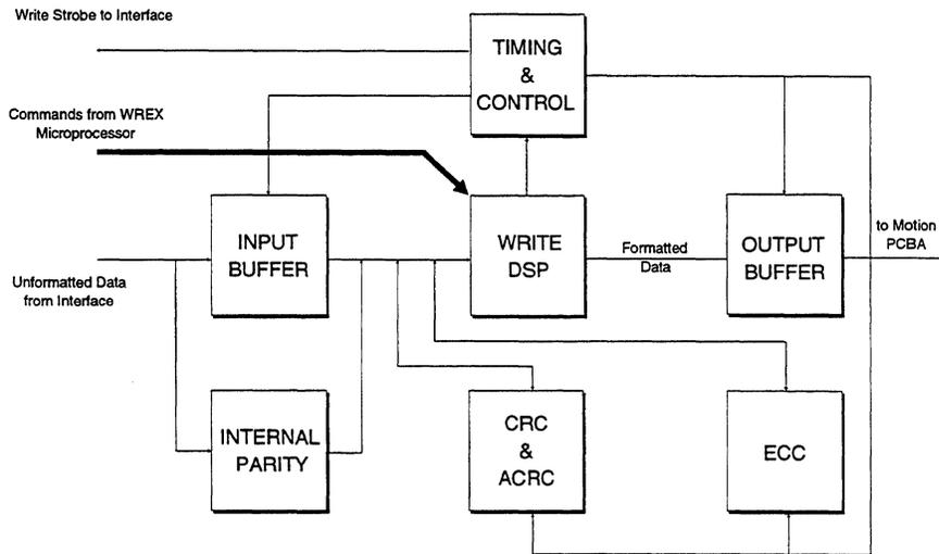
Figure 5-1 Write Formatter Block Diagram
