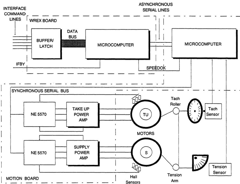
**Figure 4-2** Motor Control Block Diagram
