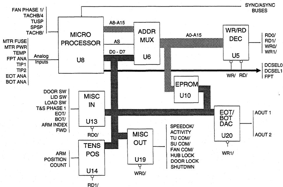
Figure 4-1 Motion Board Microcomputer Block Diagram
