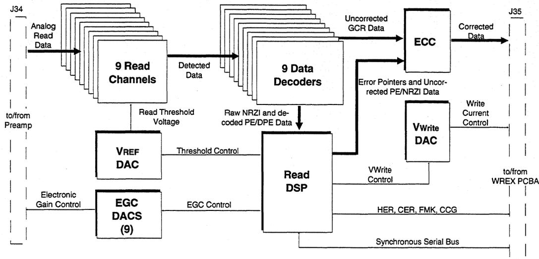
**Figure 6-3** 500557 Read Formatter Block Diagram
