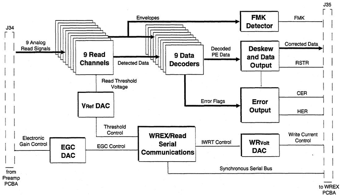
Figure 6-2 500497 Read Formatter Block Diagram
