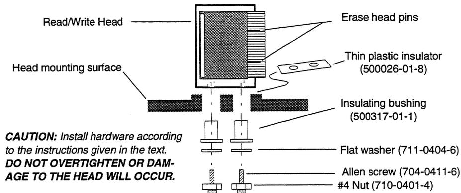
Figure 9-6 Head Installation Hardware
