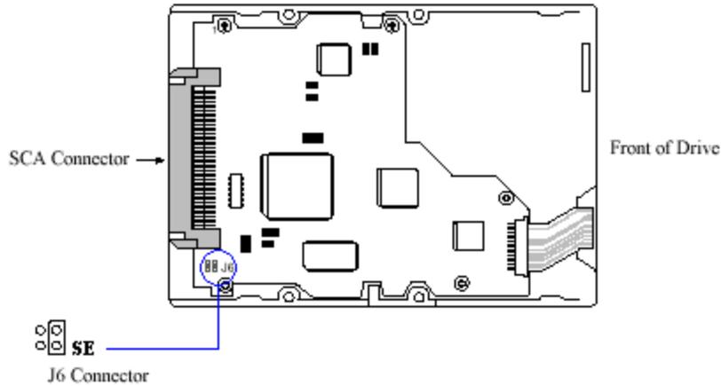
The Viking II SCA drive has only the single jumper position referenced above. Jumper position J6 determines if the drive is forced into SE mode only (jumper in) or if the drive supports multi-mode LVD (jumper out).
