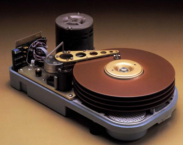
The Quantum Q2080™ is the latest addition to the Q2000 Series® of low-cost, 8" fixed disk drives, and is fully compatible with Quantum's 10-, 20-, 30- and 40-megabyte Q2000 products. It also allows a low-cost, high-capacity upgrade to low-capacity 8" fixed or floppy drives.
