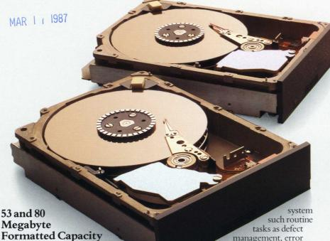
Megabyte **Formatted Capacity Drives with Integrated SCSI Controllers**
