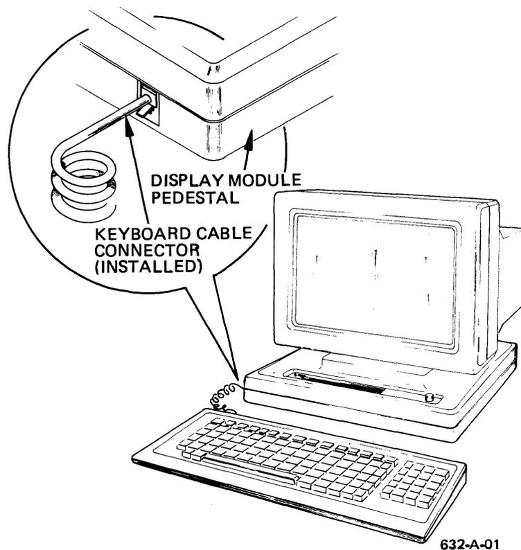
Figure 2-3. Keyboard Cable Connection to the Display Module
