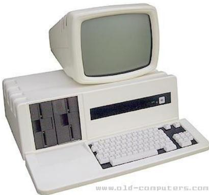
It's a PC based on Zilog Z80A, with 64k RAM, two 256Kb or 600 Kb 5"1/4 floppy disks, 14" monitor monochrome 80x24 text resolution.
