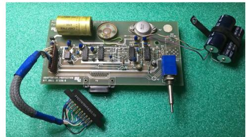
During the operations I also saw that on the analog board there is a resistance flaked and therefore is probably broken, but the problem is that the schematics are not available anywhere and for that reason the value of the resistance was unknown to me.
