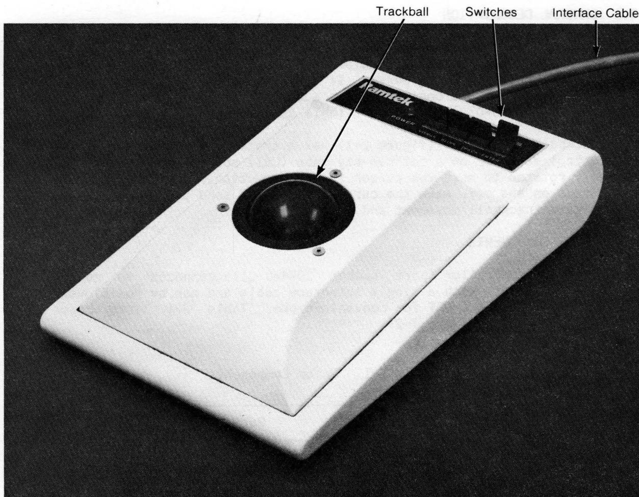
Figure 2-1. Trackball Controller
