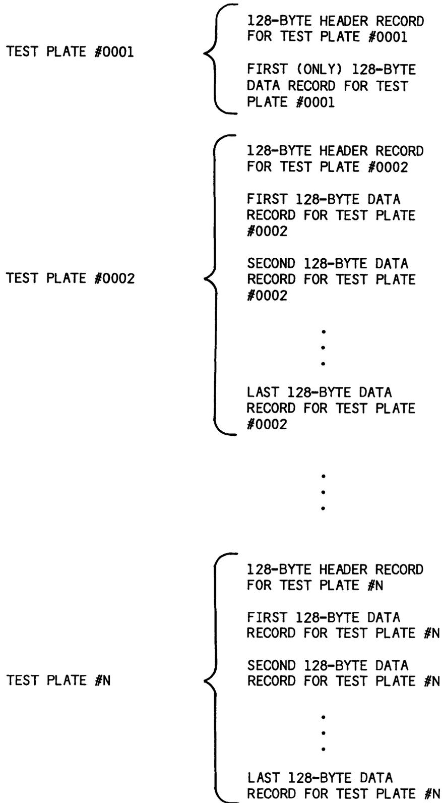
Figure C-1. Acceptance Tests Magnetic Tape Format
