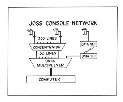
may be plugged into any one of more than 300 lines, which are connected to a centrally located line concentrator. This line concentrator, in turn, extends the connection over one of 32 lines to a data multiplexer, which intermixes all communications to the computer.
