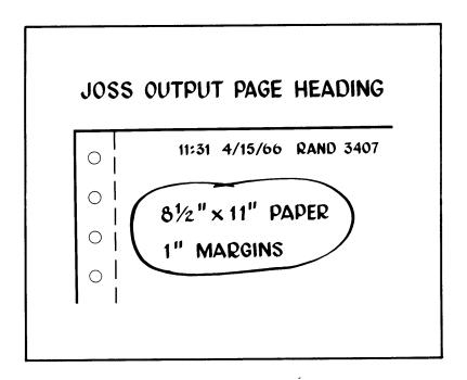
The output paper is pin fed, but when the tear strips are removed, each sheet, with a heading line as shown above, is reduced to the standard size of  $8\frac{1}{2}$  by 11 in. In addition, JOSS feeds enough lines to leave a 1-in. margin at the top of each page, and will also give us a 1-in. margin at the left and 1 in. at the bottom of each page.
