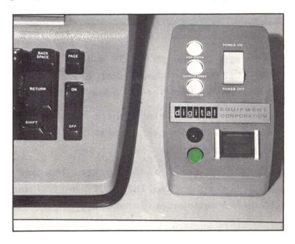
We therefore speak of the console being either in the RED state (computer control) or, as shown above, in the GREEN state (user has control and may type).
