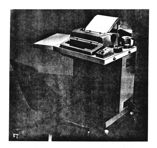
The photograph above shows the JOSS console, which consists of a modified IBM Selectric typewriter and a control box. At first, you will operate the typewriter separately, and then will use the control box to connect the console to the computer. At that point you will begin to "converse" with JOSS.
