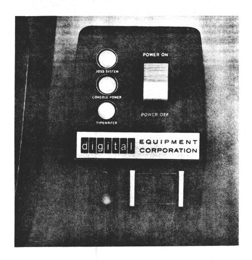
Press the white rocker switch on the control box toward POWER ON.
