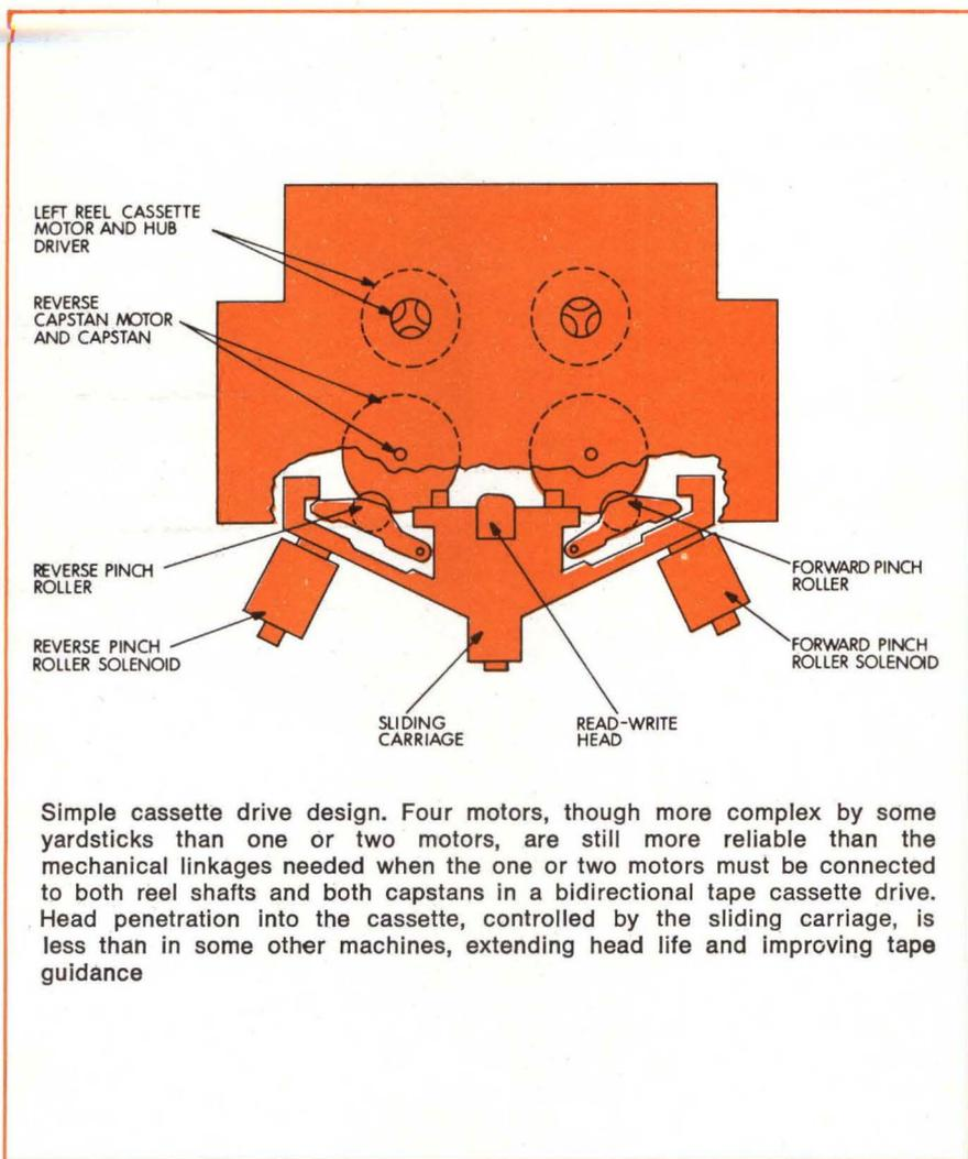
Simple cassette drive design. Four motors, though more complex by some yardsticks than one or two motors, are still more reliable than the mechanical linkages needed when the one or two motors must be connected to both reel shafts and both capstans in a bidirectional tape cassette drive. Head penetration into the cassette, controlled by the sliding carriage, is less than in some other machines, extending head life and improving tape guidance
