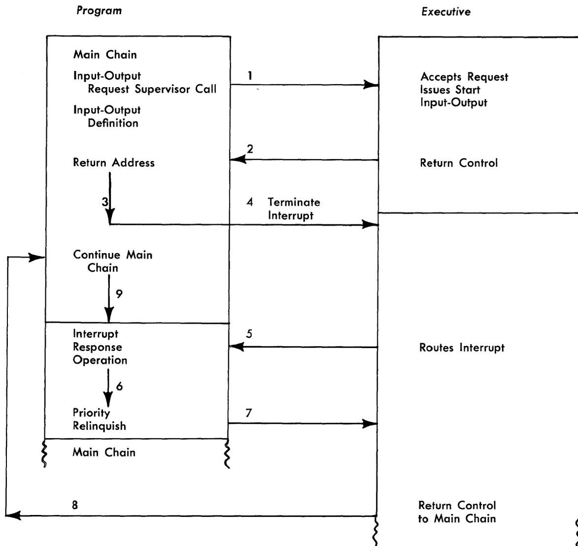
Figure 12. Control Flow During an Input-Output Operation
