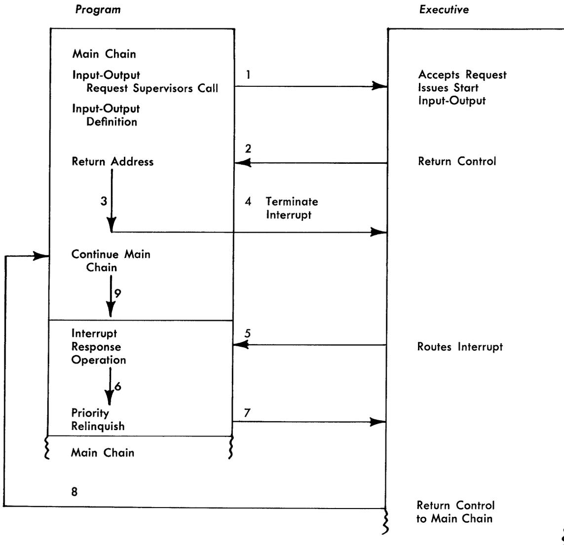
Figure 13. Control Flow During an Input-Output Operation
