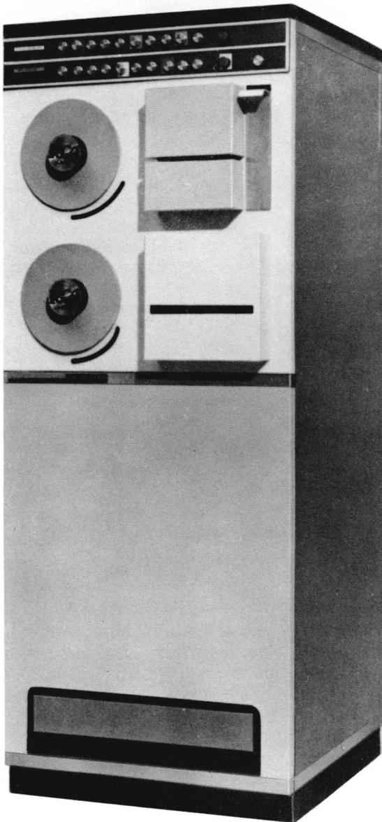
*Figure 6. Model 70/221 Paper Tape Reader/Punch*
