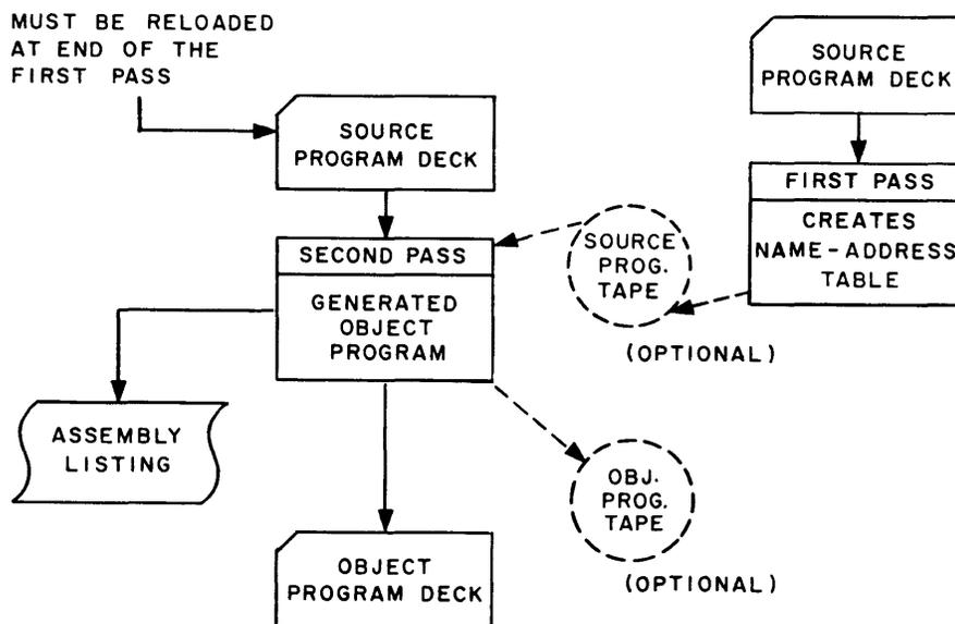
Figure 1. Assembler Operation
