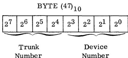
3. Stores the Standard Device Byte for the Interrupting device in the reserved HSM location forty-six  $(2E)_{16}$ .
