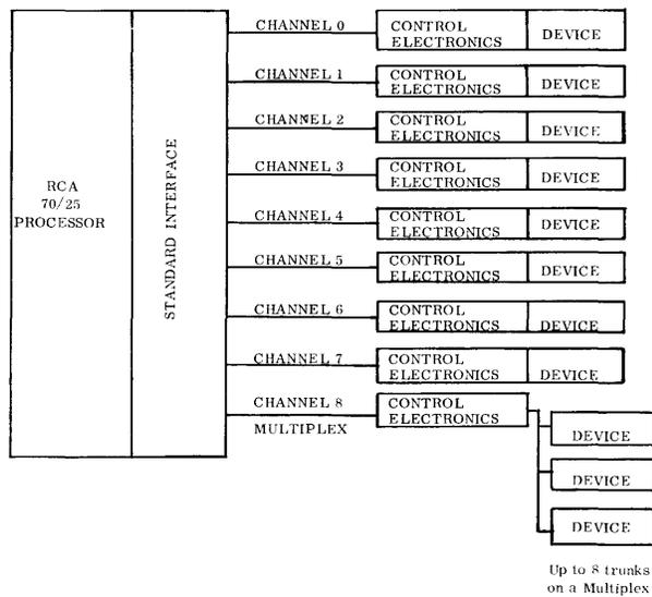
Two of the eight channels may be used for high-speed transmission, and the remaining six for medium speed, or all eight may be used for the medium speed. The high-speed channels must be the first two (0 and 1) channels.
