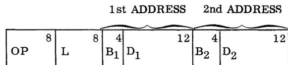
An address is divided into two parts: (1) a displacement of 12 bits contained in the instruction, and (2) a base address which is pre-stored in one of the fifteen General Registers.
