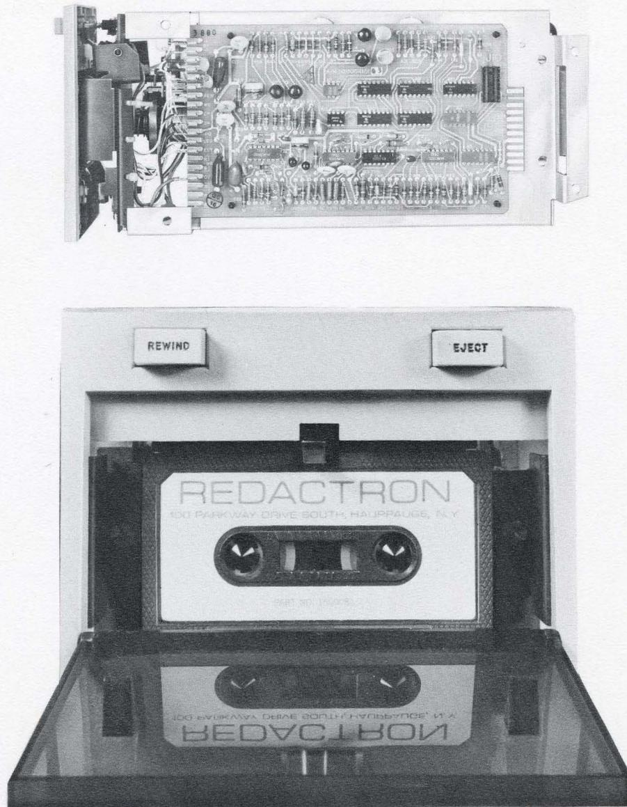
Figure 1 – Model 100 Magnetic Tape Cassette Transport
