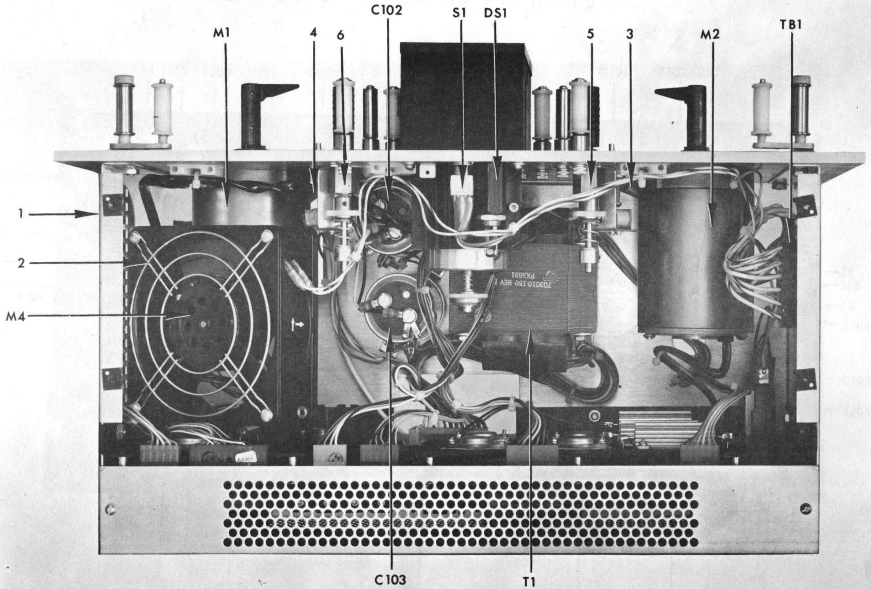
Figure 7-4. Rear View of Front Panel, RRS6500BEX/660/ARB. The location of components on the RRS6500BEX/660/DRB is approximately the same.
