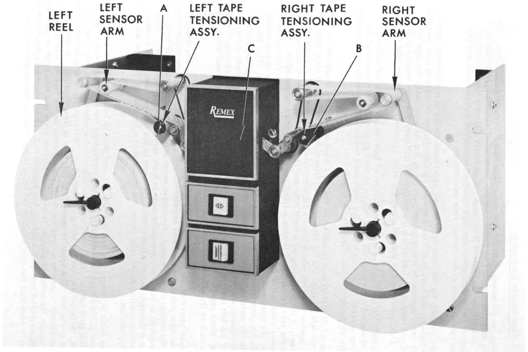
Figure 4-6. Front View Showing Various Points of Tape Tension.
