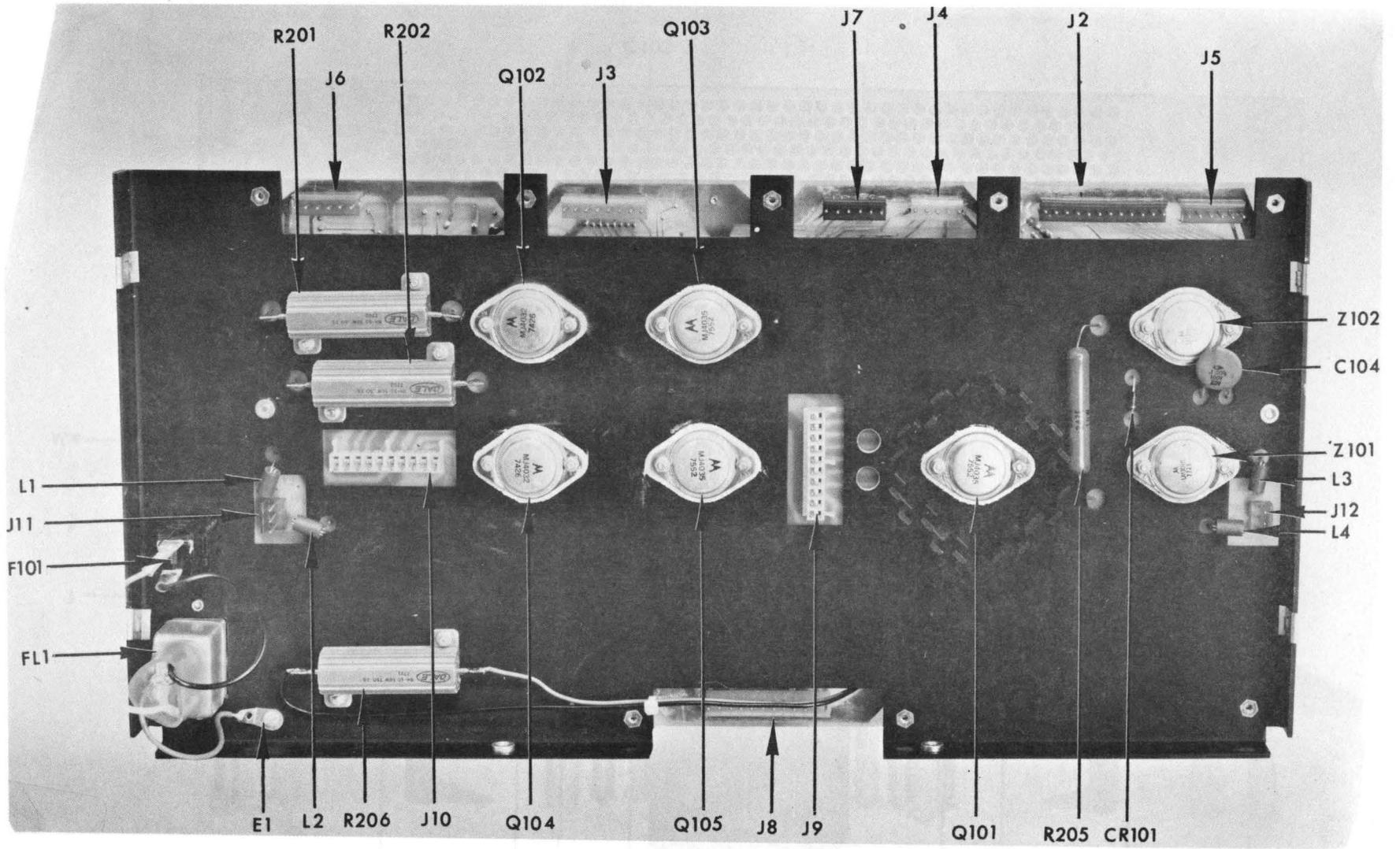
Figure 7-5. Power Driver Panel Assembly 111021-3.
