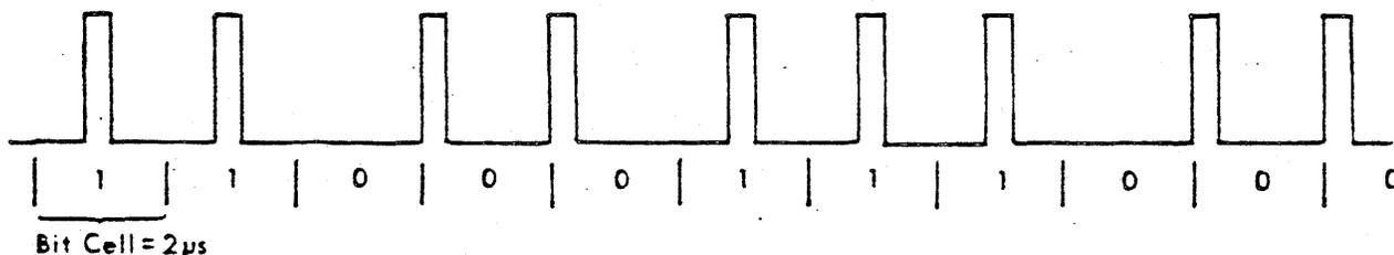
Figure 2-5. MFM Encoding.
