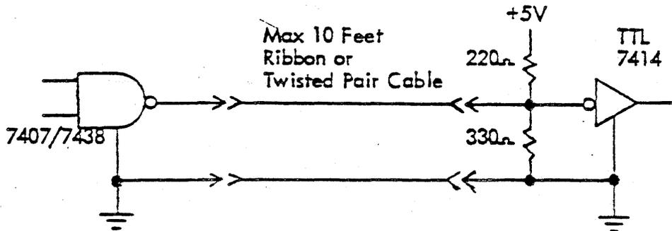
Figure 2-3. Recommended Interface Circuits.
