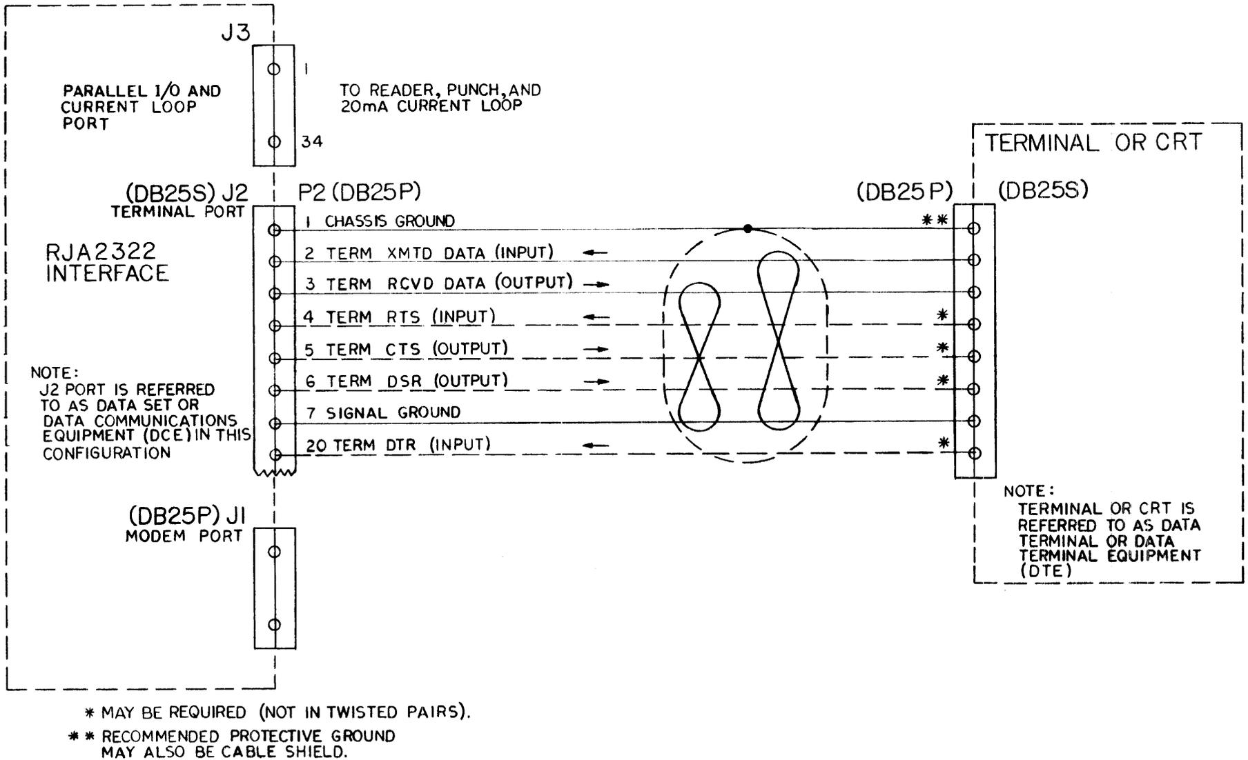
Figure 3-2. Terminal or CRT to Reader and Punch RS - 232 - C Connections.
