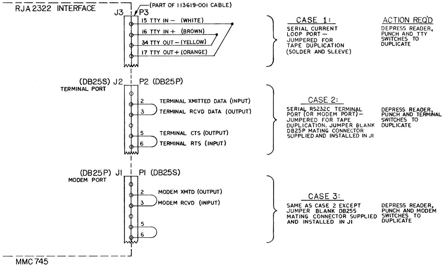
Figure 3-5. Spare Port Jumpering For Tape Duplication.
