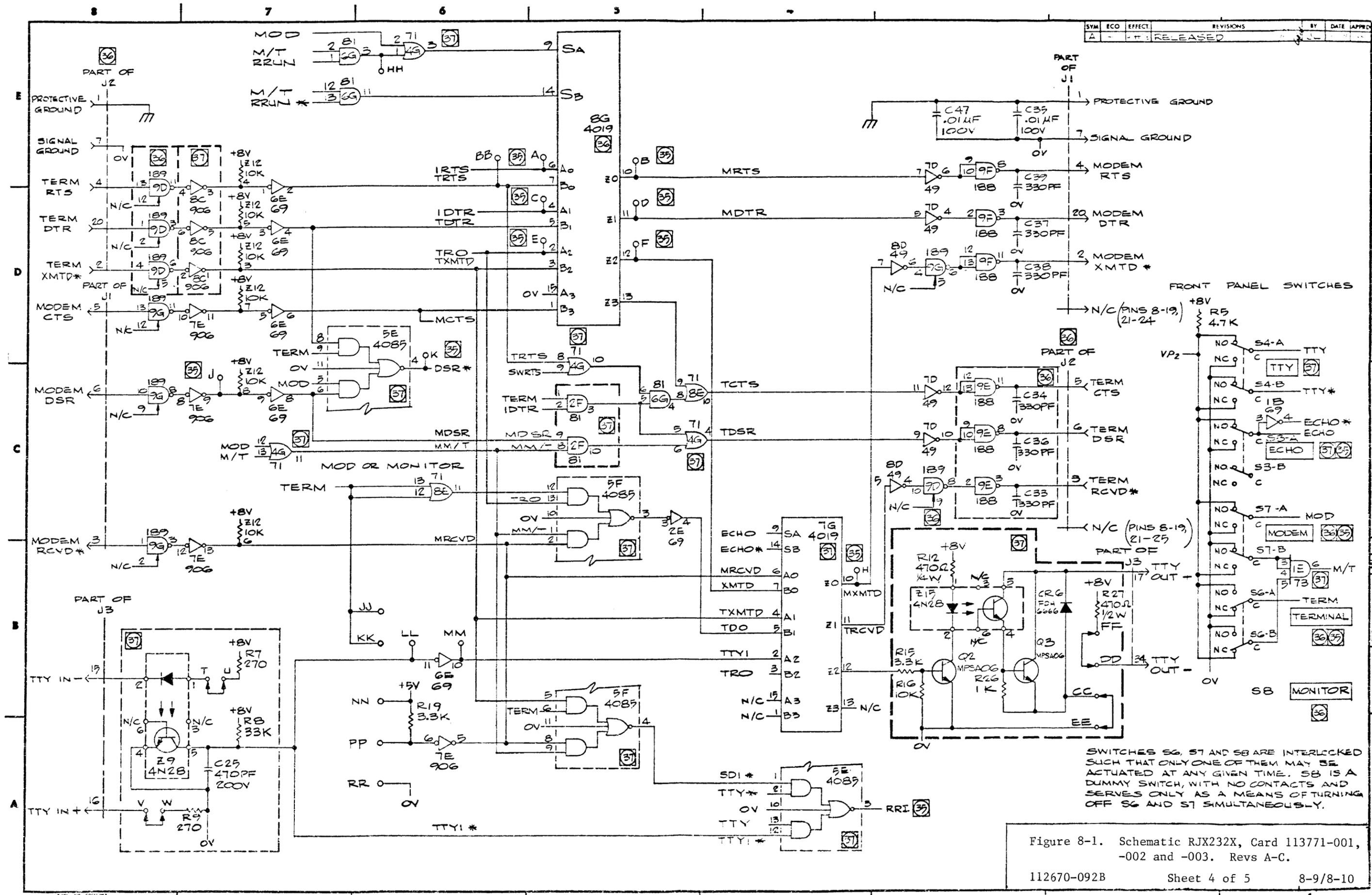
SWITCHES S6, S7 AND S8 ARE INTERLOCKED SUCH THAT ONLY ONE OF THEM MAY BE ACTUATED AT ANY GIVEN TIME. S8 IS A DUMMY SWITCH, WITH NO CONTACTS AND SERVES ONLY AS A MEANS OF TURNING OFF S6 AND S7 SIMULTANEOUSLY.
