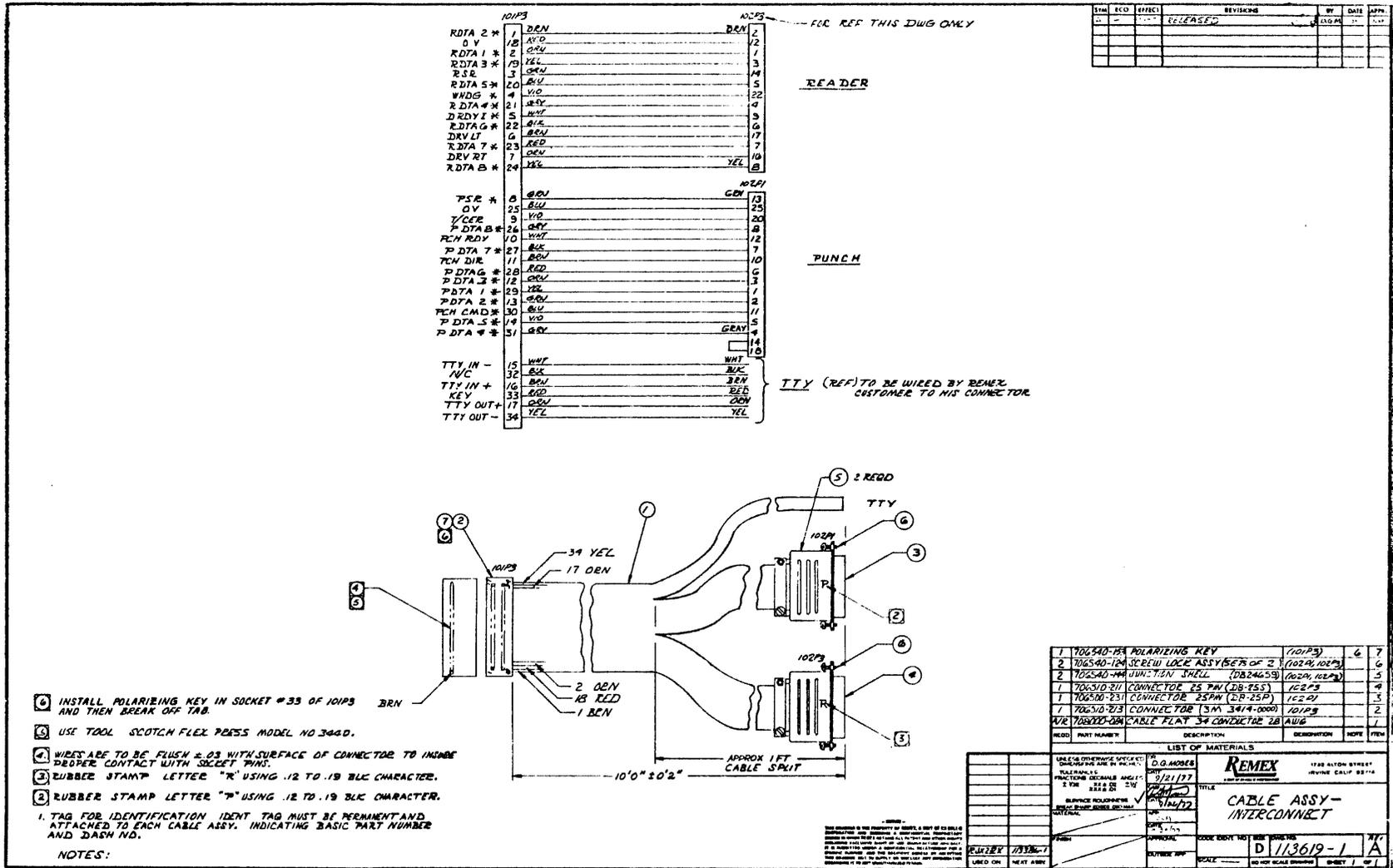
Figure 2-2. Interconnect Cable Assembly, 113619-001.
