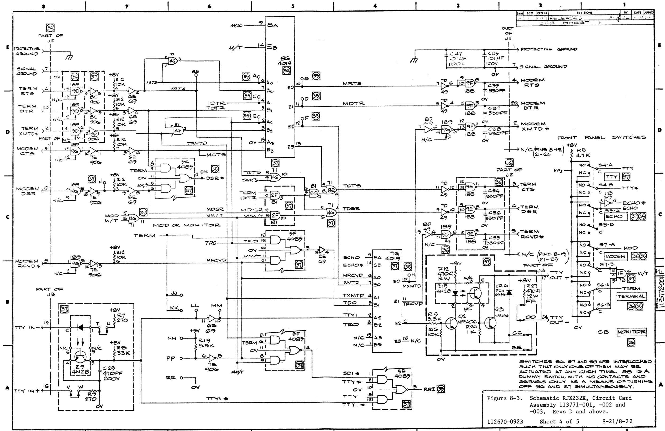
Figure 8-3. Schematic RJX232X, Circuit Card Assembly 113771-001, -002 and -003. Revs D and above.
