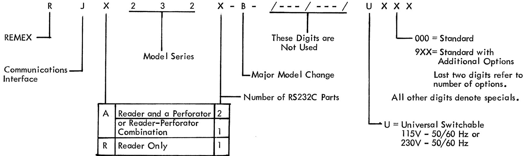
Figure 1-5. REMEX Model Number Coding.
