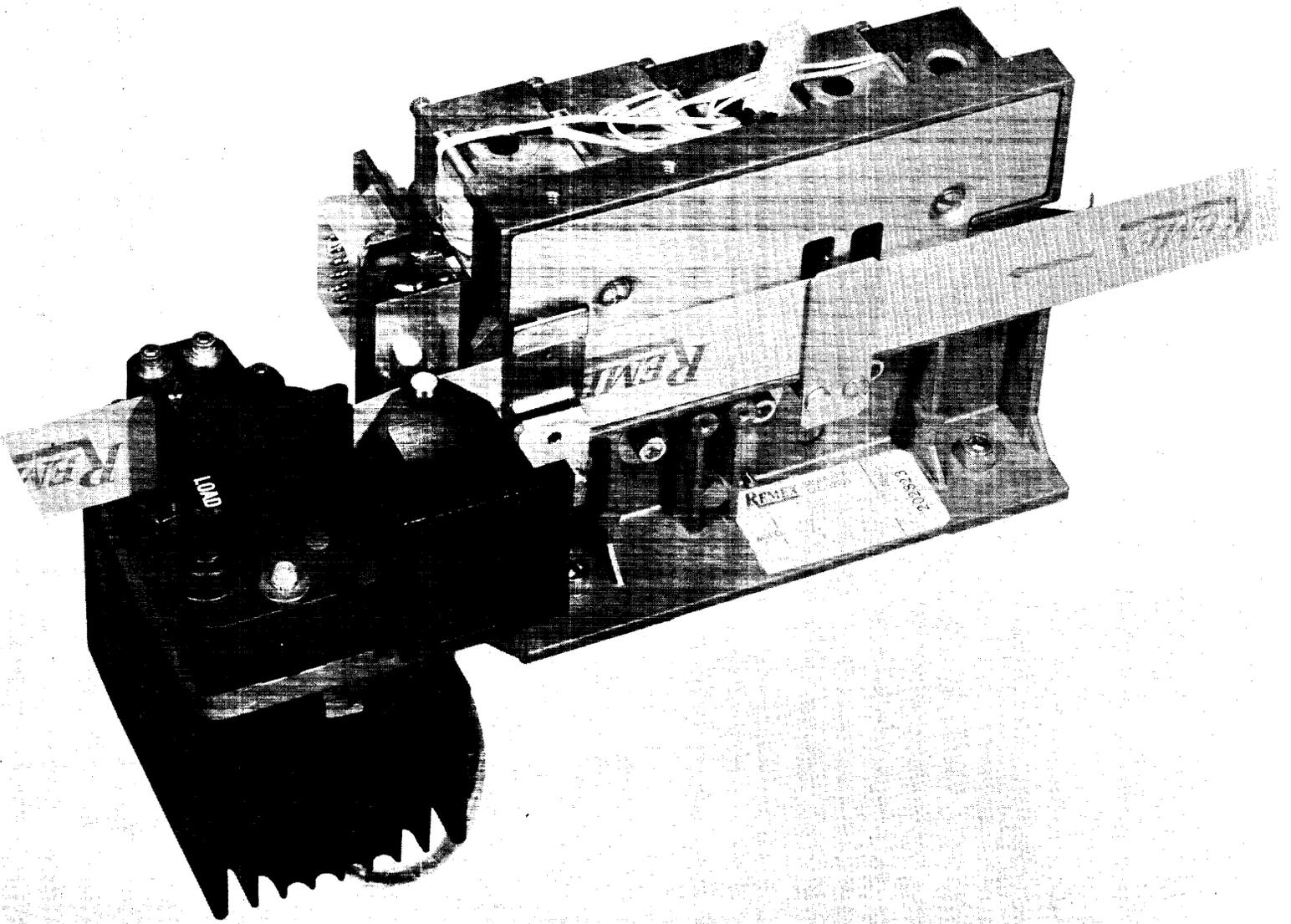
Figure 3-2. Tape Threaded Through The Punch Mechanism.
