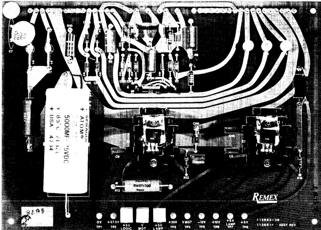
Figure 7-14. Reader Card Assembly 110801-003 (Top) and Power Supply Card Assembly 113681-001 (Bottom).
