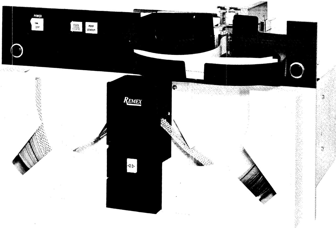
Figure 1-3. REMEX Punched Tape Reader/Perforator System, Model RAF6125BB.
