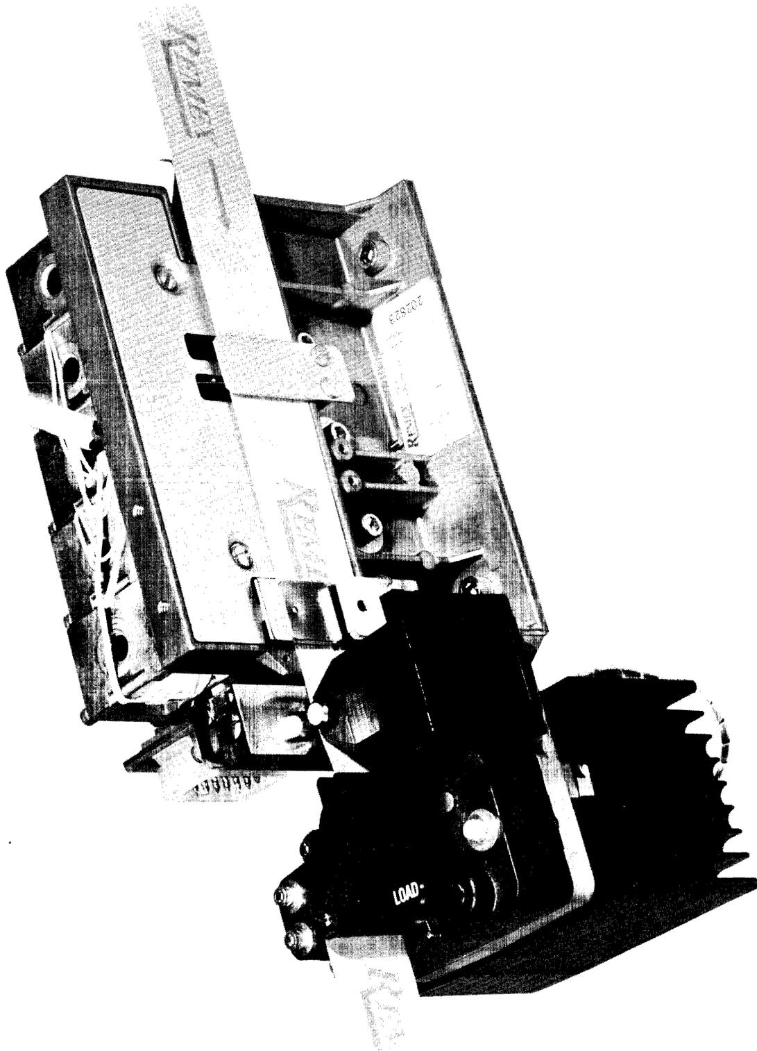
Figure 3-3. Tape Threading Through the Punch Mechanism.
