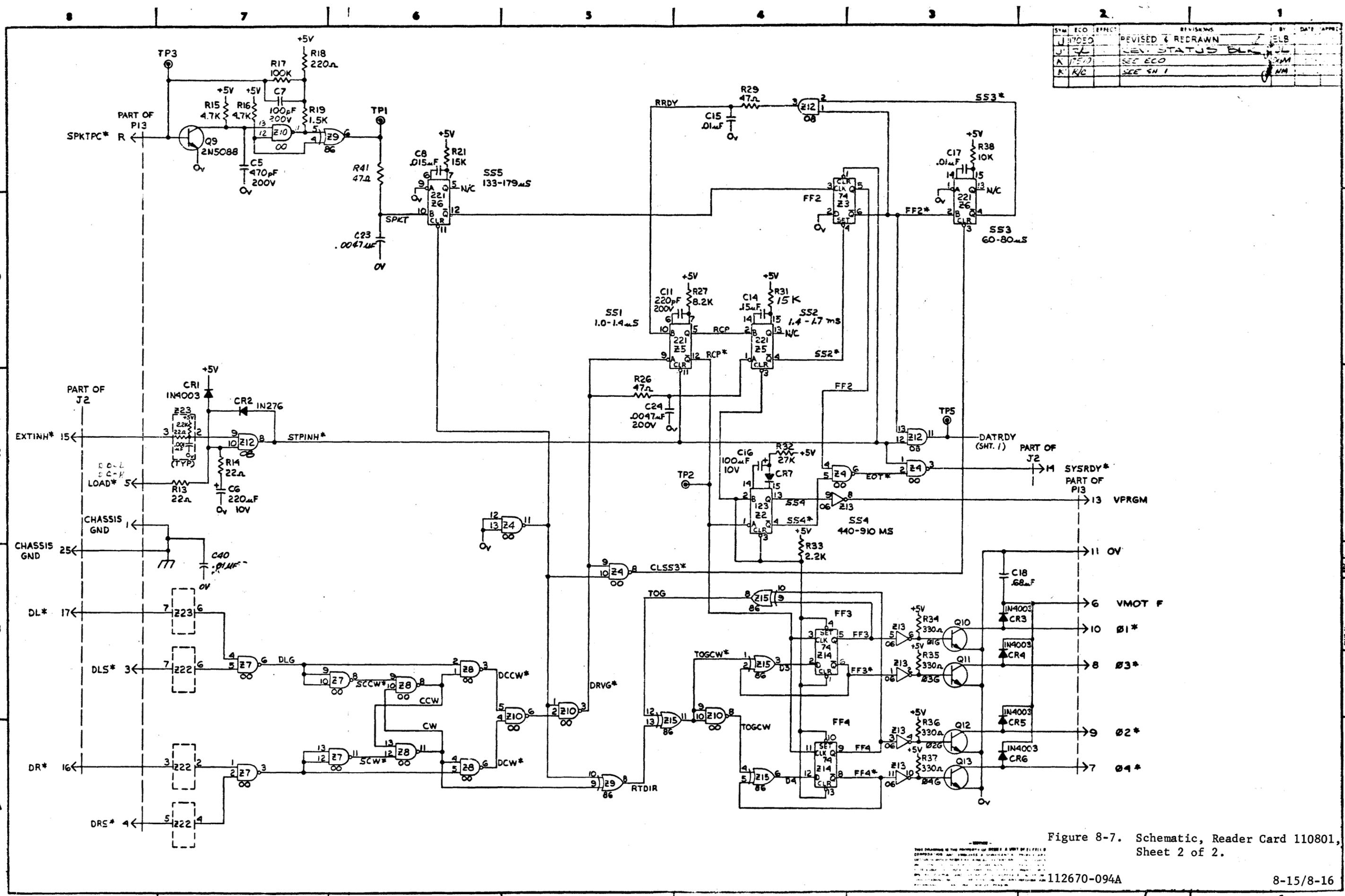
Figure 8-7. Schematic, Reader Card 110801, Sheet 2 of 2.
