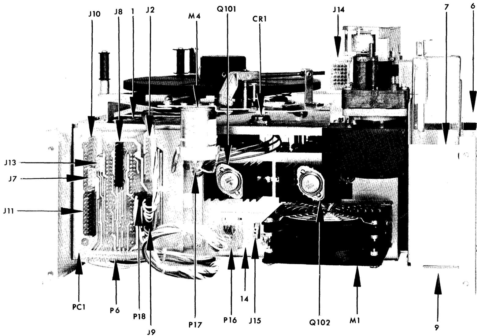
Figure 7-6. Chassis Assembly 113688-001, Inside View.
