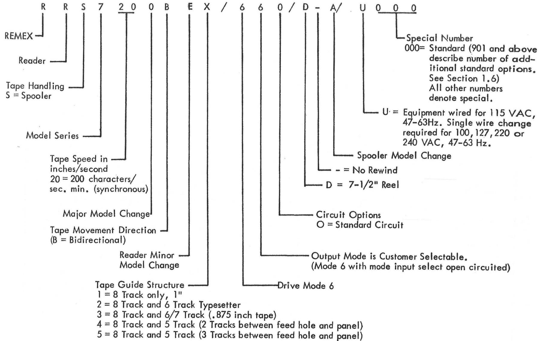
Figure 1-3. Model Number Coding For RRS7200.
