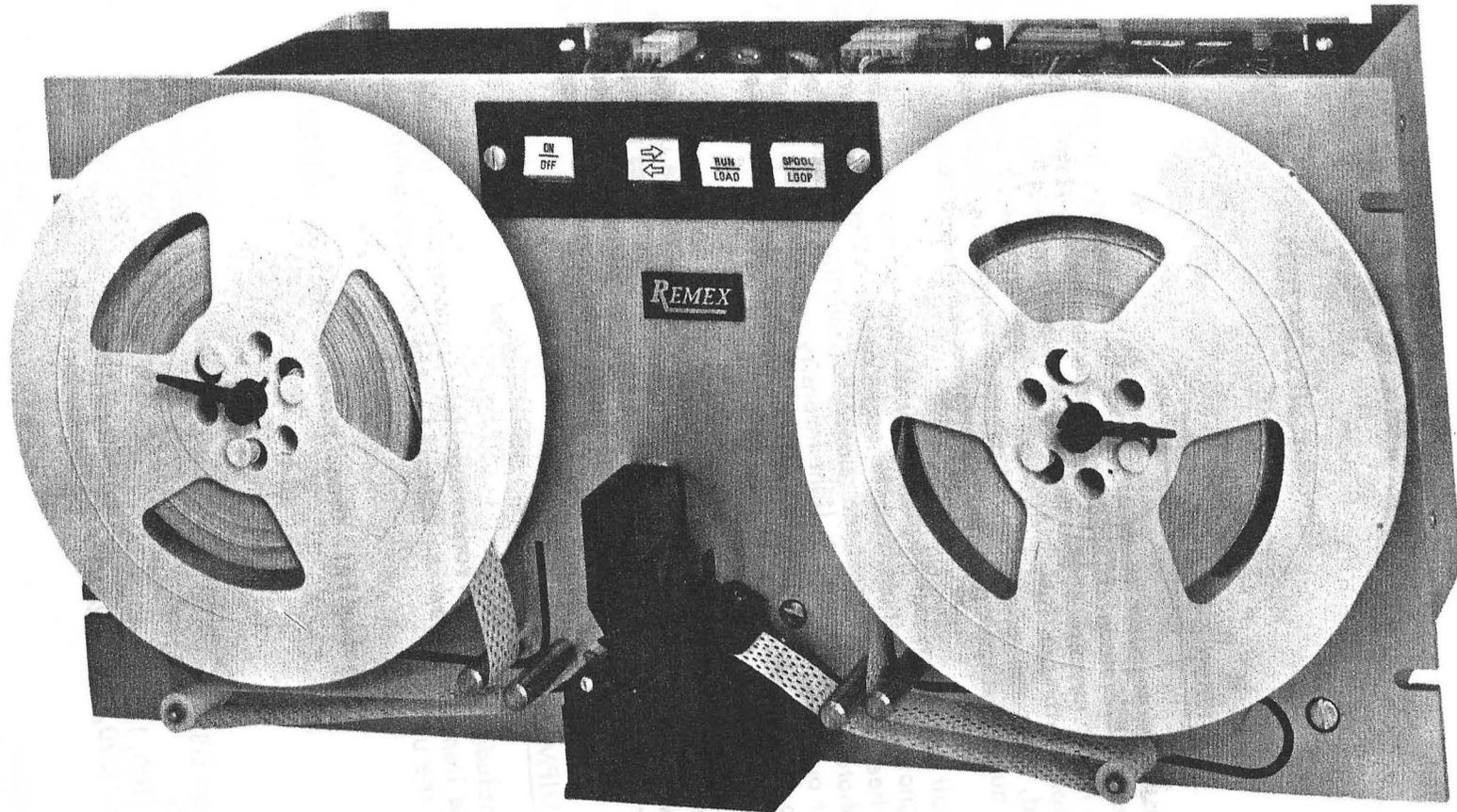
Figure 1-1. REMEX Reader Spooler, Model RRS7200BEX.
