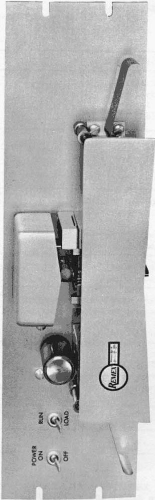
Figure 1-1A. The REMEX Tape Reader, Model RR-1002LB.
