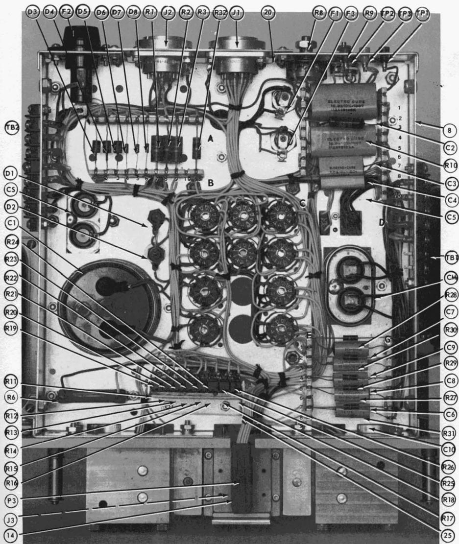
Figure 7-11. Component layout of the electronic chassis.
