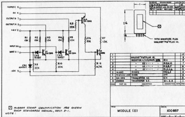
Figure 7-8. Input Control Module (X2), Schematic and Assembly, Modes 2 and 4.
