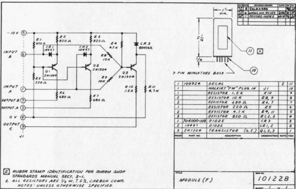
Figure 7-10. Input Control Module (X2), Schematic and Assembly, Modes 1 and 3.
