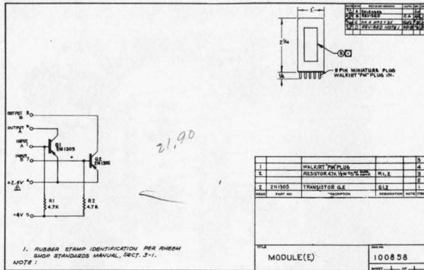
Figure 7-9. Drive and Brake Amplifier Module (X7, X8), Schematic and Assembly, All Models.
