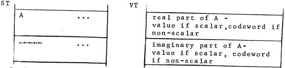
Genie constructs two argument words on the B6-list for each complex argument A. The first addresses the real part of A; the second addresses the imaginary part of A.
