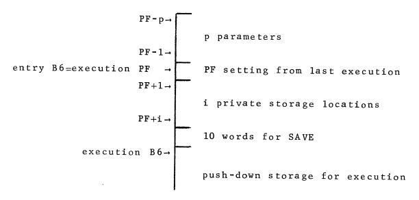
The END code sequence restores all fast registers, restores the PF setting for the last execution at END+1, backs B6 up by p+i+1 to free all B6-list list used in execution, fetches (T7) for implicit execution, and exits to the PF setting on entry. The specific code sequences are as follows:
