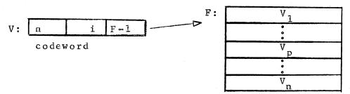
In programming, the data element V is addressed by the code p  $\rightarrow$  index register i
