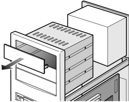
2. Insert the drive unit into the bay. Do not apply excessive pressure to the cables inside the computer.
